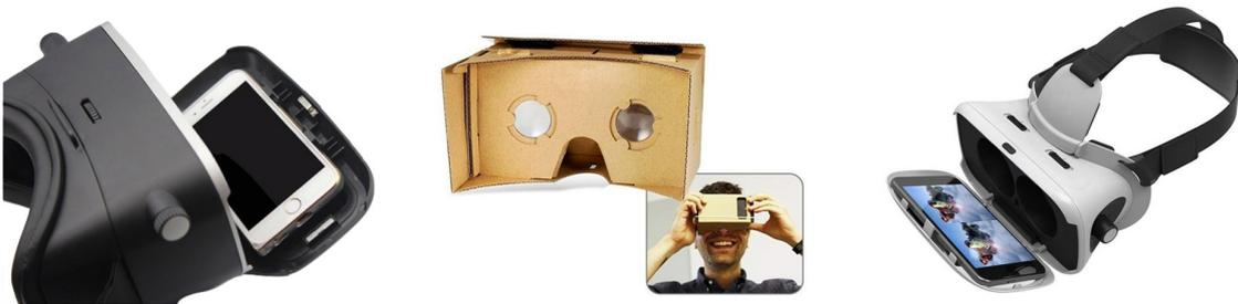
Figure 3: A variety of mobile VR headsets are available to the average consumer at a low price tag. Most mobile VR headsets are equipped with head straps and adjustable lens position for increased comfort. However, user interaction with the Virtual Environment (VE) remains problematic, as it is mostly accomplished through tedious head movements.
