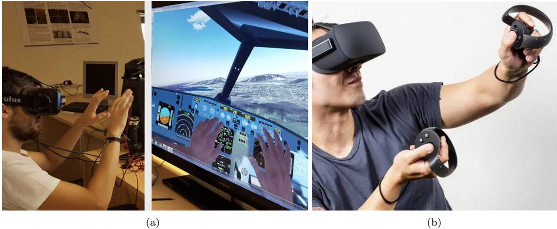
Figure 2: Examples of two common interaction modalities in VR. (a) Interacting with a virtual aircraft cockpit in real-time, using LeapMotion’s hand-tracking controller, mounted onto an Oculus Rift VR HMD. (b) Fighting with a virtual enemy, using handheld wireless controllers.
