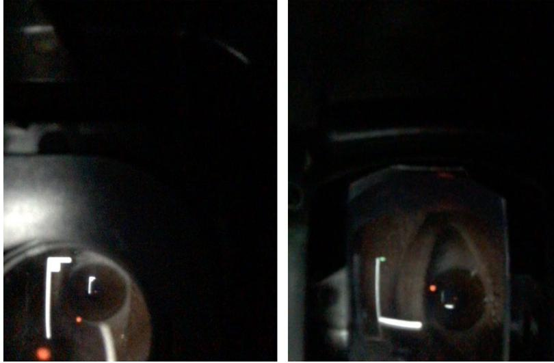
Figure 18: Raw front-facing camera frames, from two different mobile VR headsets. Our study shows that eye-tracking is possible with any mobile VR headset, as long as the iris remains visible to the front-facing camera at all times. In this case, we observe that the plastic frame of the HMD on the left partially obstructs the eye region, while the HMD on the right allows the front-facing camera a clearer view.
