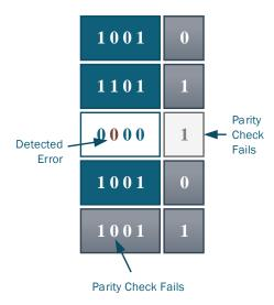
Figure 2.3: Parity:In this table parity bits are inserted for each row and each column. Bits in green boxes represent data bits and bits in gray boxes represent parity bits. The parity bit is '0' for even number of '0' and odd otherwise. In the third row and second column an example of error detection is presented where both parity checks fail.
