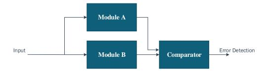
Figure 2.2: Dual Modular Redundancy: By passing the input through two different modules that perform the same operation on the input and comparing the results the system is able to detect when an error occurred but is not able to decide which of the two outputs is the correct one.
