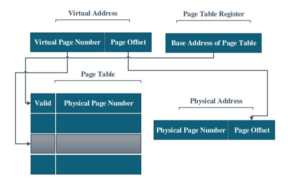
Figure 5.5: Virtual Memory Architecture: When a virtual address arives, the page table is used to map the virtual address to a physical address.
