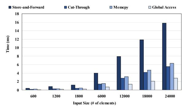
Figure 5.7: Worker Timings: Worker timings are presented here for different workload input sizes. The workload input size ranges from 600 to 24000 elements. Each bar represents a different memory transfer method, with the store-and-forward and cut-through being the reliable ones, and the memcpy and global access the unreliable ones.
