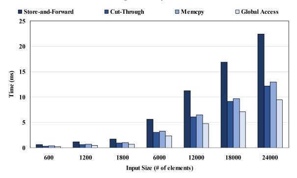
Figure 5.8: Total Timings: Total timings are presented here for different workload input sizes. The master timings is only dependant to the workload input size, hence the total timings are similar to the worker ones. The workload input size ranges from 600 to 24000 elements. Each bar represents a different memory transfer method; the store-and-forward and cut-through are the reliable ones, and the memcpy and global access the unreliable ones.
