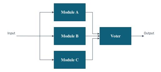
Figure 2.1: Triple Modular Redundancy: By passing the input through three different modules that perform the same operation on the input and by passing the outputs to a voter; the system is able to detect the correct output by choosing the most frequent output.
