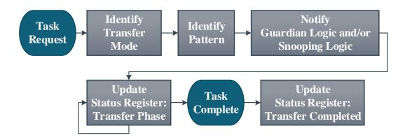
Figure 5.6: Task Request Handler Flowchart: The steps of the control logic behind the Task Request Handler is defined in 7 steps. The first steps require the identification of a new request, the current memory transfer mode and the request type by pattern recognition. The second part is the notification of the required units, based on the request and the update of the status register. The latter is continuously checked by the worker core, in order to know the transfer state.
