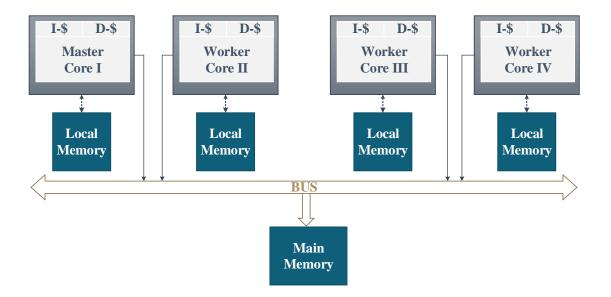
Figure 5.1: System Global Access/Memcpy: In this setup the the ASGUARDIAN is not included in the system. In the Global Access case the worker core accesses the main memory directly through the available interconnection module. In the Memcpy case each worker transfers all task descriptors and arguments to its local memory (hence keeps a task copy), executes all assigned tasks, and then commits back all results to the main memory.
