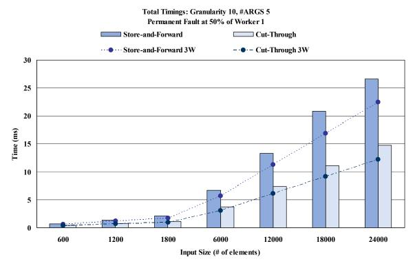
Figure 5.9: Total Timings with One Permanent Fault at 50%: The graph presents the total timing results when one worker core has a permanent fault at 50% of its workload. In addition, the lines present the total timings for three worker cores. The remaining 50% of the workload is distributed among the remaining workers evenly. The available memory transfer modes are store-and-forward and cut-through, since the unreliable versions would have failed.
