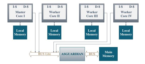
Figure 5.4: System store-and-forward: In this setup the ASGUARDIAN communicates with the cores only through "BUS Lite" and the ASGUARDIAN does not have direct access to worker local memories. Memory transfers from/to the main memory to/from the local memories are performed in a store-and-forward fashion.
