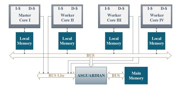
Figure 5.3: System cut-through: In this setup the ASGUARDIAN communicates with the cores through "BUS Lite" and is connected to the local memories of the cores through "BUS". Memory transfers from/to the external memory to/from the local memories are performed in a cut-through fashion.
