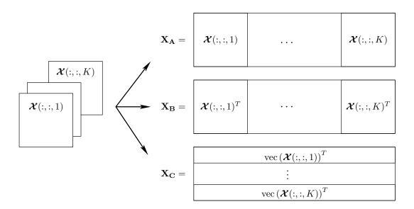
Figure 5.1: Tensor  $\mathcal{X}$  and its matricizations  $\mathbf{X}_{\mathbf{A}}$ ,  $\mathbf{X}_{\mathbf{B}}$ , and  $\mathbf{X}_{\mathbf{C}}$ , in terms of the frontal slices  $\mathcal{X}(:,:,k)$ , for  $k = 1, \ldots, K$ .
