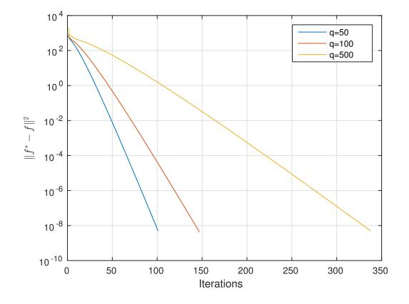
Figure 3.1: The convergence of Nesterov algorithm, for the vector NNLS problem for different conditions q = 50, 100, 500. The problem dimension is n = 1000.
