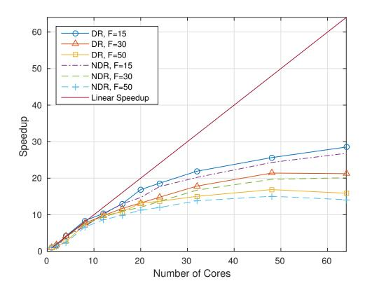
Figure 5.2: Speedup diagram of the Nesterov-based AO NTF algorithm, for rank F = 15, 30, 50, with data replication (DR) and with no data replication (NDR). The tensor size is  $1000 \times 1000 \times 1000 \times 1000$  (8 Gb).
