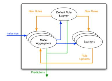
Figure 3.3: Hybrid AMRules (HAMR) with multiple Model aggregators and separate Default Rule Learner
