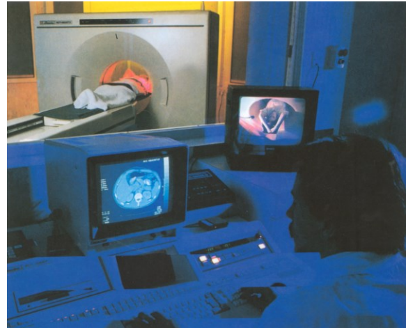
Figure 3.1 Spiral CT scanning principle. The X-rays source and oppositely mounted detectors in rows perform two motions: 1. rotation around the axis, 2. longitudinal movement along the axis. In this way, a large anatomic volume can be scanned rapidly [16].
