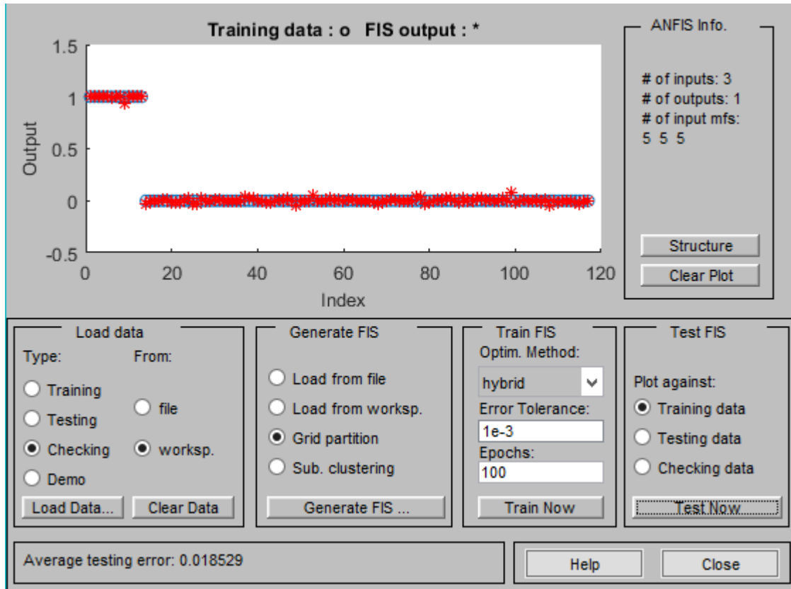
Figure 67: Thesis results of ANFIS based on GLCM using the whole dataset. Training plot of ANFIS with inputs the features of energy, homogeneity and kurtosis that were extracted with GLCM matrix from MRI without pre-processing and ROI segmentation
