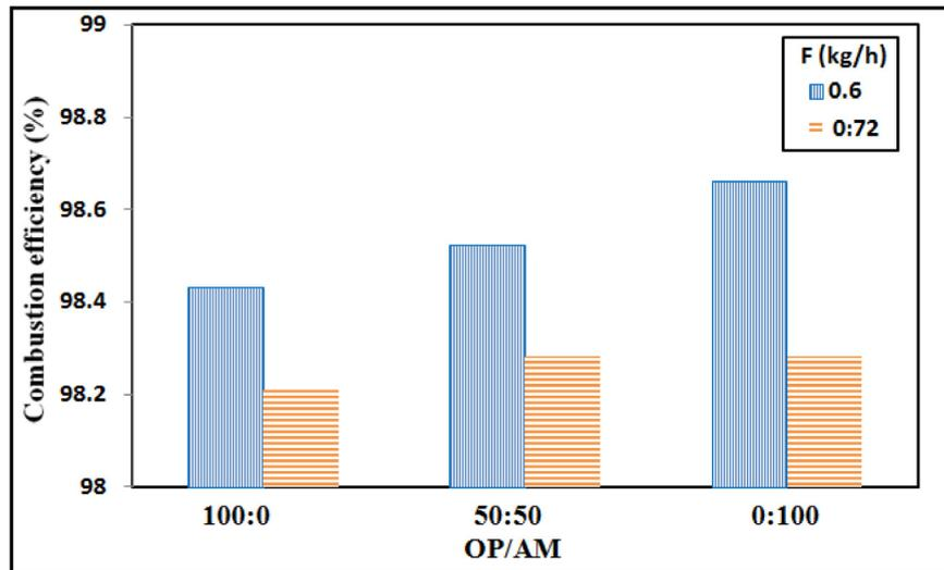
**Fig. 6.** Effect of fuel loading on combustion efficiency of fuels and their blends at  $\lambda = 1.4$ .
