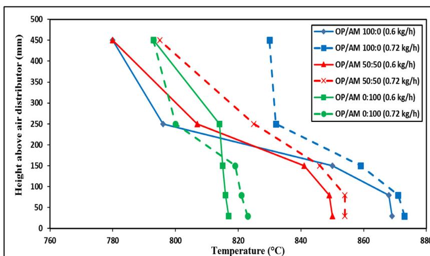
Fig. 4. Temperature profiles of the fuels and their blends along the reactor height at  $\lambda = 1.3$ , as a function of feed rate.
