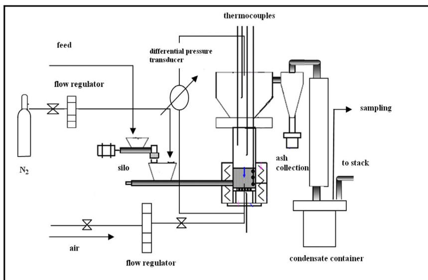
Fig. 1. Schematic diagram of the fluidized bed system.
