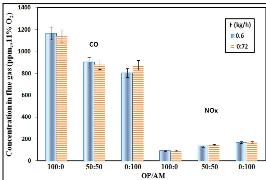
Fig. 5. Average ( $\pm$  standard error) flue gas emissions of the fuels and their blends at  $\lambda = 1.3$ , as a function of feed rate.
