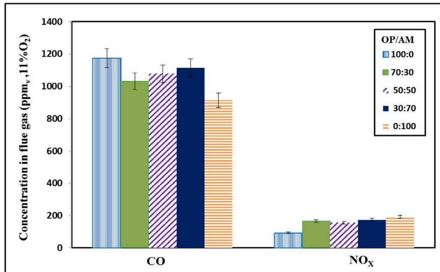
**Fig. 3.** Average ( $\pm$  standard error) flue gas emissions of the fuels and their blends at  $F = 0.6$  kg/h and  $\lambda = 1.4$ .
