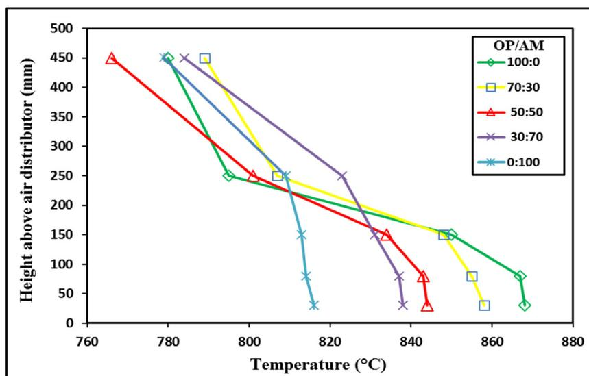
**Fig. 2.** Temperature profiles of the fuels and their blends along the reactor height at  $F = 0.6$  kg/h and  $\lambda = 1.4$ .
