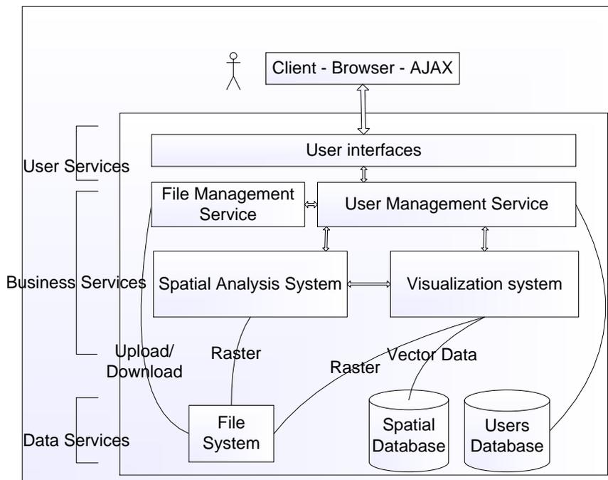
**Fig.1: Open source web mapping portal with decision support system**
