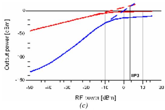
Fig.4. (a) CG vs. RF power, (b) NF vs. inductance L, (c) Output power vs. RF power
