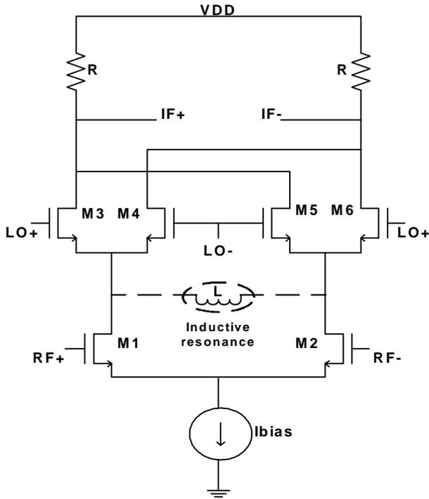
Fig.3. Schematic of the Gilbert cell mixer with inductive resonance technique
