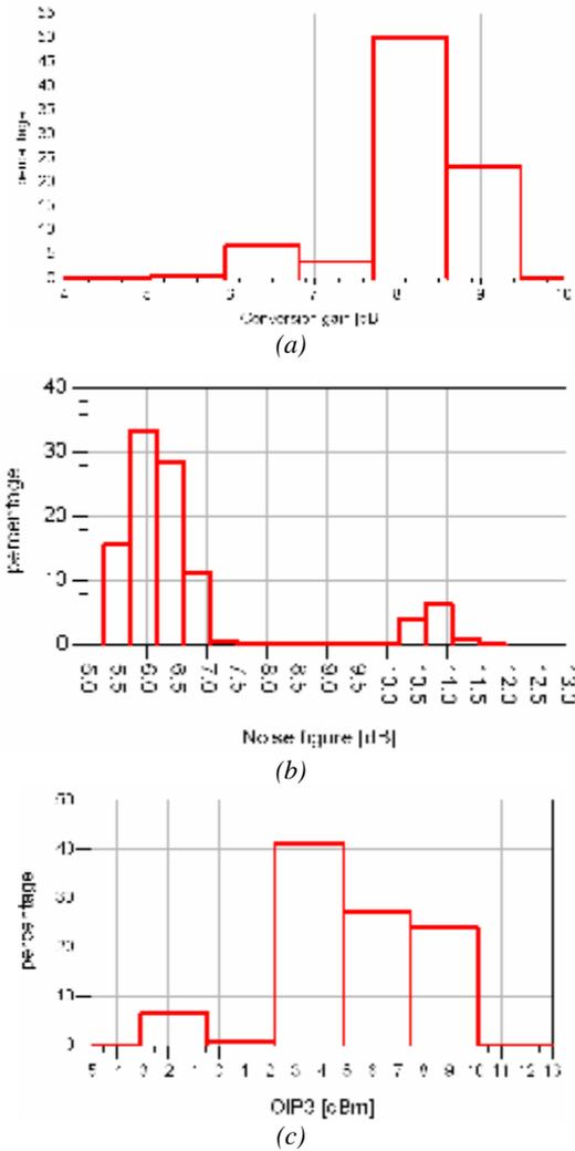
Fig.5. Monte Carlo analysis for (a) CG, (b) NF, (c) OIP3
