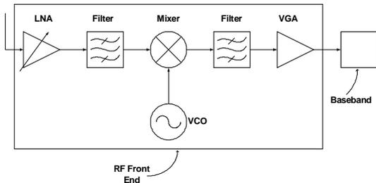
Fig. 1. Direct-conversion receiver
