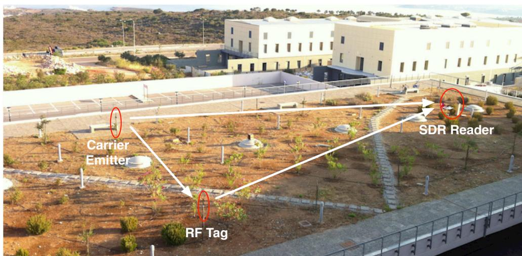
Figure 4.8: Experimental setup outdoor deployment.
