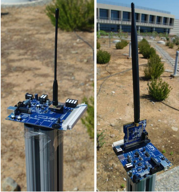
Figure 4.6: Left: RF tag prototype. Right: Carrier emitter.
