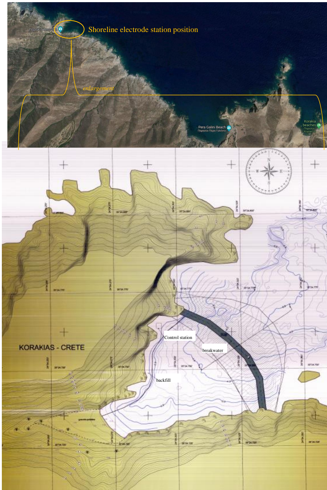
Figure 12. Shoreline electrode station at Korakia beach, Crete [78].
