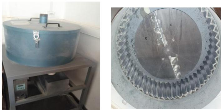
**Fig7.** Centrifugal crusher showing hard steel blade
