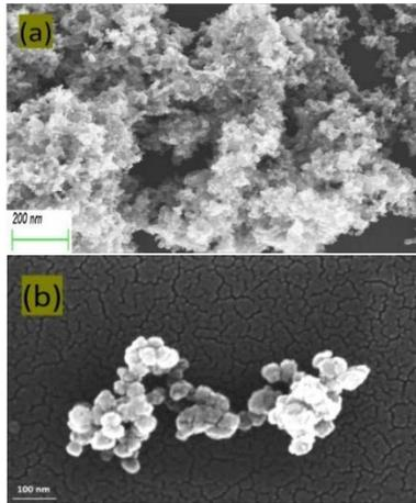
FIGURE 1. FE-SEM images of the NPs in high magnifications: (a) TiO<sub>2</sub> NPs, (b) SiC NPs.
