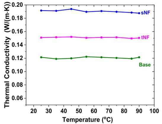
FIGURE 7. Change of the thermal conductivity of the samples in question as a function of temperature (range 25-90 °C).
