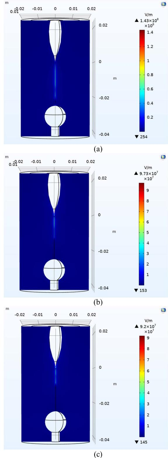
**FIGURE 15.** Electric field distribution in 3D across the gap at  $t = 15 \mu s$  after the application of the 75 kV LIV for: (a) Matrix oil, (b) TNF, (c) sNF.
