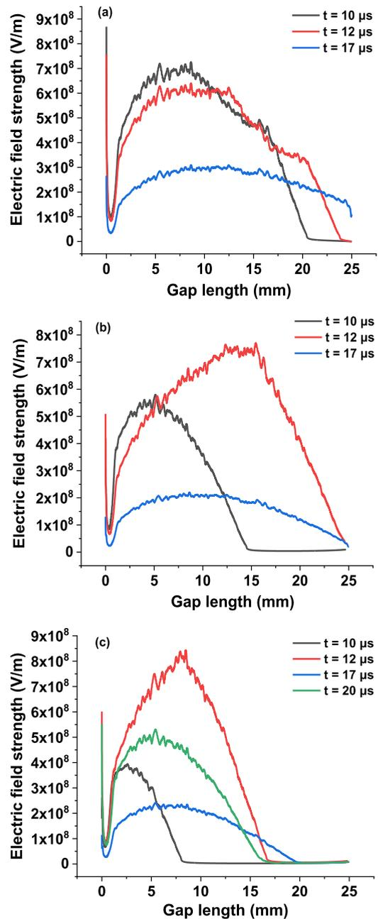
**FIGURE 19.** Electric field distribution across the gap at  $t = 10, 12$  and  $17 \mu s$  after the application of the 80 kV LIV for (a) Matrix oil, (b) tNF and  $t = 10, 12, 17$  and  $20 \mu s$  for (c) sNF.
