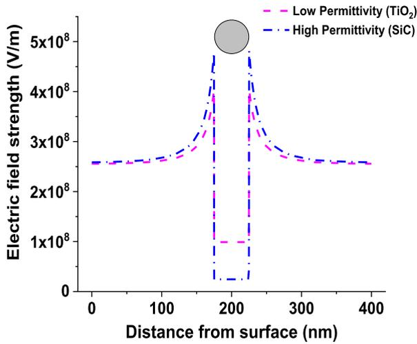
FIGURE 11. Simulated electric field distribution around the surface of SiC and TiO<sub>2</sub> NP.
