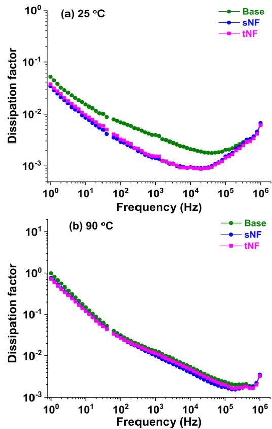
FIGURE 9. Spectral change of dissipation factor of the samples in question (range 1-10<sup>6</sup> Hz): (a) at 25 °C, (b) at 90 °C.
