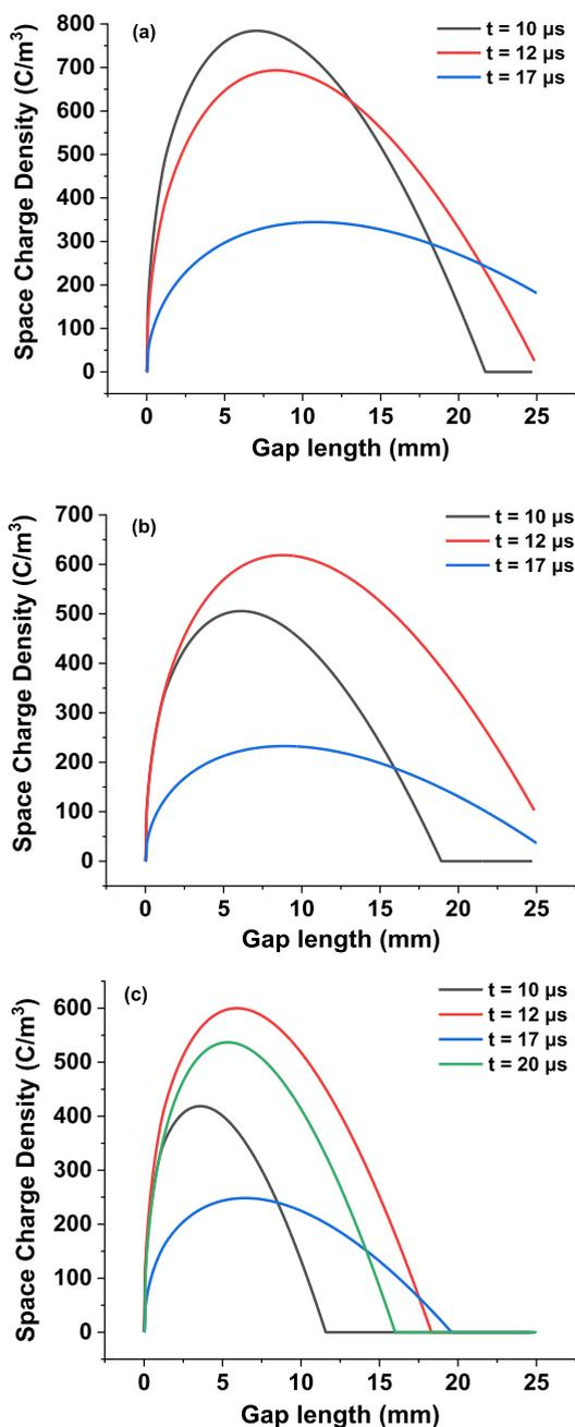
**FIGURE 20.** Space charge density across the gap at  $t = 10, 12$  and  $17 \mu\text{s}$  after the application of the 75 kV LIV for: (a) Matrix oil, (b) tNF, (c) sNF.
