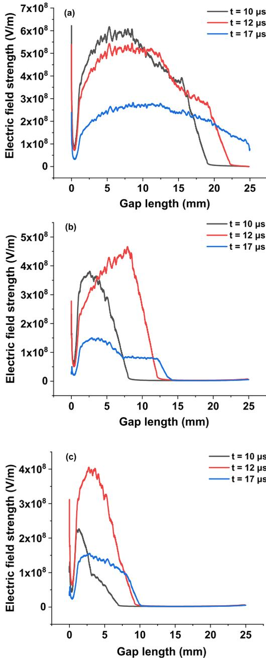
**FIGURE 16.** Electric field distribution across the gap at  $t = 10, 12$  and  $17 \mu s$  after the application of the 75 kV LIV for: (a) Matrix oil, (b) tNF, (c) sNF.
