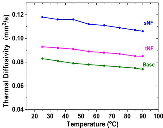
FIGURE 6. Change of the thermal diffusivity of the samples in question as a function of temperature (range 25-90 °C).
