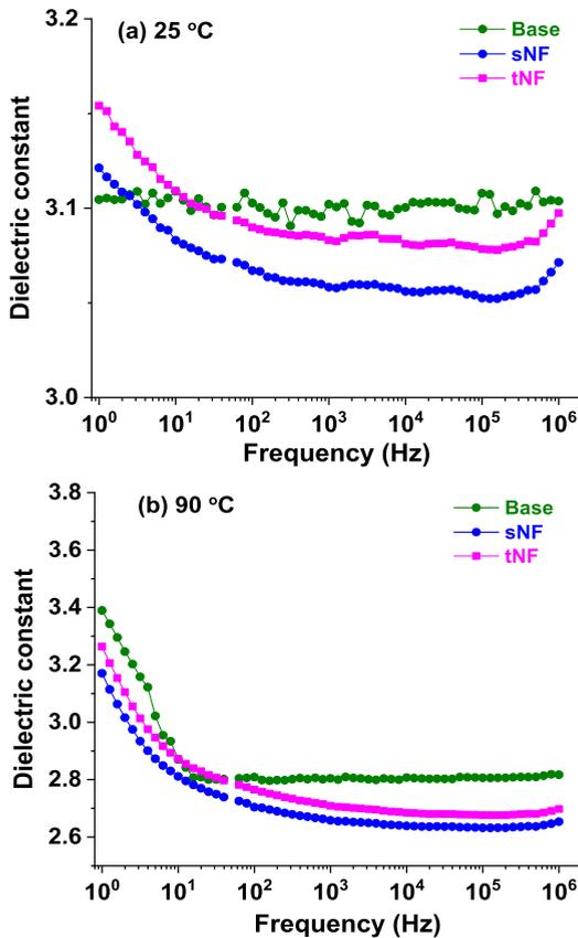
FIGURE 8. Spectral change of dielectric constant of the samples in question (range 1-10<sup>6</sup> Hz): (a) at 25 °C, (b) at 90 °C.
