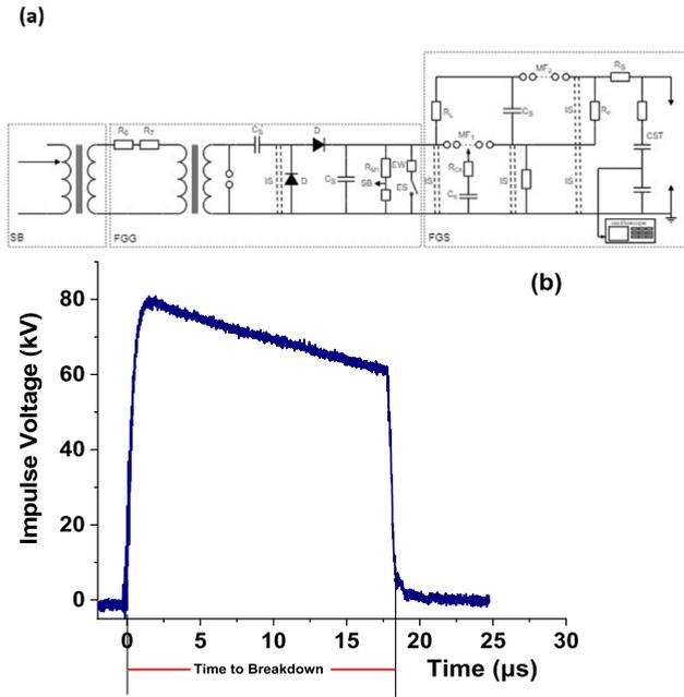
FIGURE 5. (a) Equivalent circuit of the impulse generator, (b) Typical LI waveform (1.2/50 μs) displaying the breakdown time.
