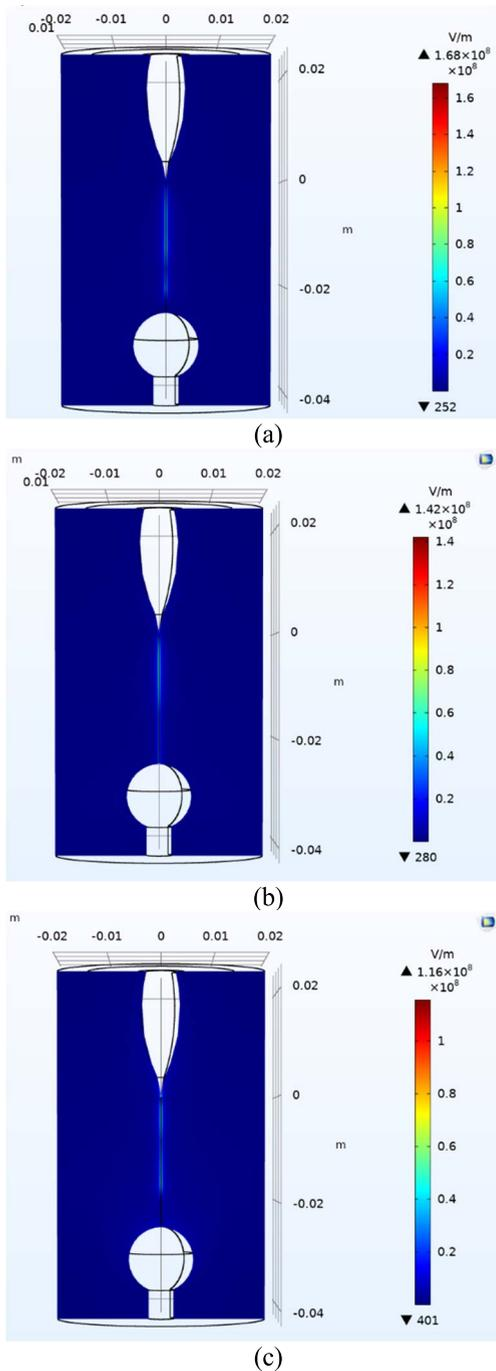
**FIGURE 18.** Electric field distribution in 3D across the gap at  $t = 15 \mu s$  after the application of the 80 kV LIV for: (a) Matrix oil, (b) tNF, (c) sNF.
