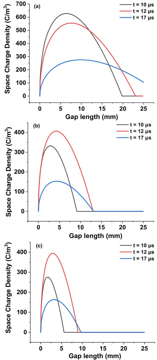
**FIGURE 17.** Space charge density across the gap at  $t = 10, 12$  and  $17 \mu s$  after the application of the 75 kV LIV for: (a) Matrix oil, (b) tNF, (c) sNF.
