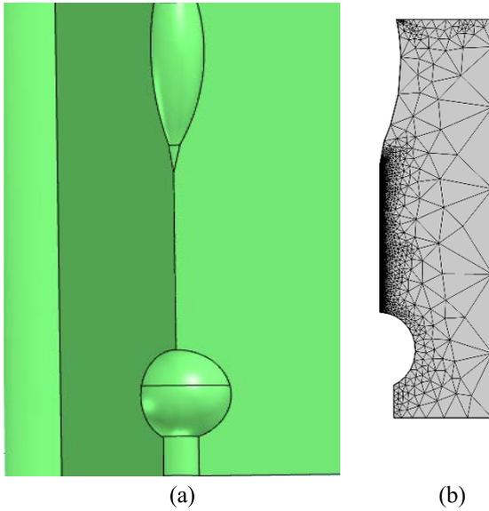
**FIGURE 14.** (a) Point-sphere gap in COSMOL Multiphysics environment before the application of Lightning Impulse Voltage, (b) Mesh distribution across the gap.
