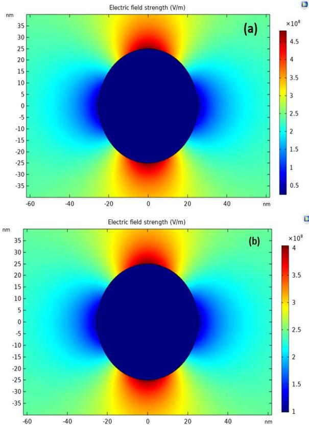
FIGURE 12. 3D plot of electric field distribution around each NP: (a) TiO<sub>2</sub> NP, (b) SiC NP.
