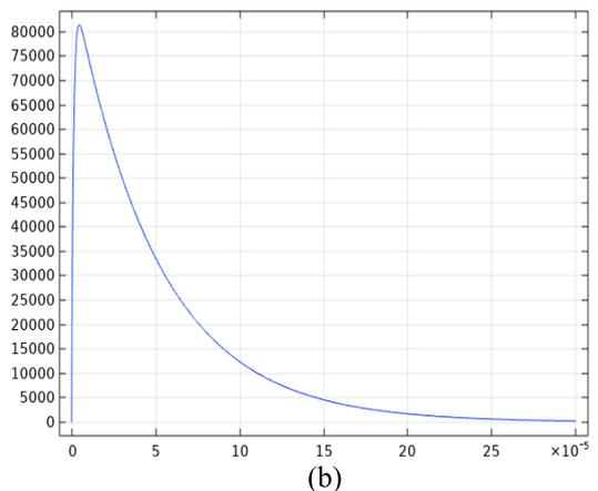
FIGURE 13. Lightning Impulse waveforms for the two simulation cases: (a) 75 kV, 1.2/50  $\mu\text{s}$ , (b) 80 kV, 1.2/50  $\mu\text{s}$ .
