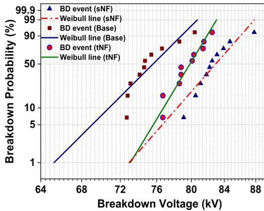
FIGURE 10. Weibull plot of the LI breakdown events for the matrix and the two nanofluid samples under investigation.
