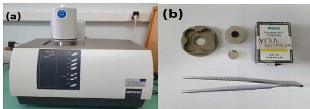
**FIGURE 4.** (a) NETZSCH LFA 467 Hyper Flash apparatus, (b) LFA test cell along with the liquid samples.
