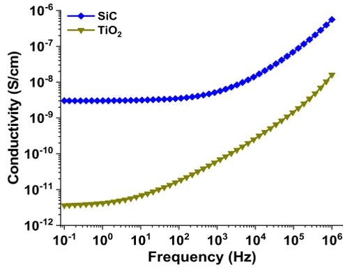
**FIGURE 3.** Change of electrical conductivity versus frequency for: (a) the used NPs, (b) the matrix.
