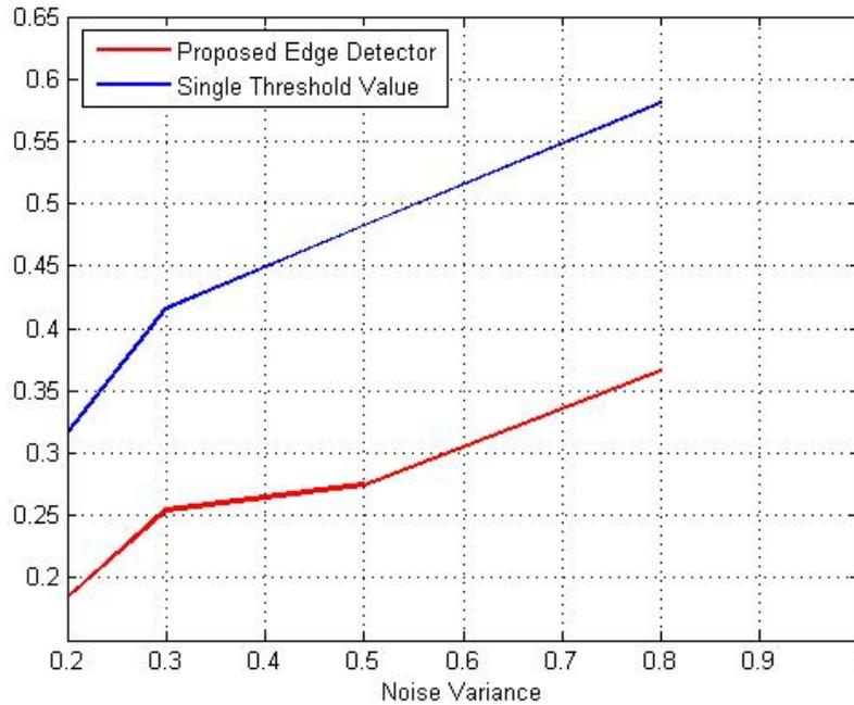
*Figure 1: Performance of the algorithm in terms of the RMSE using the proposed edge detector vs. using a single threshold value.*
