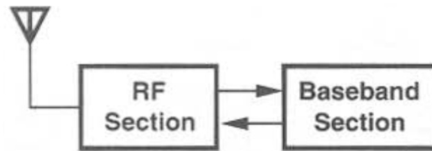
Fig.4 RF and baseband processing in a transceiver.
