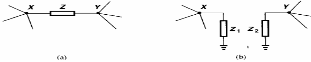
Fig.8 Miller effect on floating impedance.
