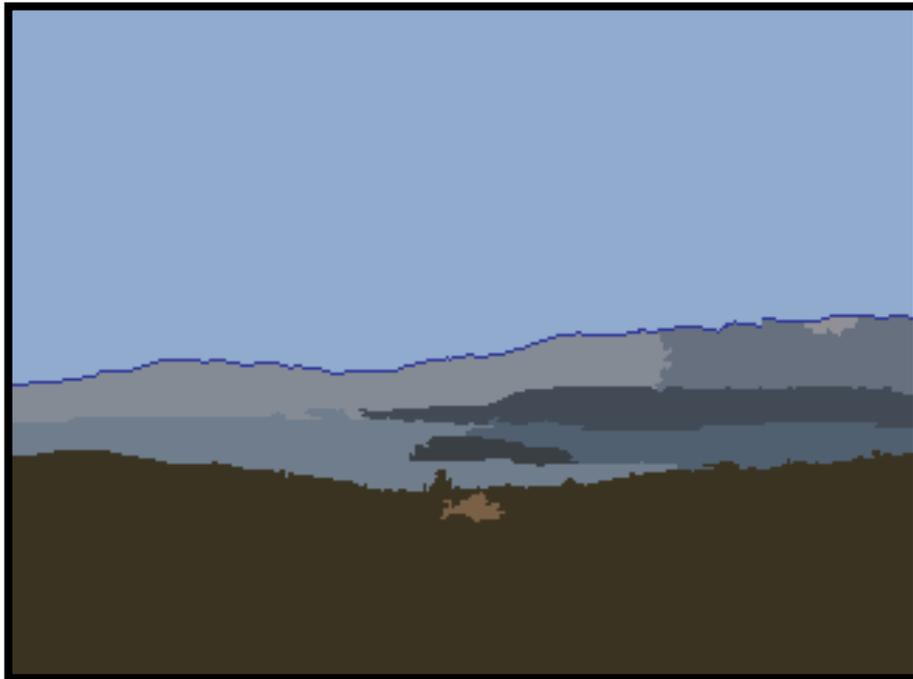
FIGURE 22: DETECTION OF A SINGLE SKY REGION AND EXTRACTION OF THE SKYLINE - RIDGELINE
