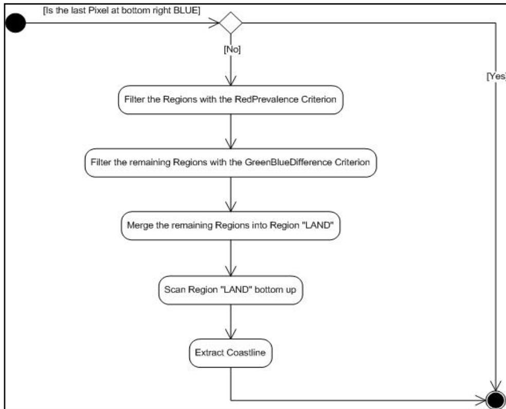
FIGURE 25: ACTIVITY DIAGRAM OF THE LAND DETECTION ALGORITHM
