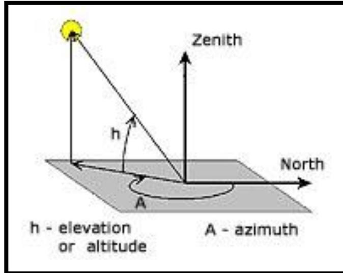
FIGURE 13: AZIMUTH AND ALTITUDE ANGLES
