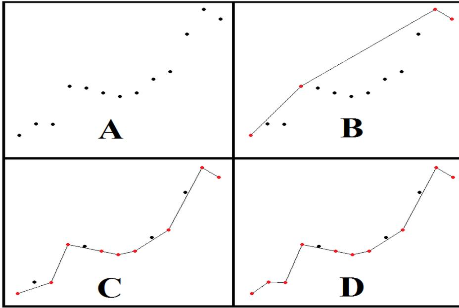
**FIGURE 36: LINE SEGMENT APPROXIMATION EXAMPLE. A) INITIAL POINT SET. B) APPROXIMATION BASED ON COMPUTING THE UPPER CONVEX HULL. C) FURTHER APPROXIMATION AFTER COMPUTING THE LOWER CONVEX HULL. D) FINAL APPROXIMATION USING THE UPPER CONVEX HULL AGAIN FOR THE 3 FIRST POINTS.**
