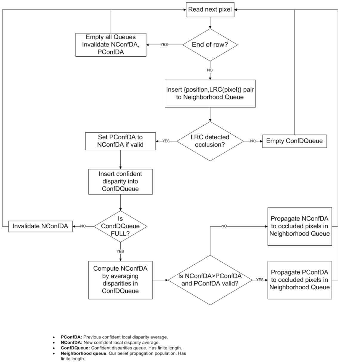
**Fig 14:** Flowchart of our belief propagation algorithm. If we encounter foreground pixels when moving on the background ( $NConfDA > PConfDA$ ), we propagate the background confident disparity ( $PconfDA$ ). The opposite happens when we encounter background pixels whilst on the foreground ( $PconfDA \geq NConfDA$ ).
