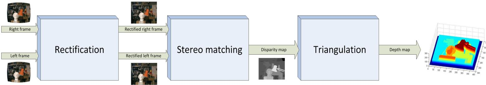
**Fig 4:** General stereo vision system structure.
