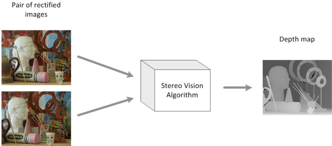
**Fig 1:** Inputs-Output of a stereo vision algorithm. Middlebury 2005 Art dataset.
