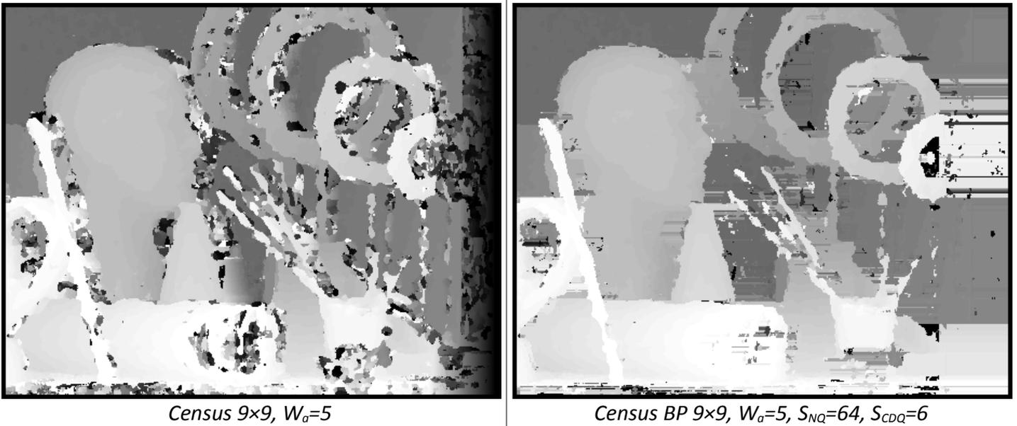
**Fig 22:** Visual comparison of pure census vs census with the proposed belief propagation procedure. Notice how BP fills in previously occluded pixels on object borders and on the right side of the image.
