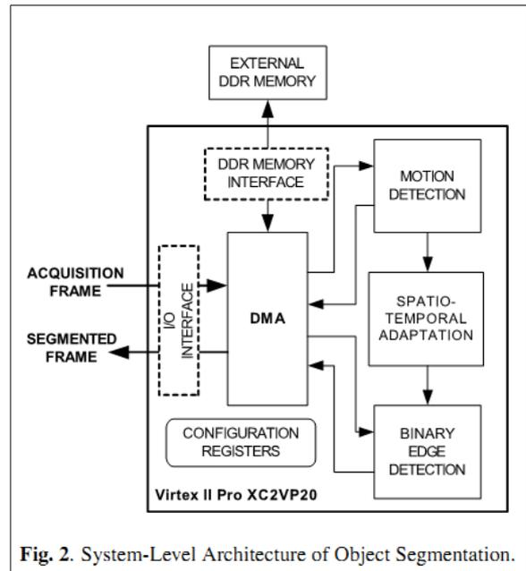
Fig. 2. System-Level Architecture of Object Segmentation.
