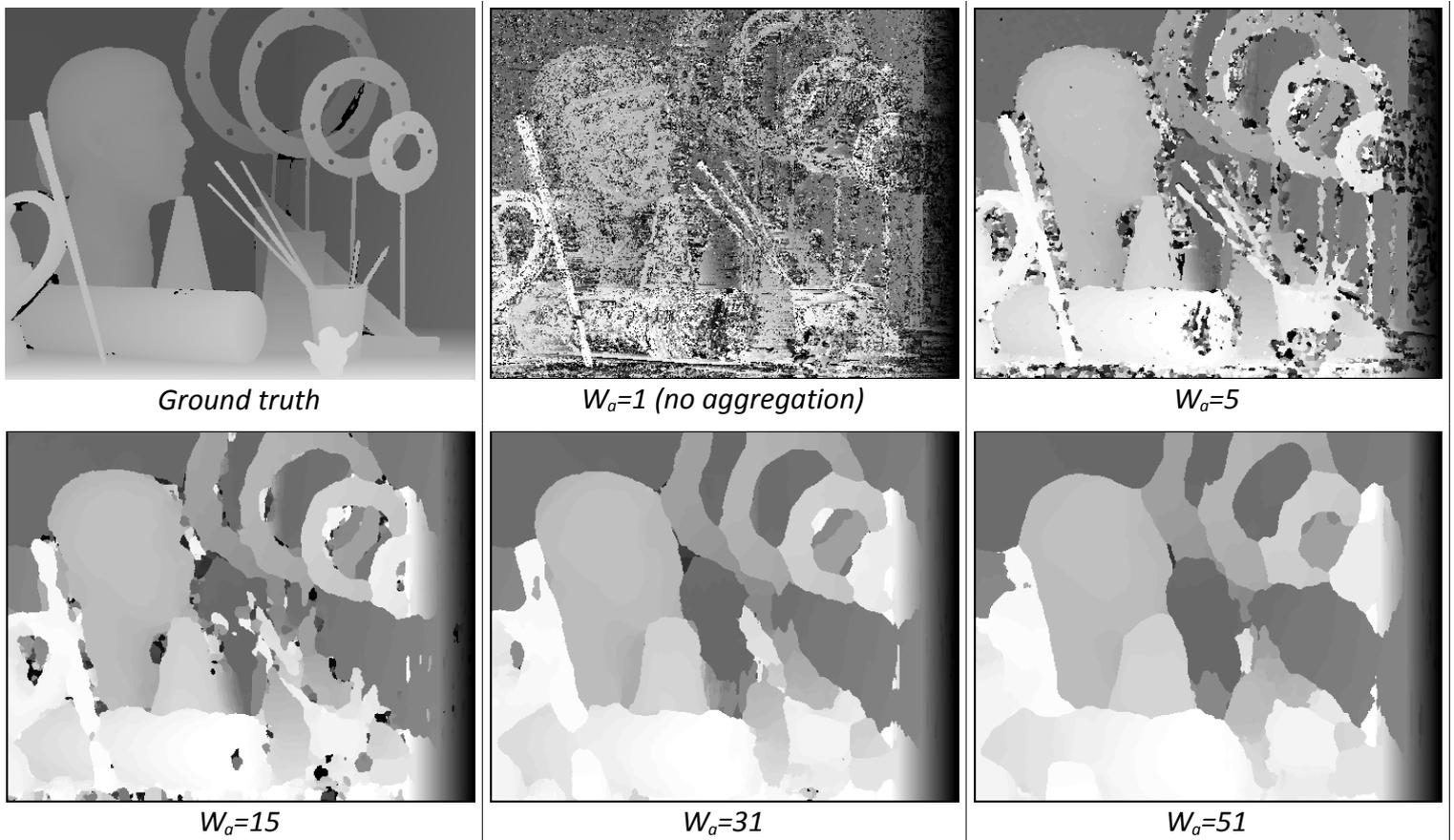
**Fig 15:** The blur effect of increasing aggregation window sizes with a  $5 \times 5$  census.
