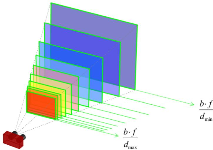
**Fig 17:** Discrete disparity space, illustrating the stereo system's range capabilities. Image courtesy of Stefano Mattoccia.
