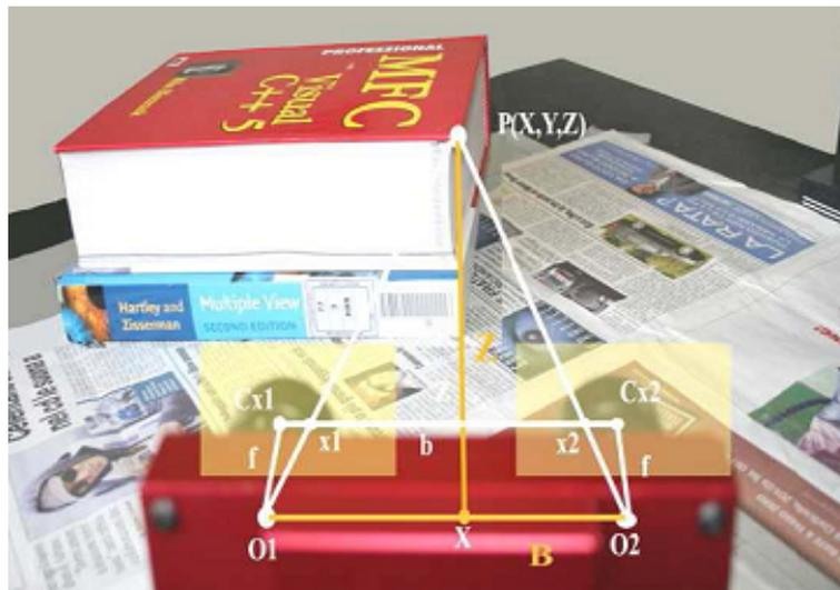
**Fig 2:** Point  $P(X,Y,Z)$  corresponds to points  $x_1$  and  $x_2$  in the two cameras.  $Z$  is the unknown distance of the point,  $f$  the focal length of the cameras and  $b$  the baseline distance between the two cameras. Using these values and the coordinates of  $x_1$  and  $x_2$  in the two images we can extract  $Z$  through triangulation. Image courtesy of Stefano Mattoccia [16].
