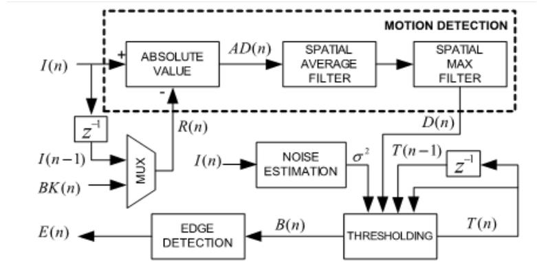
Fig. 1. Block Diagram of the Object Segmentation [9].
