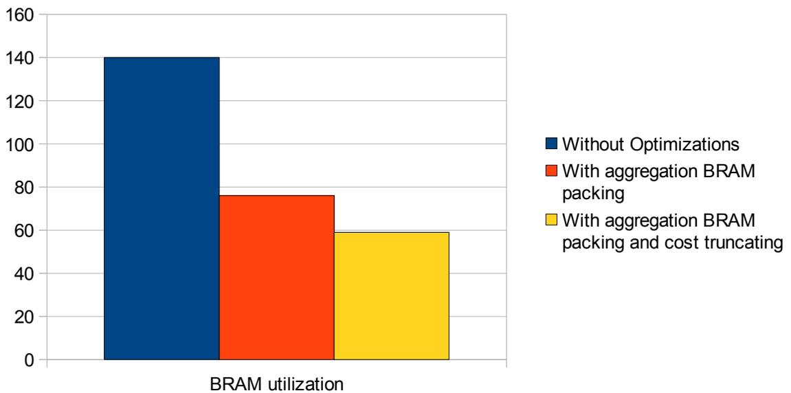
**Fig 33:** Resource savings with optimized aggregation buffer structure.
