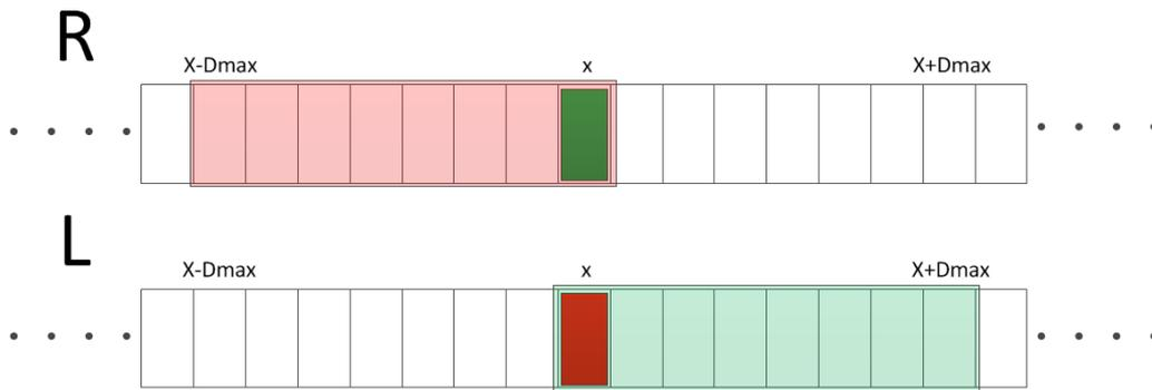
**Fig 29:** At the top row are pixels of the right image, whereas at the bottom are pixels of the left image. The green pixel on the right image has a search space denoted by the green shade on the left image. In order to determine the validity of  $Disp_{RL}(x,y)$  we need all left-to-right disparities in the green space and thus we need right-to-left costs up to  $x+D_{max}$ .
