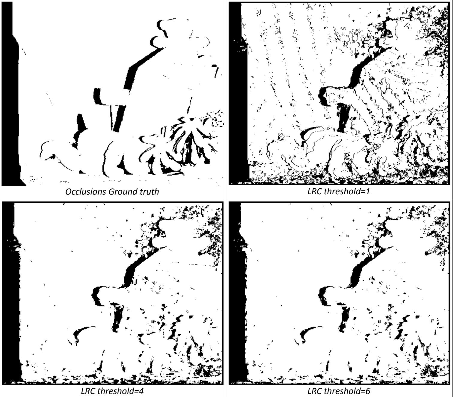
**Fig 21:** Left/Right Consistency check for several values of the LRC threshold.
