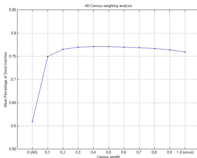
**Fig 11:** AD-Census analysis for different weighting values. X-axis shows the weight of Census,  $c \in [0,1]$ . AD weight is defined as  $1-c$ .
