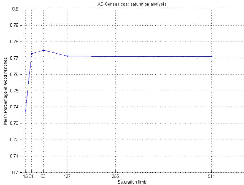
**Fig 32:** Cost size/accuracy analysis. The peak value shifts to the right as the true maximum cost increases.
