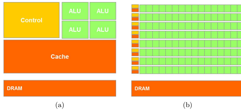
Figure 6.2: (a) Abstract view of a typical CPU architecture, (b) Abstract view of a typical GPU architecture, with 8 multiprocessors, each one having a lot of ALUs
