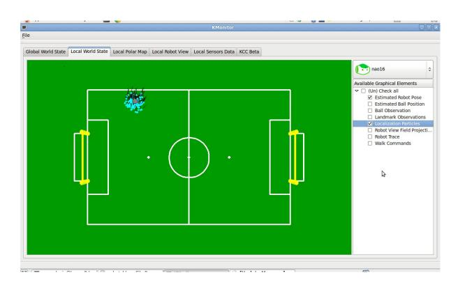
Figure 5.14: Visualization of the localization particles
