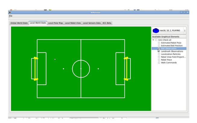
Figure 5.12: Visualization of the instantaneous ball observation
