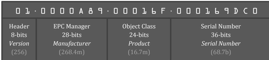
Figure 1.9 – 96-bit EPC structure
