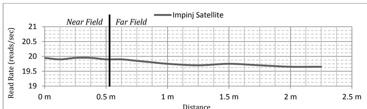
Figure 3.10 – Impinj Satellite Read rate versus Distance
