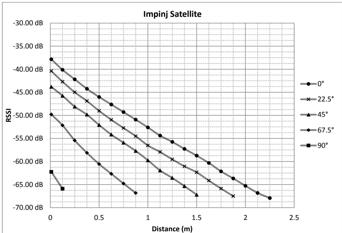
Figure 3.2 - Impinj Satellite Mapping
