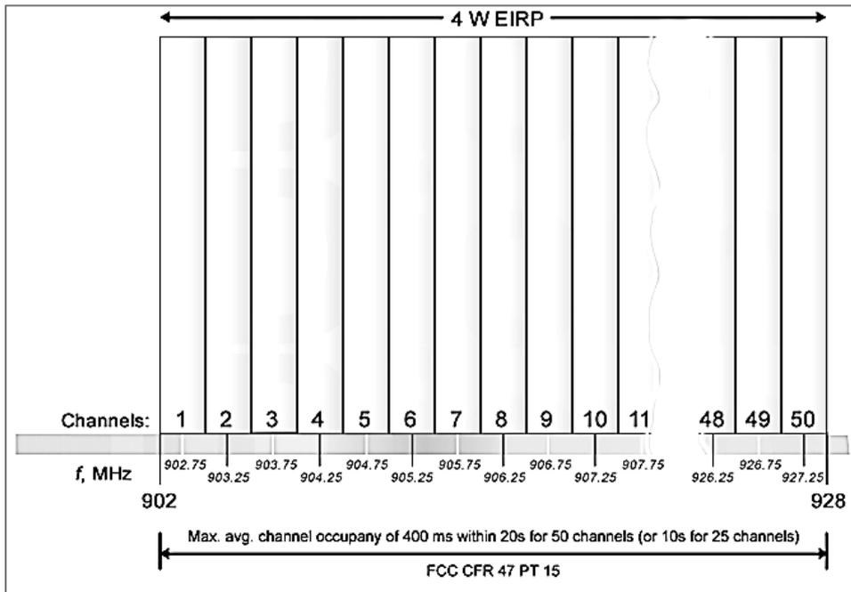
Figure 1.4 - FCC Channels & Power limits
