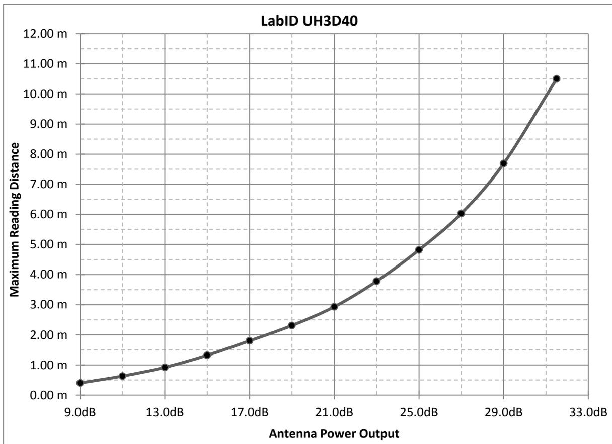
Figure 3.23 - LabID UH3D40 scanning distance versus antenna power output
