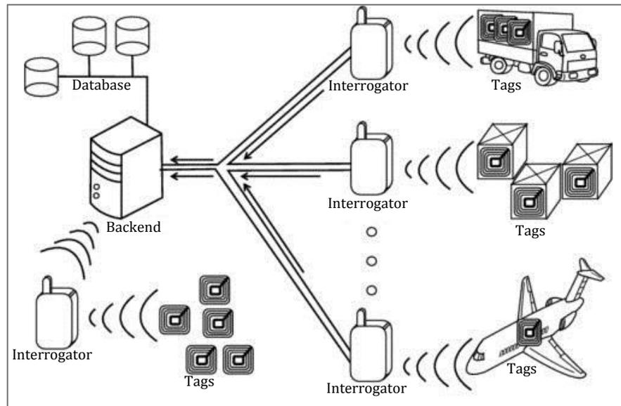
Figure 1.2 – RFID System Components
