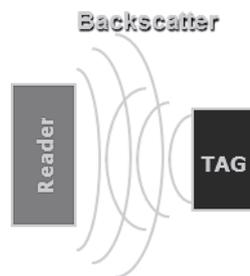
Figure 1.7 - Backscatter coupling
