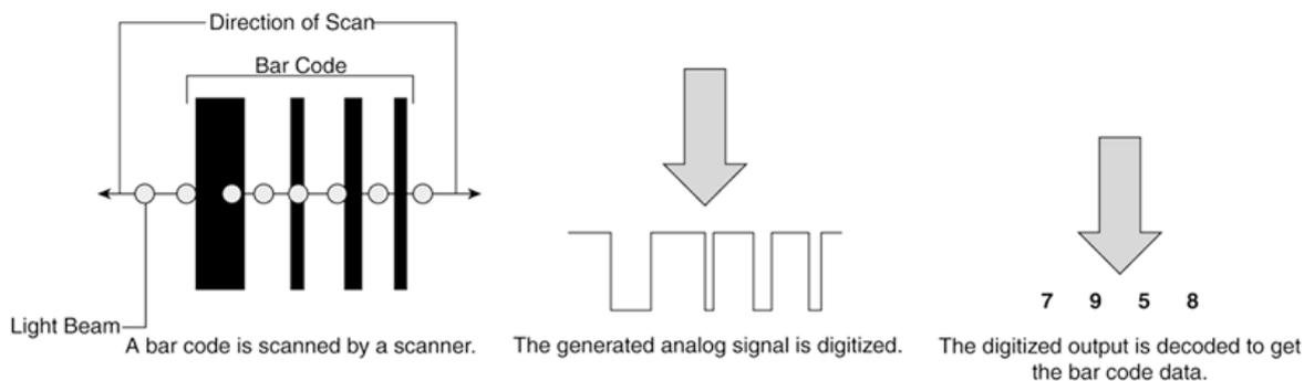
Figure 1.11 - Barcode scanning process
