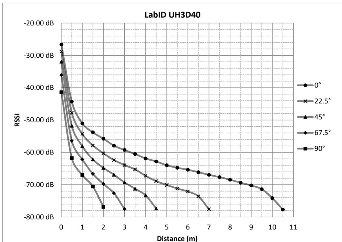
Figure 3.3 - LabID UH3D40 Mapping
