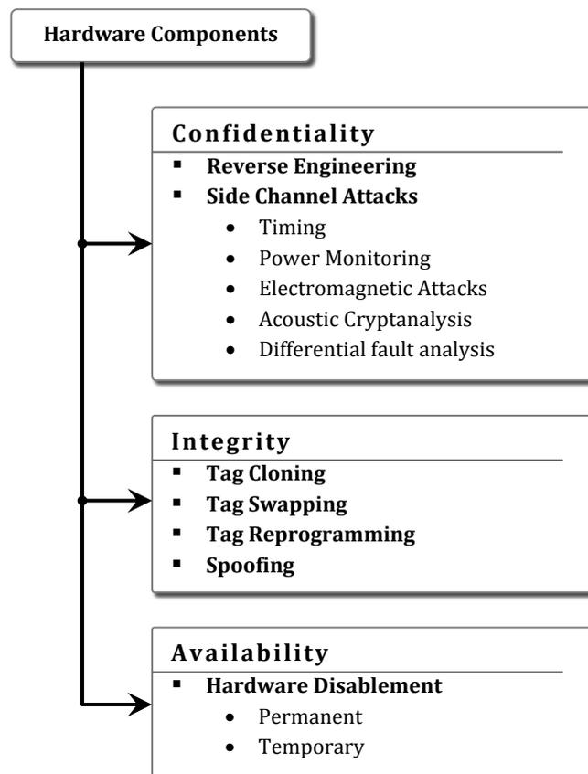
Figure 4.3 - RFID Hardware security threats
