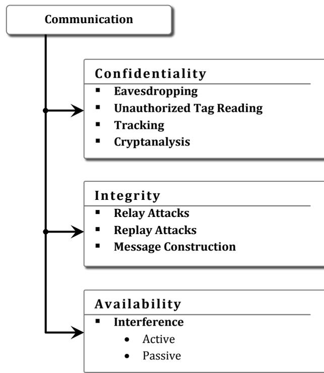
Figure 4.4 - RFID Communication security threats
