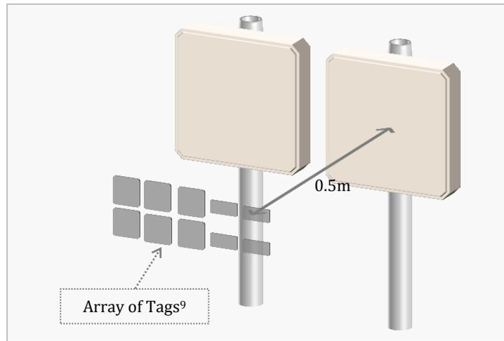
Figure 5.10 - Reader modes evaluation setup
