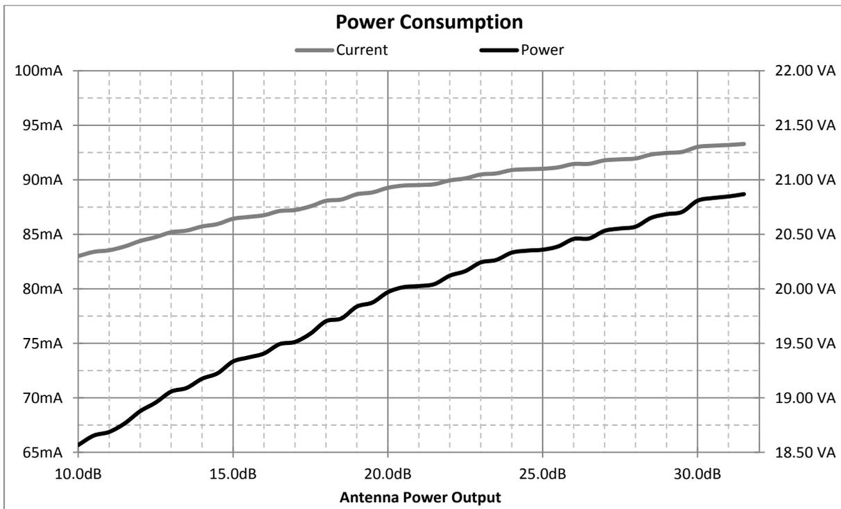
Figure 3.26 – Antenna Power Output versus Power Consumption
