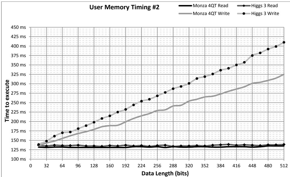
Figure 5.2 - User memory various lengths write performance
