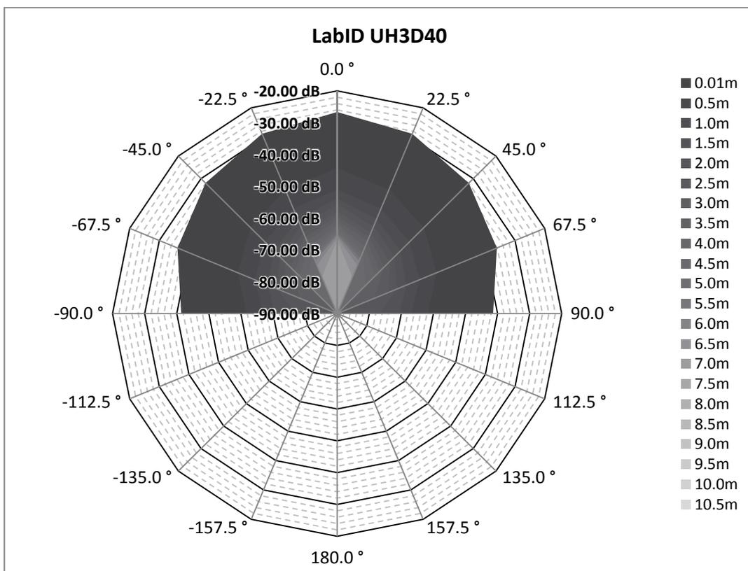
Figure 3.7 – LabID UH3D40 RSSI diagram
