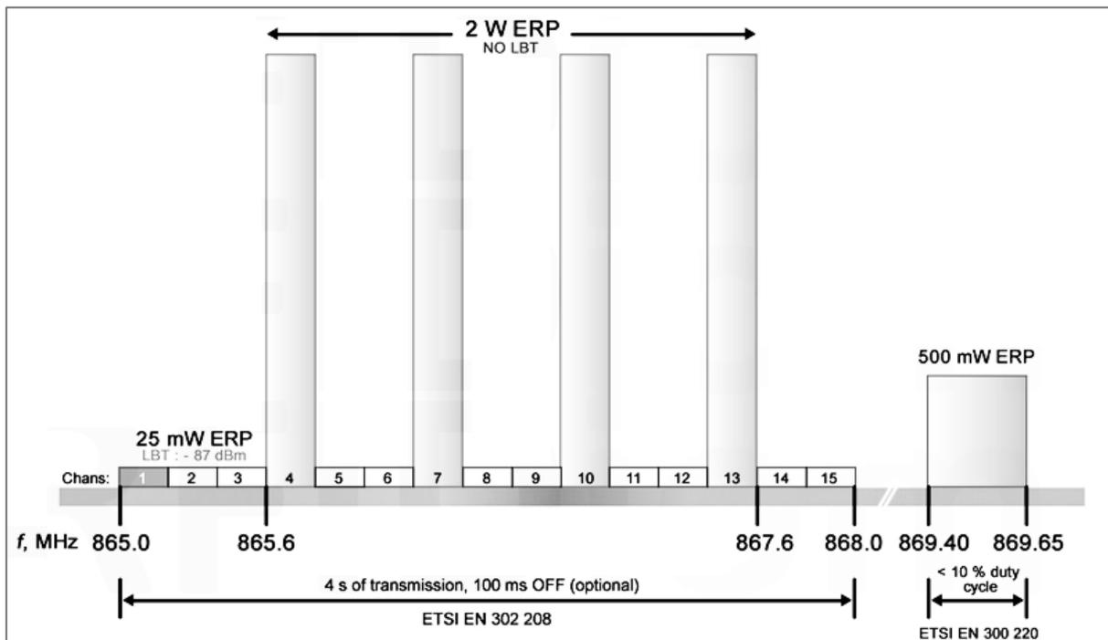
Figure 1.5 - ETSI Channels & Power limits
