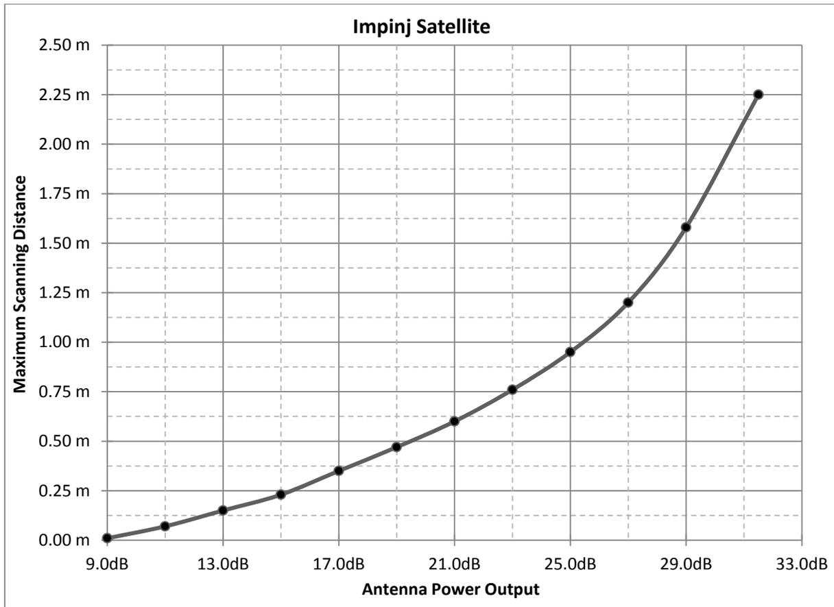
Figure 3.22 - Impinj Satellite scanning distance versus antenna power output
