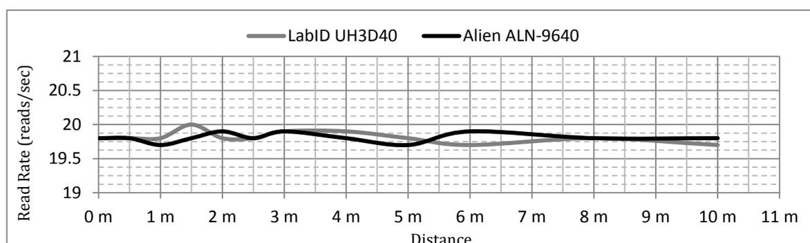
Figure 3.11 – LabID UH3D40 & Alien ALN-9640 Read rate versus Distance
