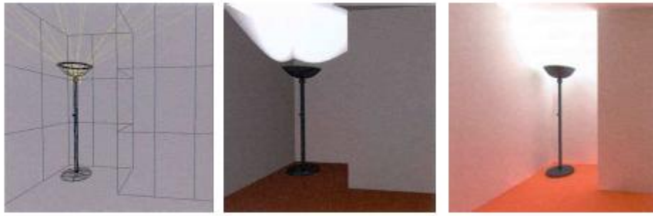
Figure 12: The difference in image quality between ray tracing (middle) and radiosity (right hand image).
