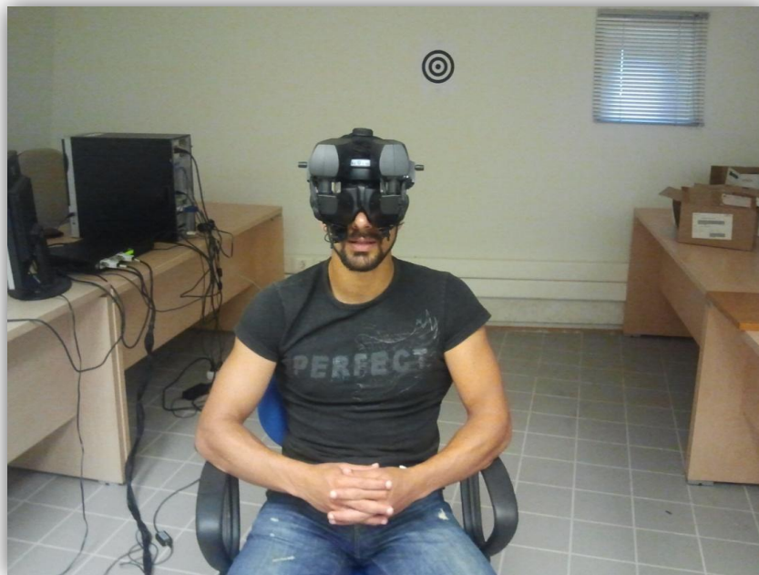
Figure 28: A participant wearing the head mounted display model nVisor SX111 during the experiment.
