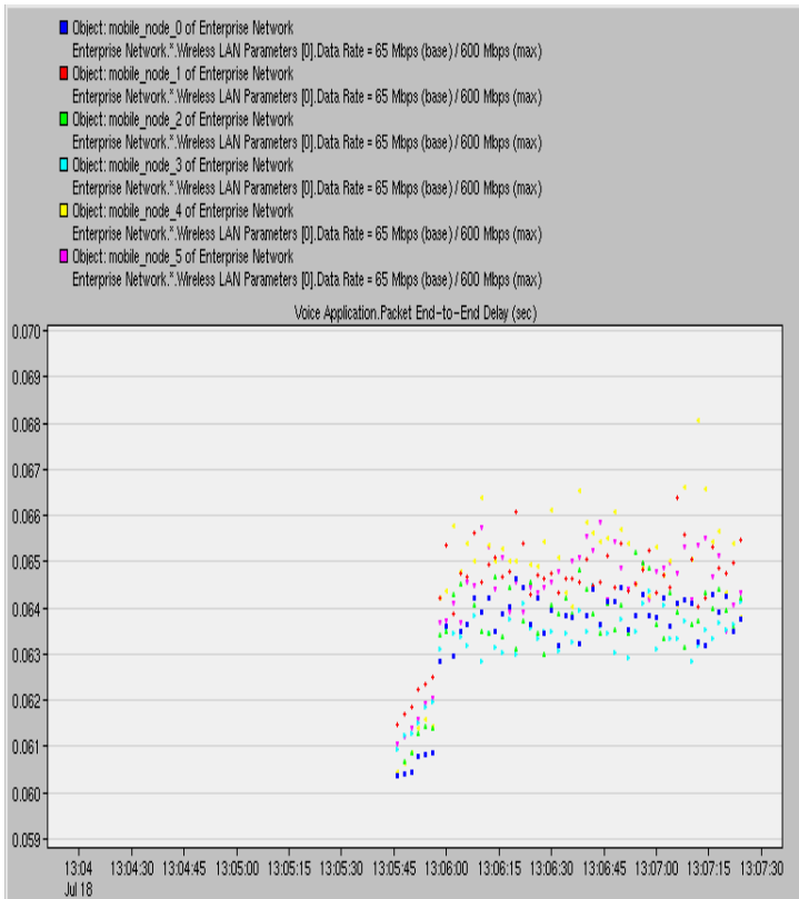
Figure 206: Packet End To End Delay For Each Mobile Node – P2P Links Operating On Channel 6, 5 Calls Per P2P Link
