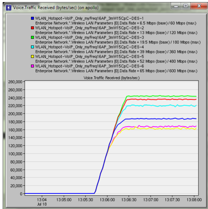
Figure 65: Voice Traffic Received, 15 workstations per cell, 1 call per workstation, IP Telephony Call
