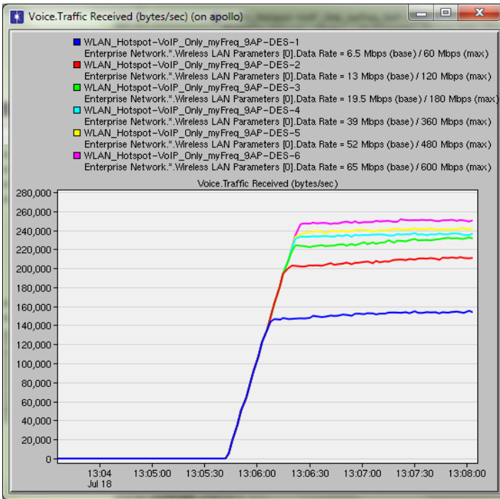
Figure 48: Voice Traffic Received, 1 workstation per cell, 30 calls per workstation, IP Telephony Call
