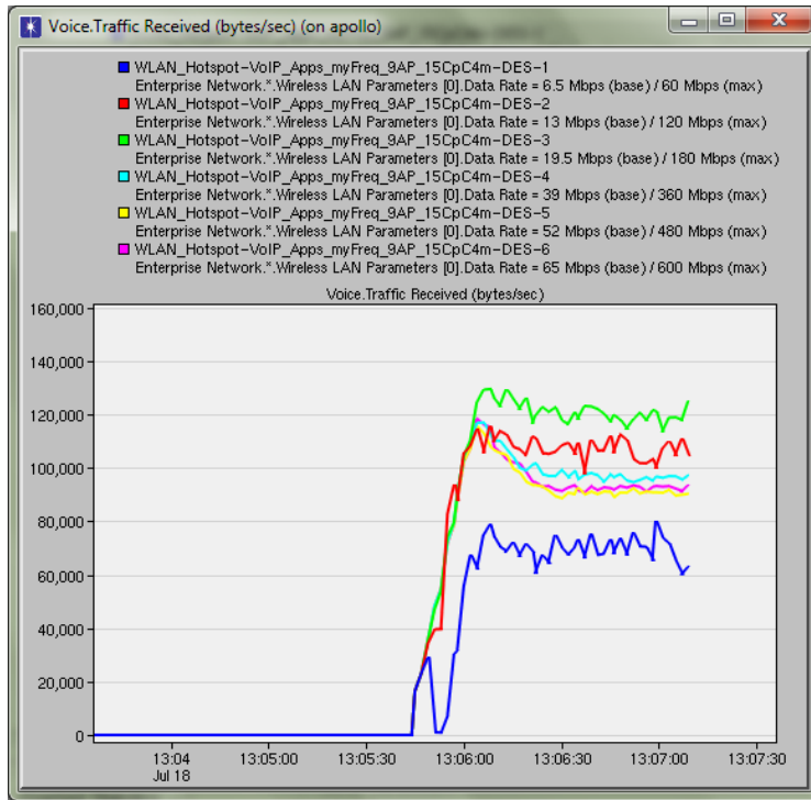
Figure 52: Voice Traffic Received, IP Telephony Call, Applications added in the simulation
