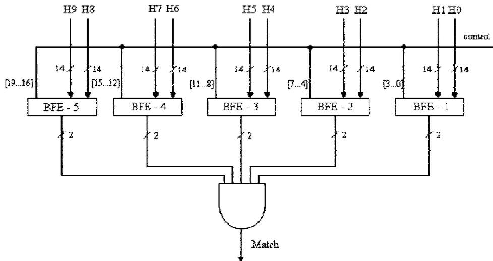
Figure 4.4: An example of a 5-element BF arrangement
