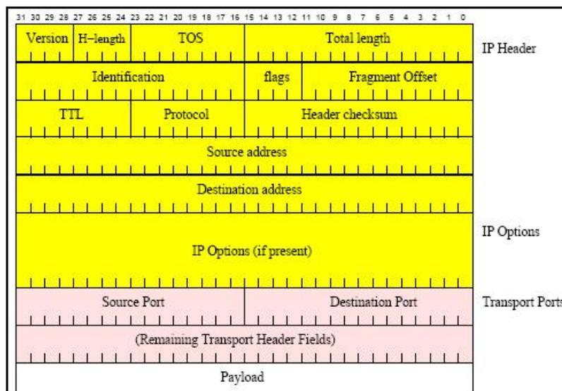
**Figure 1.1: IP header format**
