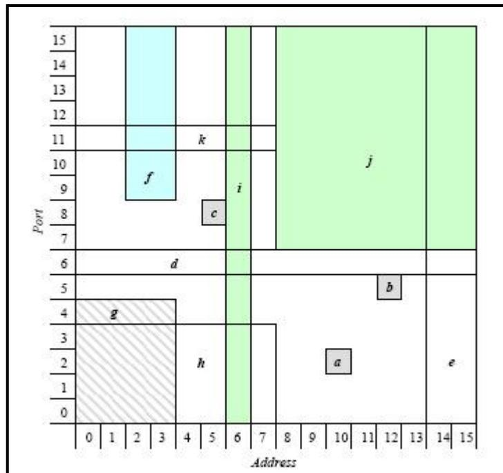
**Figure 2.8: HiCuts geometric representation**
