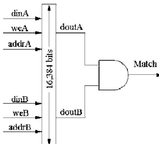
**Figure 4.3: Dual Port Block Ram used as a Bloom Filter Element**
