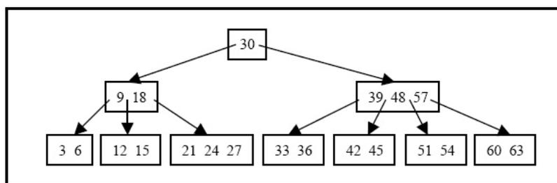
**Figure 2.1: Example B-Tree data structure**
