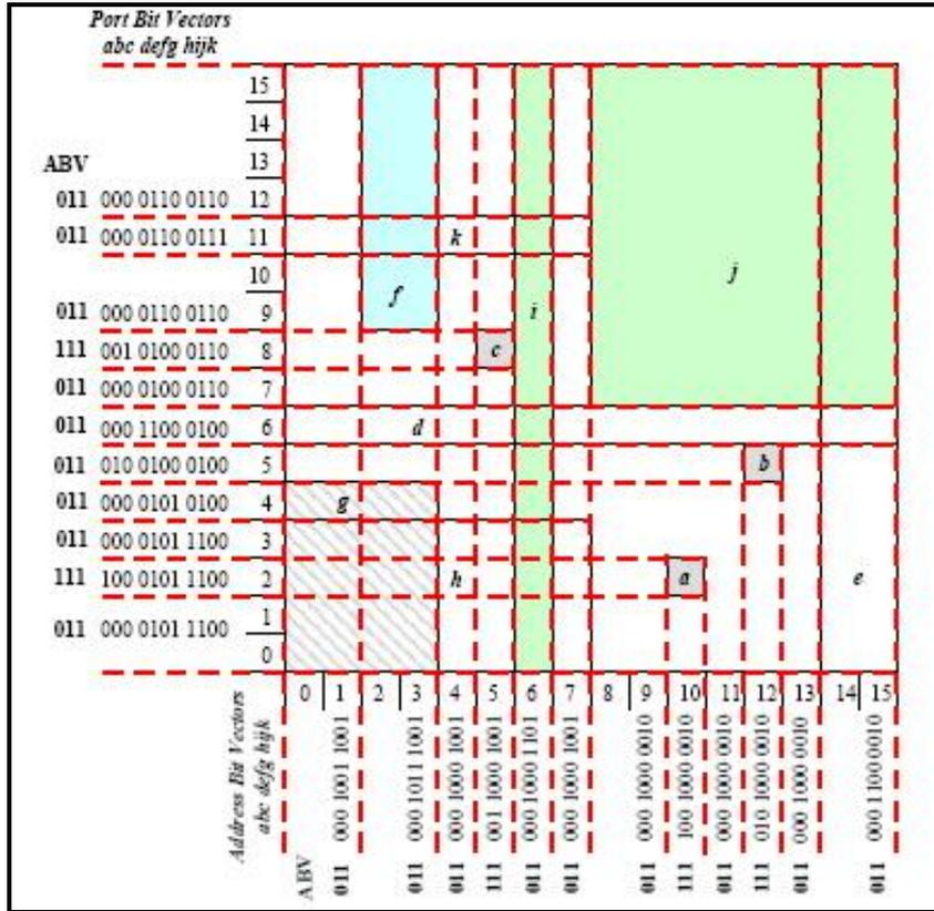
Figure 2.12: Aggregated Bit Vector example
