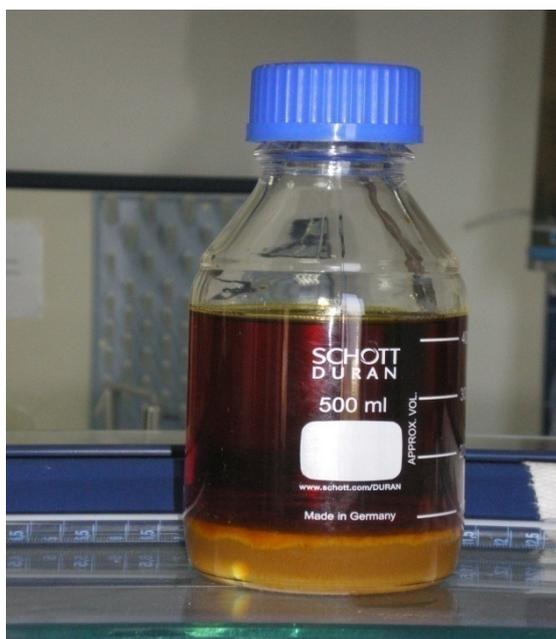
**Fig 6. 8 - Alkali transesterification (lower layer contains glycerin, soapstock and impurities while upper layer is CPO methyl ester)**
