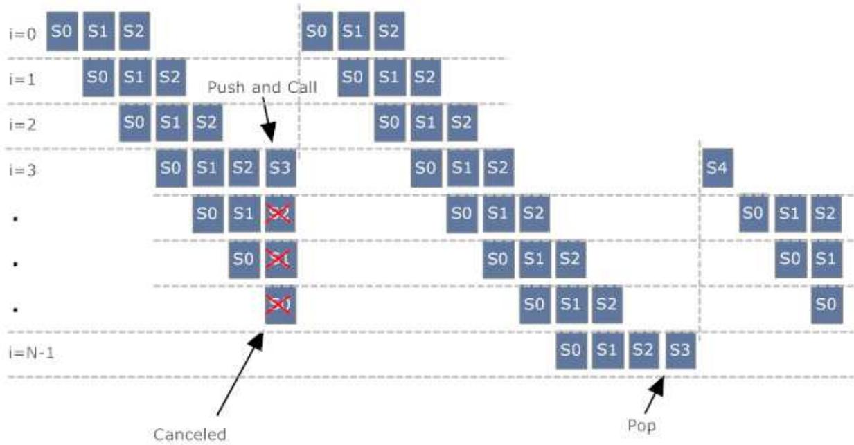
Figure 12 : Stage transition for the Knight's Tour speculative execution
