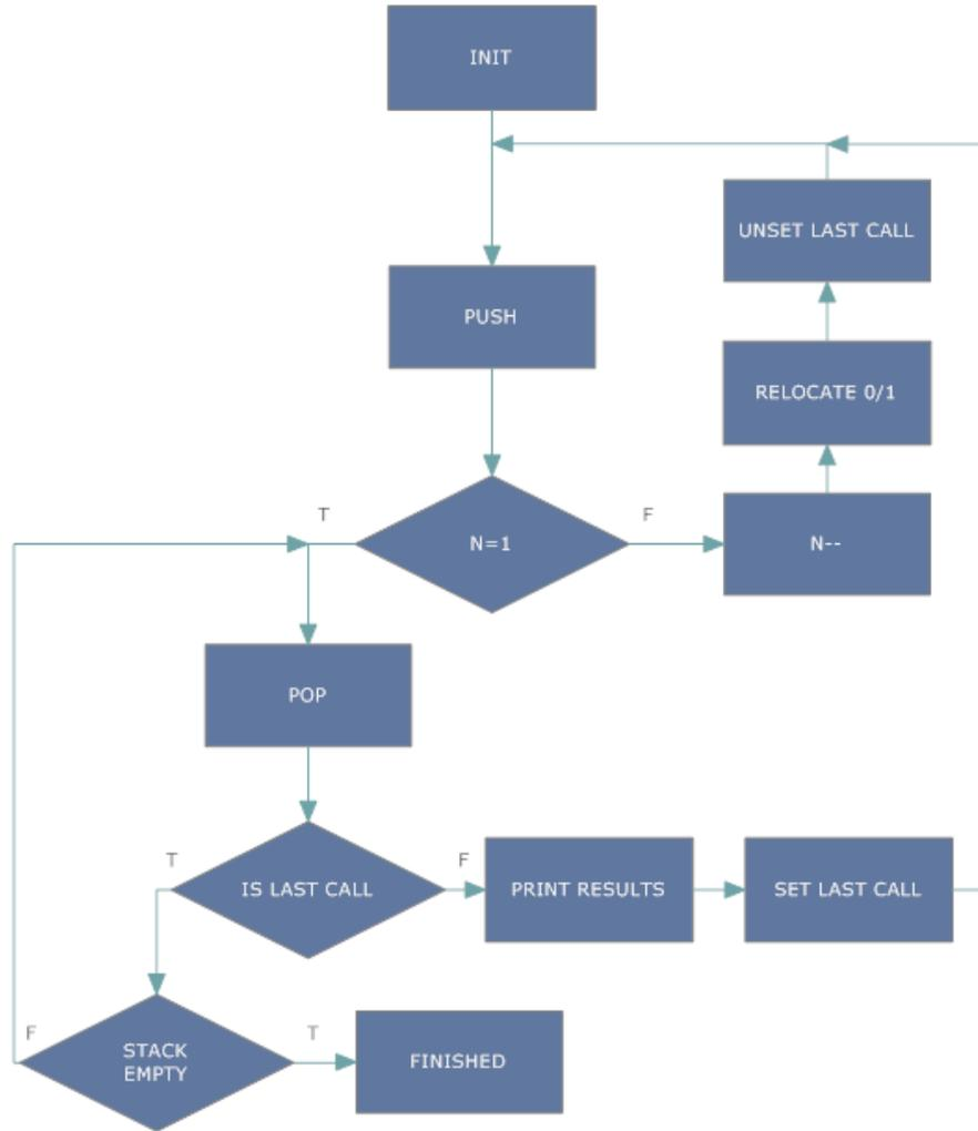
Figure 29 : The Towers of Hanoi ASM
