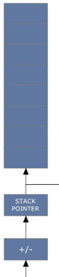
Figure 35 : Single cycle stack implementation
