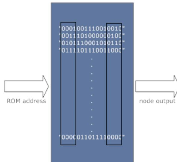
**Figure 40 : ROM contents example for a binary tree of depth 4**
