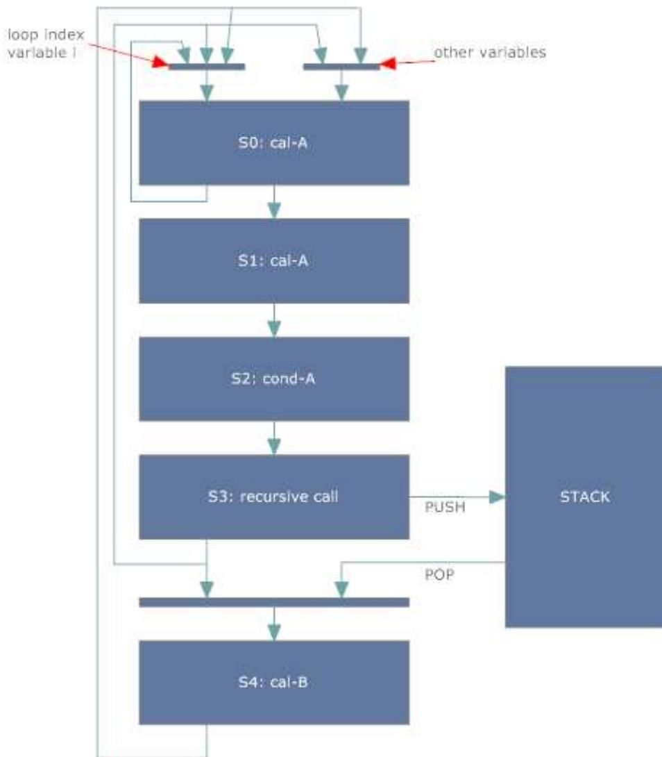
Figure 11 : Speculative execution stage transitions flow diagram
