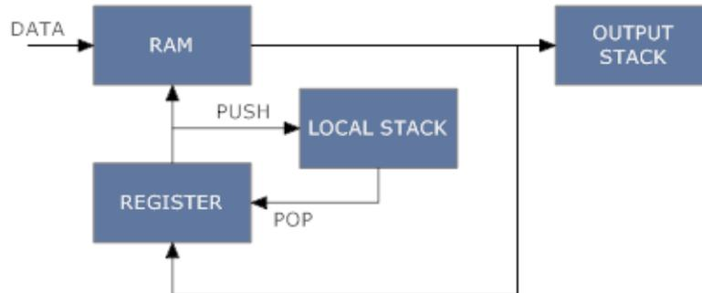
**Figure 21 : Example of an execution unit for a binary tree traversal**
