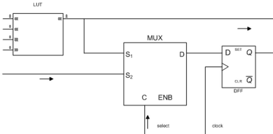
Figure 2 : A basic logic element structure
