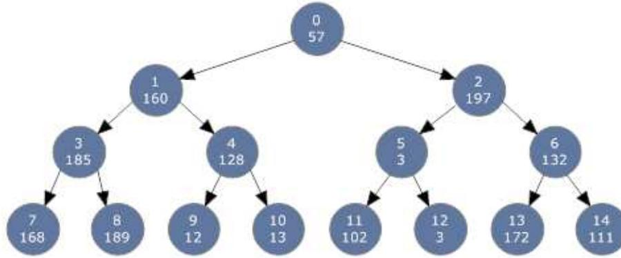
**Figure 41 : A binary tree example for depth 4**
