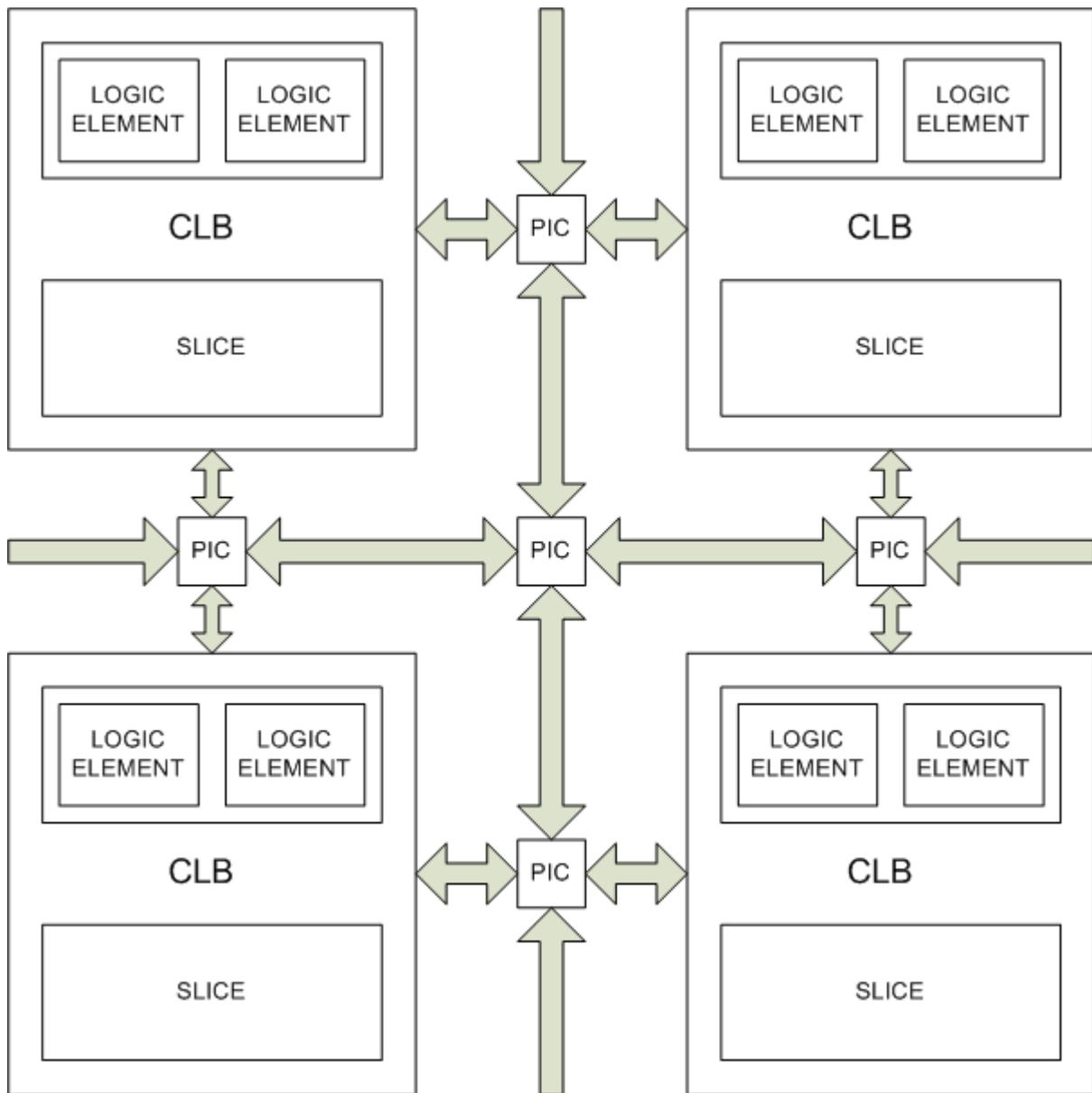
**Figure 4 : Example of an FPGA structure**
