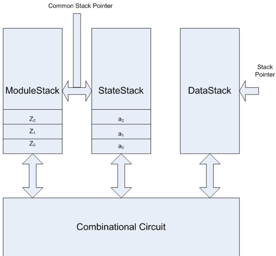
**Figure 16 : General structure of a recursive algorithm implementation**
