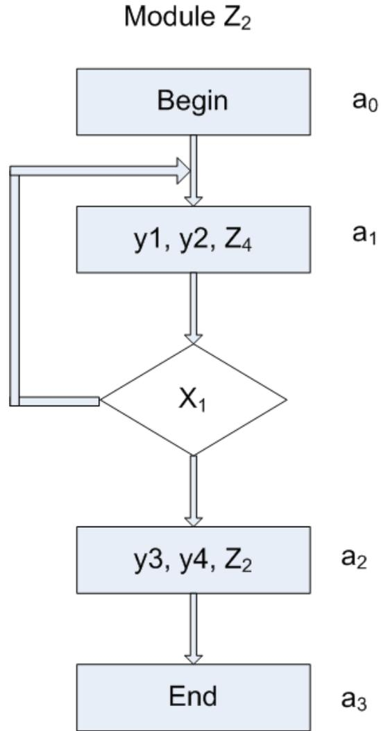
**Figure 18 : Example of  $Z_2$  module with recursion call**
