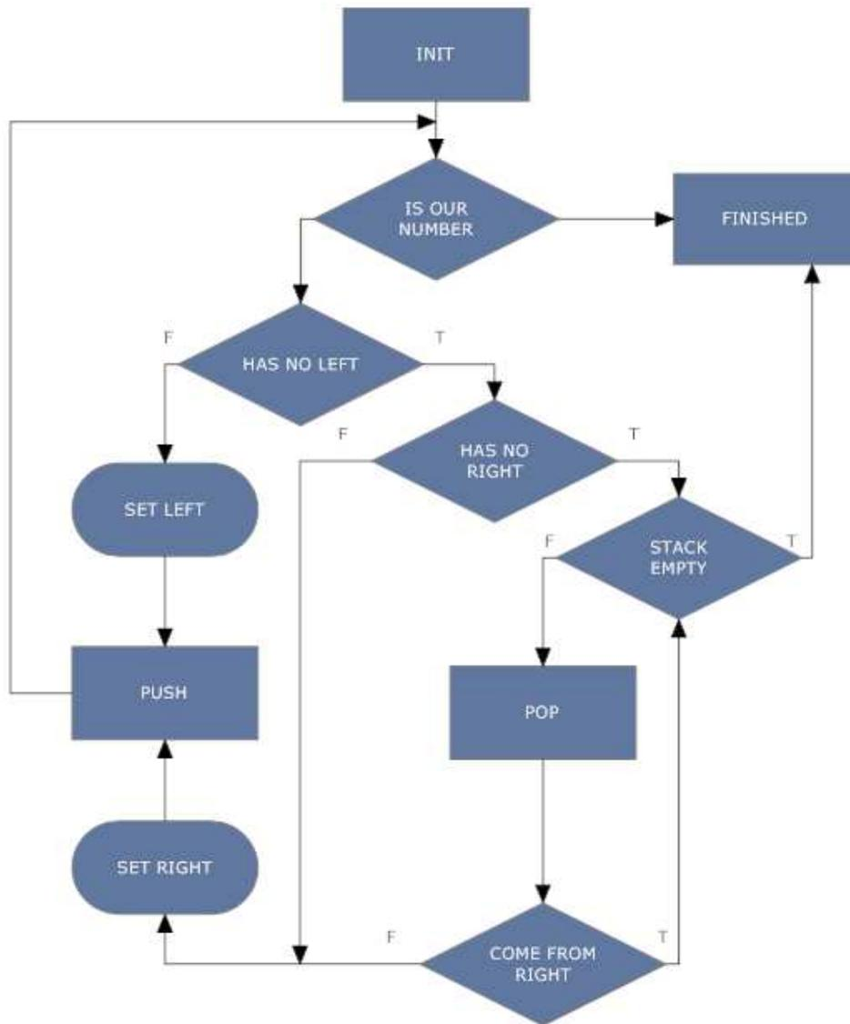
Figure 31 : The ASM of a binary tree traversal algorithm
