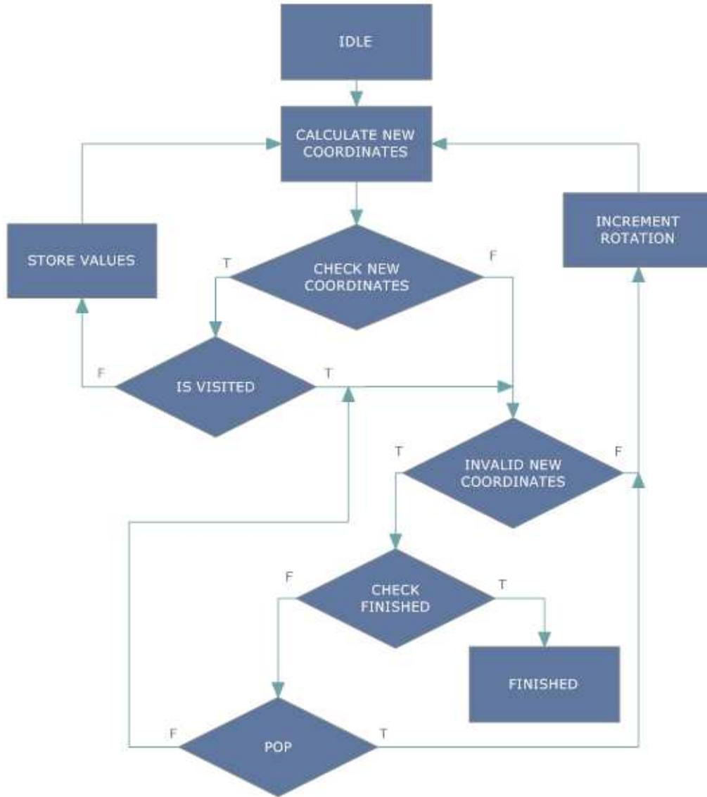
Figure 26 : Knight's tour algorithmic state diagram
