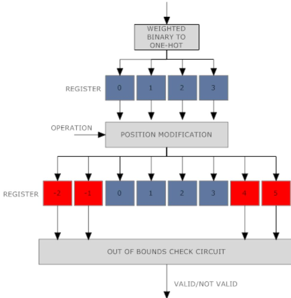
**Figure 32 : Positional comparator substitute circuit**
