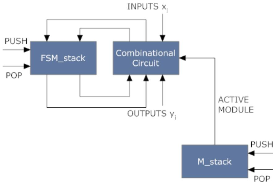
**Figure 20 : Recursive Hierarchical Finite State Machine (RHFSM) basic structure**
