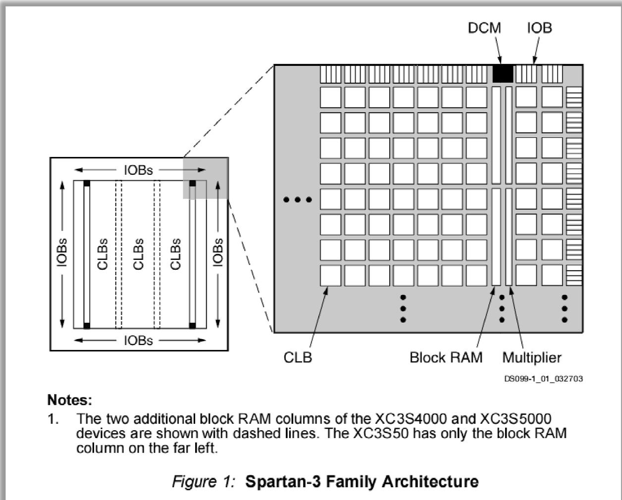
Figure 22 : Spartan 3 structure from [19]
