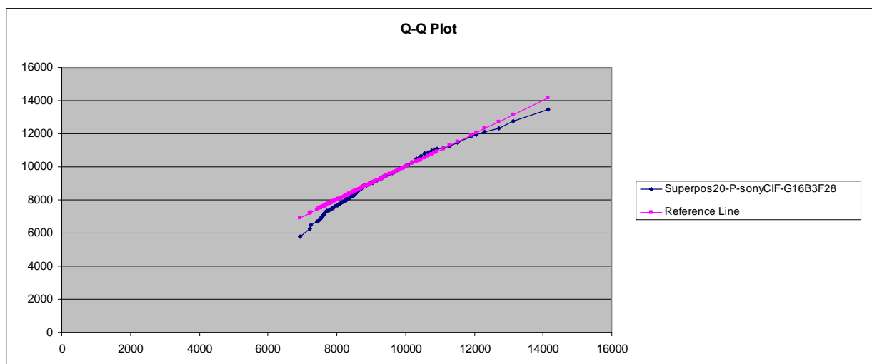
Figure 3. Q-Q plot of the DAR(1) model versus the actual video for the P frames of Sony Demo ([CIF, G16, B3, 28]), for 20 superposed sources. All values are in packets.
