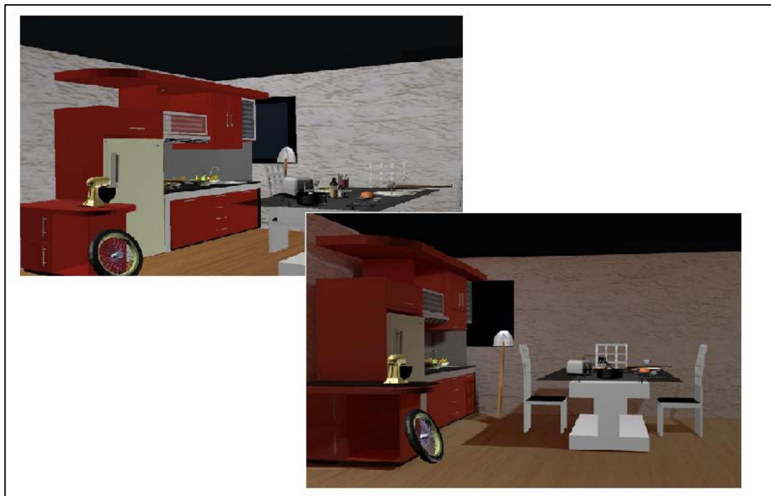
Figure 63: : Left: The kitchen before applying the radiosity solution. Right: The kitchen after applying the radiosity solution. Shadows and simulation of physical energy propagation (right) make the scene more realistic.
