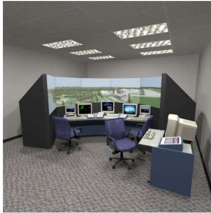
Figure 23: An impression of an ATC tower simulator (using 'rear-projected' LCD), courtesy of Adacel Canada Ltd.
