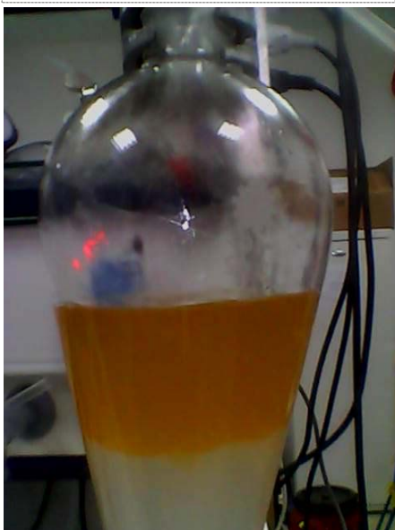
Picture 3: Biodiesel - wash water separation
