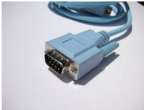
Figure A.4: Serial Cable, typically used for RS-232 serial communication
