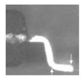
Figure 3.13. A side view of a QFP lead
