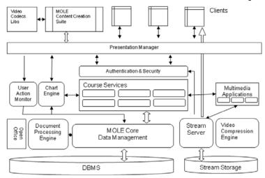
Figure 2 The MOLE internal components
