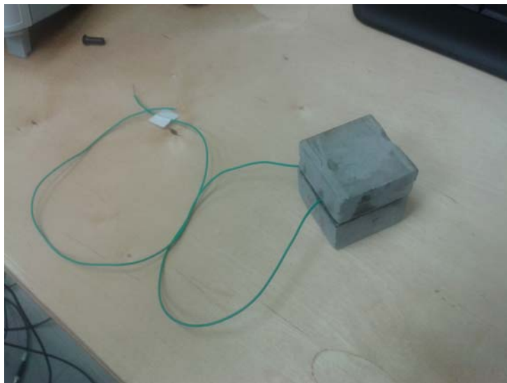
Figure 3: Aggregate-like enclosure for PZT protection
