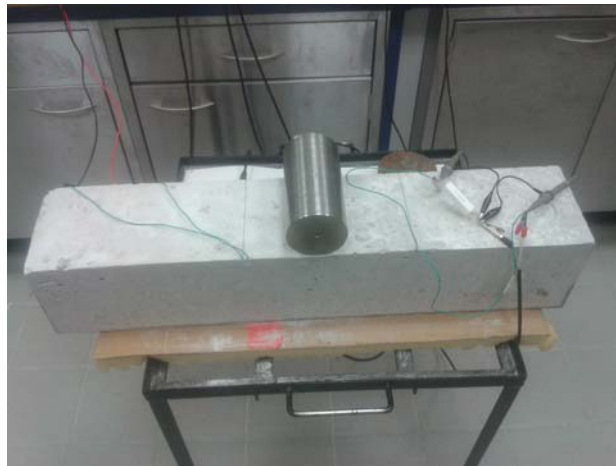
Figure 2: Concrete beam specimen with embedded PZT-based measuring system
