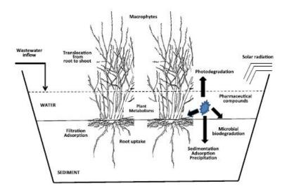
Figure 2. Mechanisms of pharmaceutical removal in CWs (Zhang et al., 2014).
