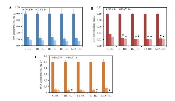
Figure 12. Concentration of BPA (A), CIP (B) and SMX(C) of the different treatments after 0, 14 and 21 days when the high concentration (HC) of contaminants were added (data with asterisk are significantly different (p<0,05) compared to the non-inoculated plants). Bacteria names are described at table 2.
