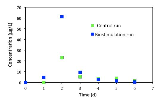
Figure 4. BPA concentration ( $\mu$ g L<sup>-1</sup>) measured in the effluent in the control run (with BPA but no stimulants) and in the biostimulation run where organic acids (oxalic, tartaric, formic, malonic and lactic) were added.
