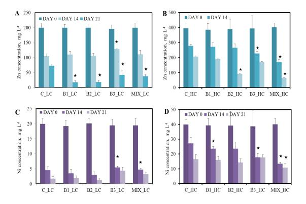
Figure 13. Concentration of Zn (A,B) and Ni (C, D) of the different treatments after 0, 14 and 21 days when the low (A,C) and high (B,D) concentration of contaminants were added (data with asterisk are significantly different (p<0,05) compared to the non-inoculated plants).
