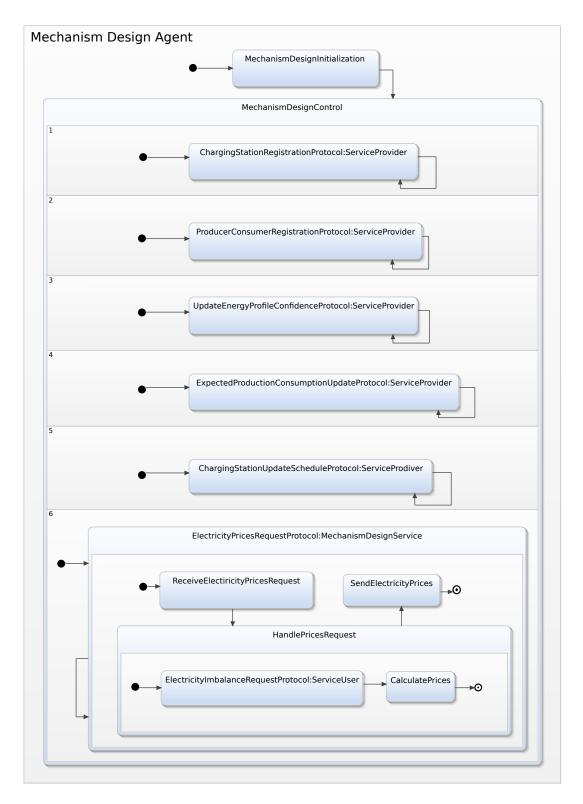
FIGURE 6.19: The intra-agent model of the Mechanism Design agent.
