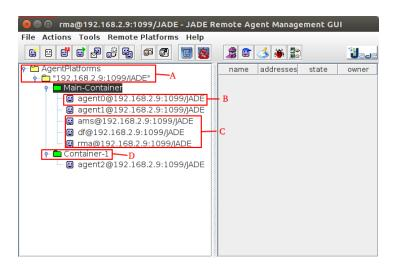
FIGURE 3.7: Example GUI of the JADE RMA showing the basic platform elements.
