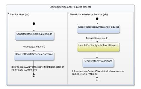
FIGURE 6.8: The model of the Electricity Imbalance Request Protocol.
