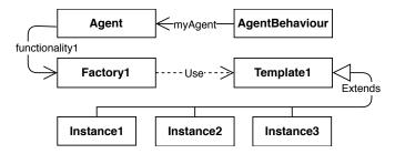
FIGURE 6.23: The abstraction of the Functionality Design Pattern.
