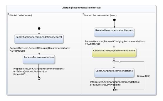
FIGURE 6.1: The model of the Charging Recommendation Protocol.
