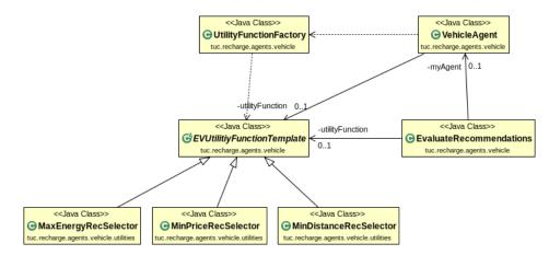
FIGURE 6.14: The impementation of the functionality design pattern for the utility function of the EV agent.
