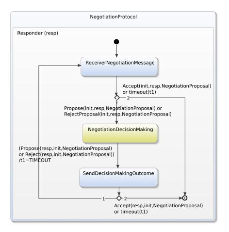
FIGURE 6.3: The model of the Charging Negotiation Protocol.
