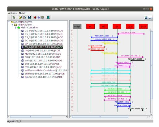
FIGURE 7.9: A screenshot of the JADE sniffer agent that illustrates the communication process of an EV agent that requests charging recommendations and makes a reservation at the selected charging station.
