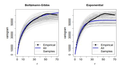
FIG 6. Estimated variograms based on training sets with 400 randomly selected observations (100 repetitions). On both plots, black dots represent the experimental variogram computed with the complete dataset. Blue lines show variograms estimated on the complete dataset, and grey lines correspond to variograms estimated on the 100 training sets, using CL with  $r_0 = 30$  in both cases. Left: Boltzmann-Gibbs variograms. Right: Exponential variograms.
