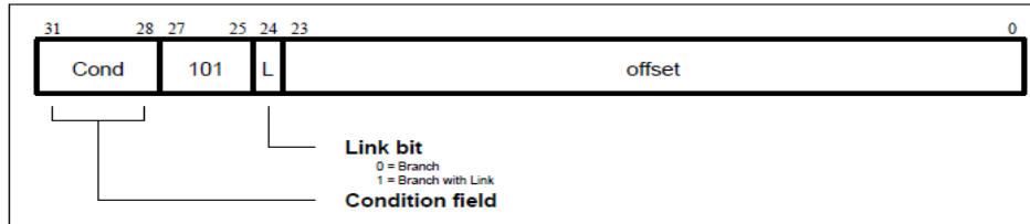
Figure 3. 5: ARM Branch Instructions Encoding
