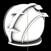
The first ring that surround the Dome is the train ring. The train ring provides quick and easy access to key parts of the dome and connects the working space with the living space.
