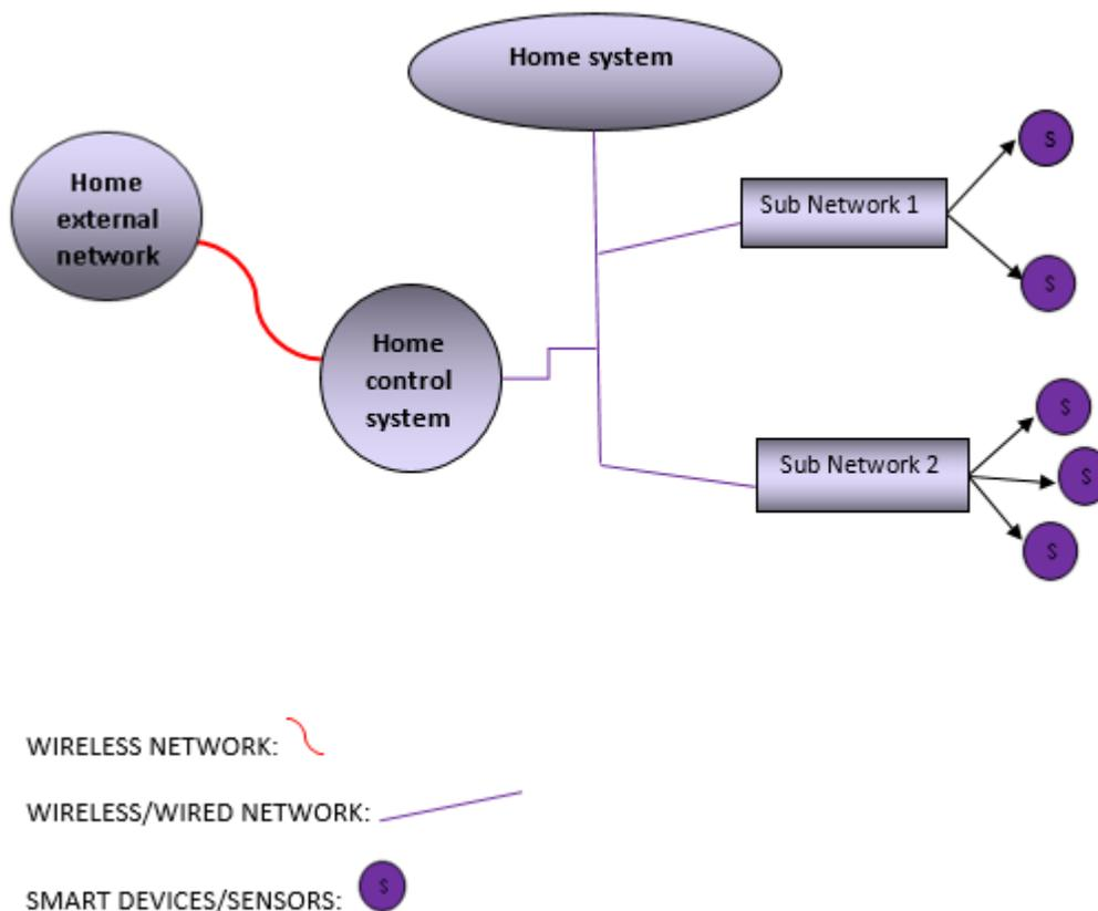
*Figure 1: Basic Structure of a Smart Home System*
