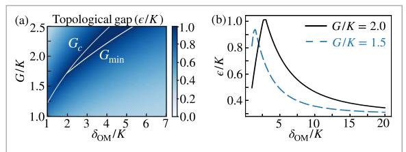
**Figure 3.** Topological gap. (a) Topological gap size  $\epsilon$  as a function of G and the detuning  $\delta_{\mathrm{OM}}$  for J/K=200. The upper white line represents  $G_{\epsilon}$  (see equation (5)) and the bottom one shows the minimal OM coupling  $G_{\min}$  for which  $\epsilon$  reaches K. (b) Gap size as a function of  $\delta_{\mathrm{OM}}$  for G/K=1.5 and G/K=2.0 with J/K=200.
