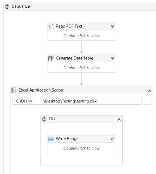
Figure 4: UiPath Process Example
