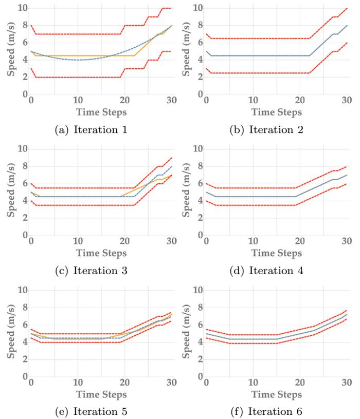
Fig. 2. Received (blue dashed line) and optimal (orange line) speed trajectories of DDDP algorithm in each iteration. The corridor  $\Delta_C^{(l)}$  is marked with red dashed lines.
