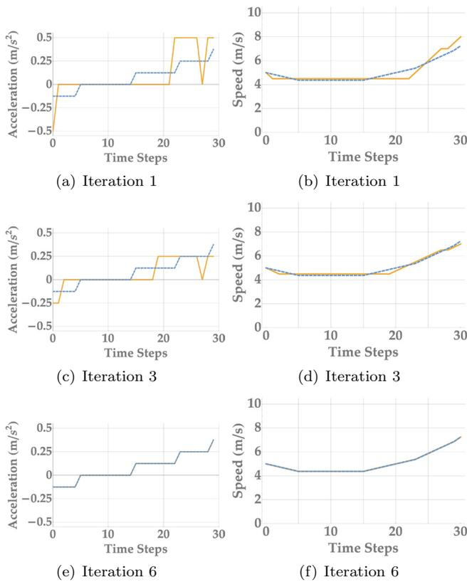
Fig. 3. Optimal acceleration and speed trajectories (orange line) of three DDDP iterations, compared with corresponding optimal trajectories of the one-shot SDP (blue dashed line).
