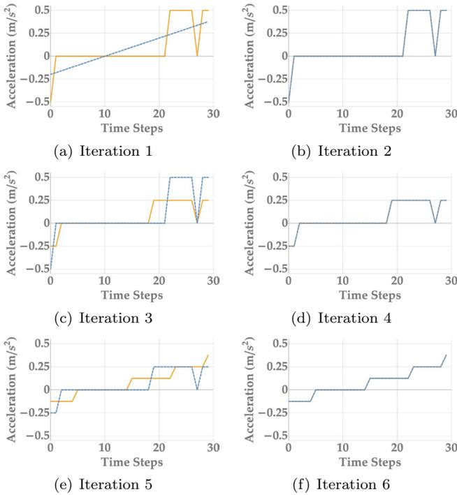
Fig. 1. Received (blue dashed line) and optimal (orange line) acceleration trajectories of DDDP algorithm in each iteration.
