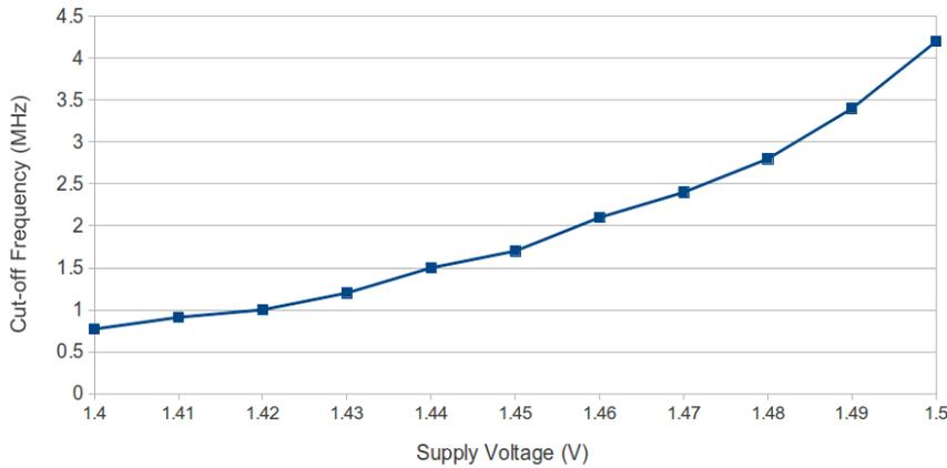
Figure 5.6: Gm-C filter tunability in relation to (Driver) supply voltage.
