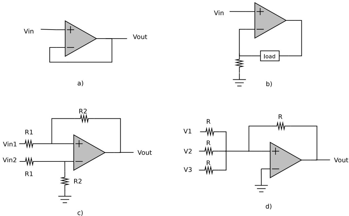
Figure 3.3: OpAmp Typical Networks: a) Follower. b) Current Source. c) Differential Amplifier. d) Summing Amplifier
