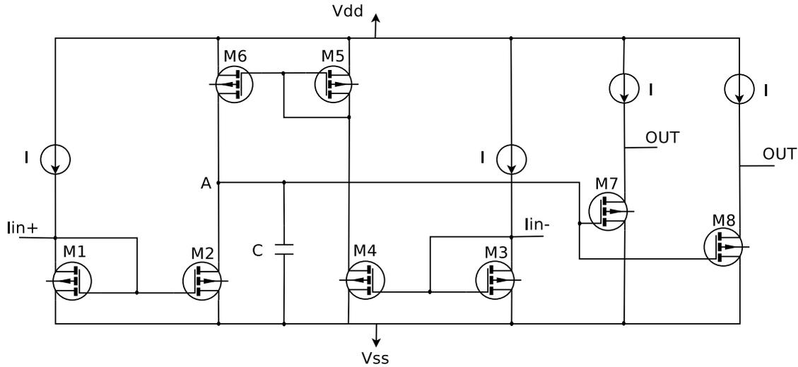
Figure 4.19: Detail schematic of the current mode OpAmp
