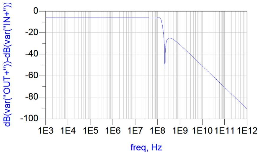
Figure 4.2: The Passive 3rd order 150 MHz low-pass elliptical filter frequency response
