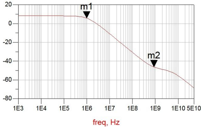
Figure 4.14: Frequency response for the redesigned filter with the driver amplifier in 1.42 supply voltage. The cut-off point is at 5.2db and 986.4KHz
