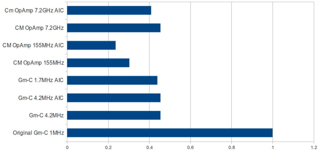
Figure 5.1: Voltage Supply of filters normalized to the supply of the original 1MHz filter(AIC - After IC analysis).
