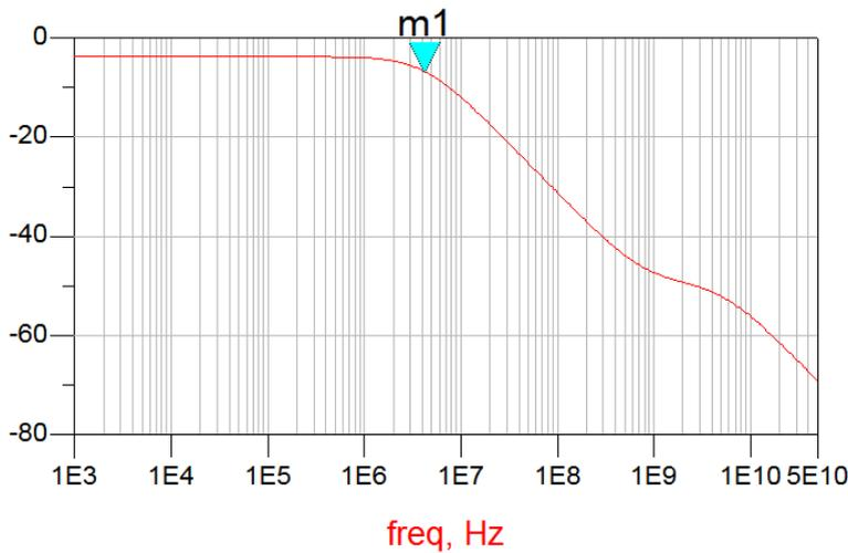
Figure 4.15: Frequency response for the redesigned filter with the driver amplifier in 1.5 supply voltage. The cut-off point is at -6.8db (similar to the original design) and 4.2MHz
