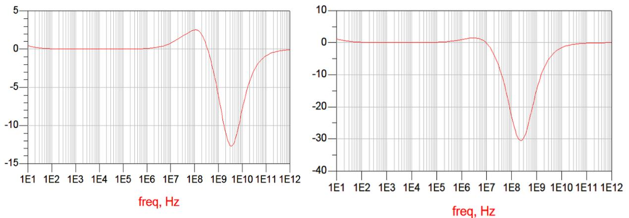
Figure 5.3: Phase Response for initial CM OpAmp 7.2GHz and 155MHz filters. Cut-off points at -9.9 and -28.4 degrees respectively.
