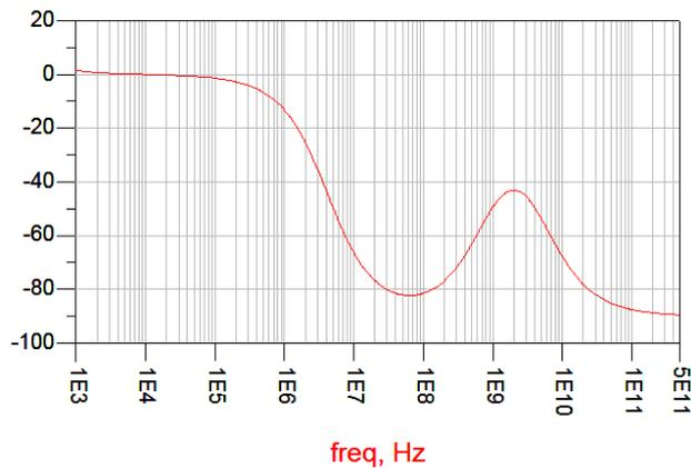
Figure 5.2: Phase Response for the first 4.2MHz Gm-C filter. Cut-off point at -44.6 degrees.
