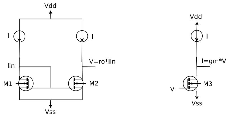
Figure 4.18: I-V conversion with simple current mirror and V-I conversion with simple current source
