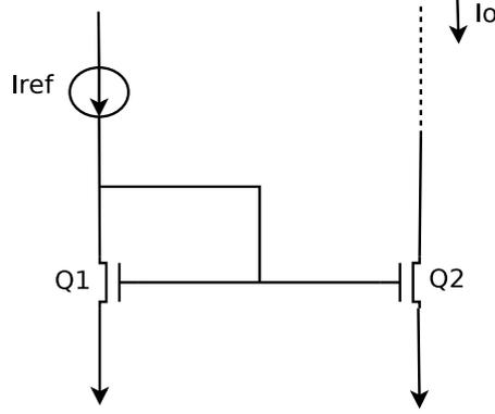
Figure 3.9: The Simple Current Mirror
