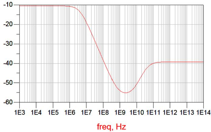
Figure 4.26: 4.2MHz Gm-C frequency response after IC analysis filter. -3db point at -13.5db at 4.2 MHz frequency point.
