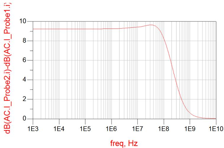
Figure 4.28: 155MHz CM filter frequency response for the updated aspect ratios. -3db point at 6.6db at 154.9 MHz frequency point.
