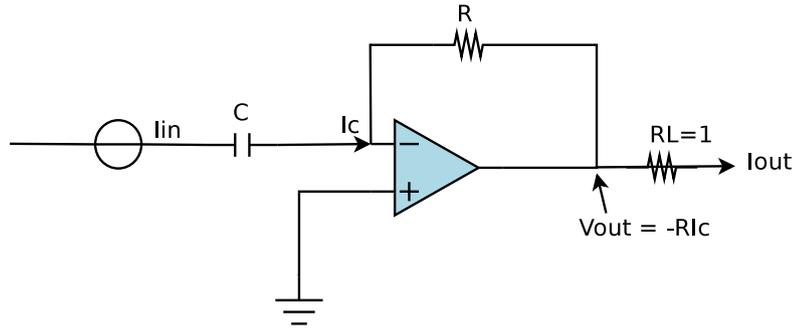
Figure 4.16: Differentiator topology working inter-reciprocal to the voltage mode integrator
