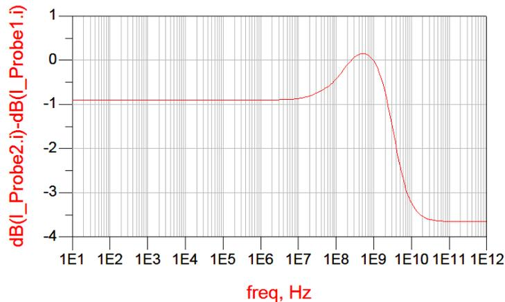
Figure 4.24: 7.2GHz CM filter frequency response. -3db point at -2.92db at 7.197GHz frequency point.
