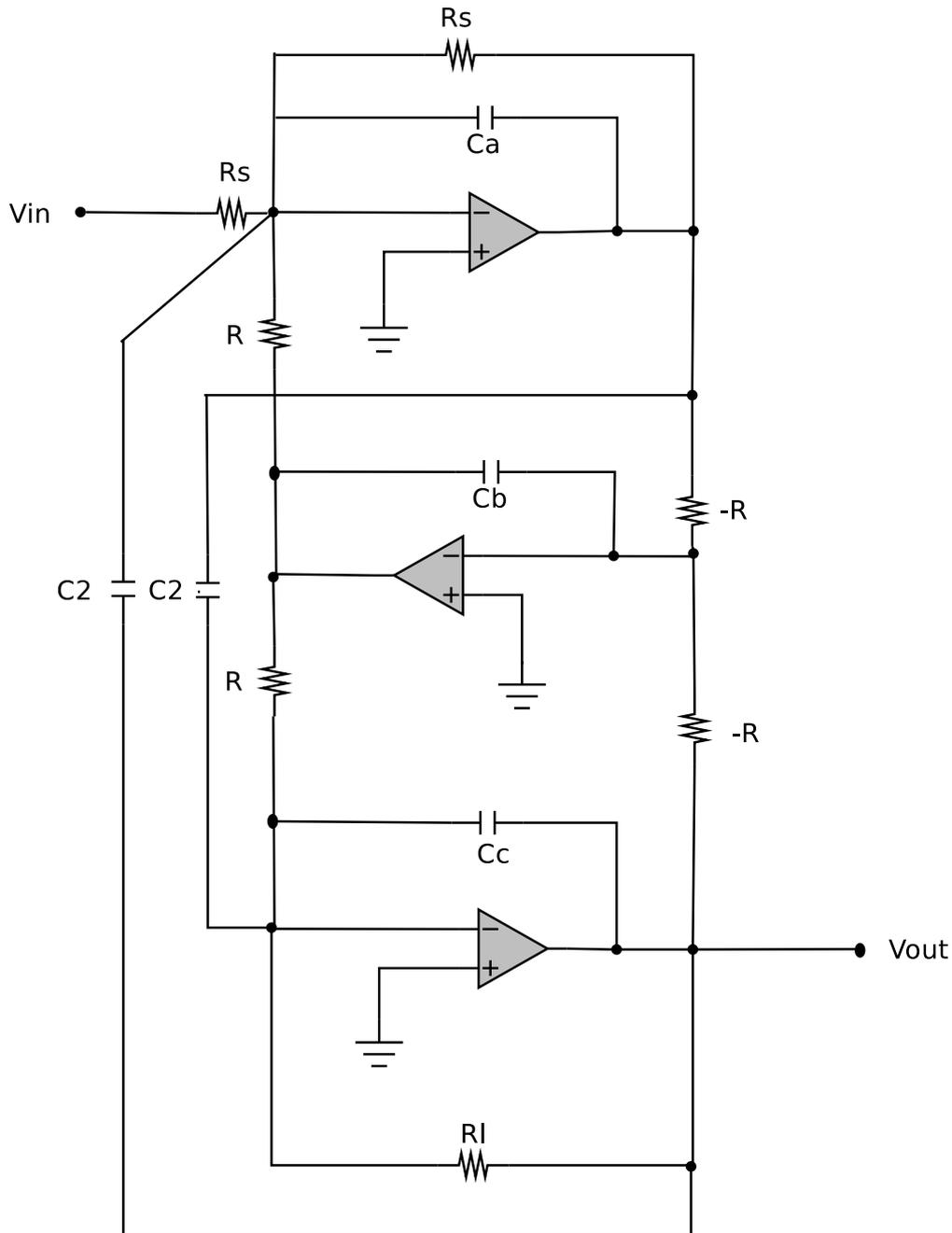
Figure 4.4: The active RC implementation of the elliptical filter, using OpAmps
