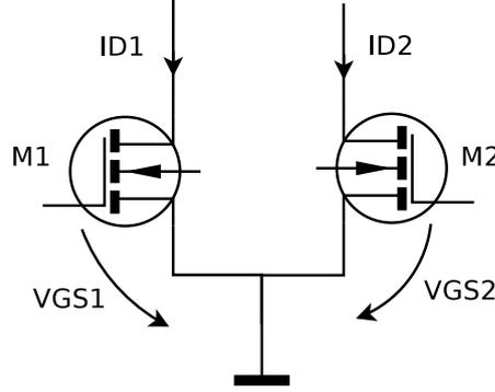
Figure 4.6: MOSFET pair presenting the Drain Current Difference linearization principle.
