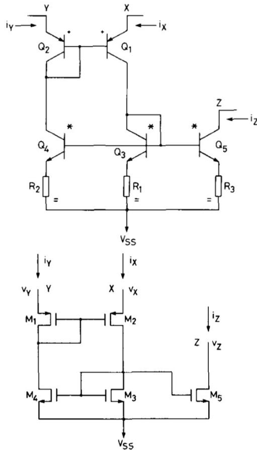
Figure 1.2: The first Current Conveyors in bipolar and MOS transistor implementations [23]
