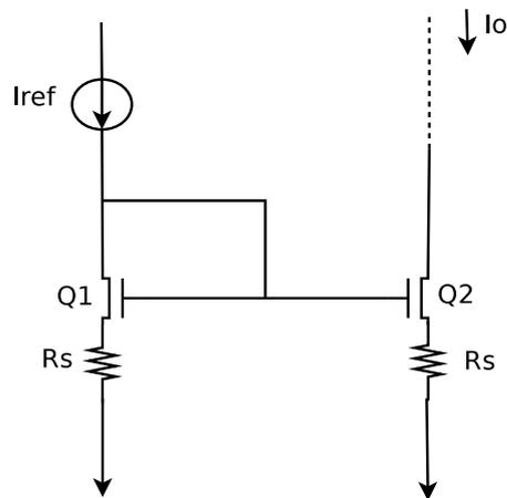
Figure 3.10: Source Degenerate Current Mirror
