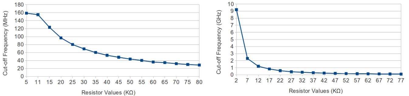
Figure 5.7: CM OpAmp filters' tunability in relation to differentiator resistor values.
