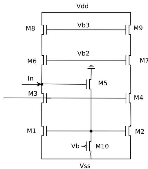
Figure 2.3: Current Amplifier used for integrator design in [16]
