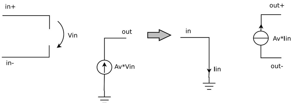
Figure 1.4: Voltage mode and Current Mode operational Amplifiers functionality
