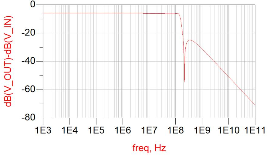
Figure 4.5: The active RC 3rd order 150 MHz low-pass elliptical filter frequency response
