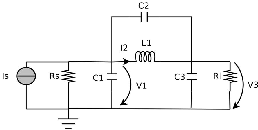
Figure 4.1: The Passive 3rd order low-pass elliptical filter
