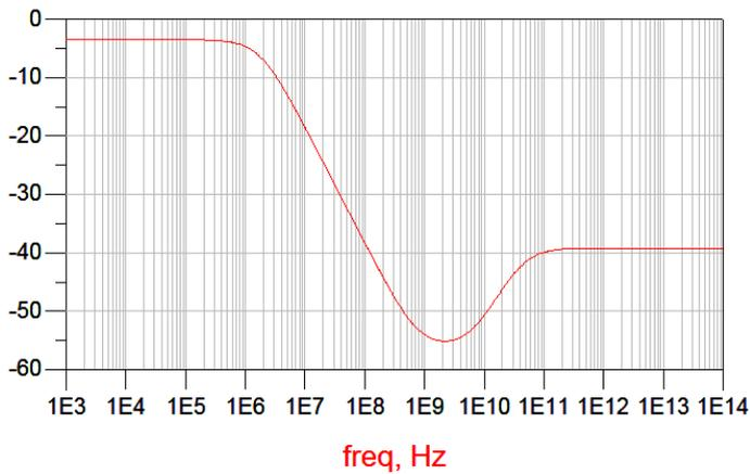
Figure 4.27: 1.7MHz Gm-C frequency response after IC analysis filter. -3db point at -6.4db at 1.76 MHz frequency point.
