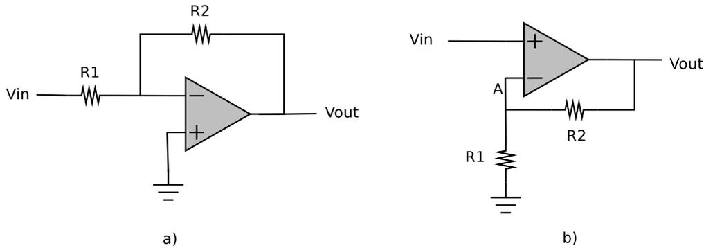
Figure 3.2: The inverting and non-inverting amplifier
