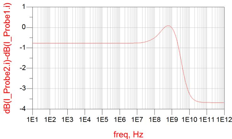
Figure 4.29: 7.2GHz CM filter frequency response for the updated aspect ratios. -3db point at -2.93db at 7.21 frequency point.
