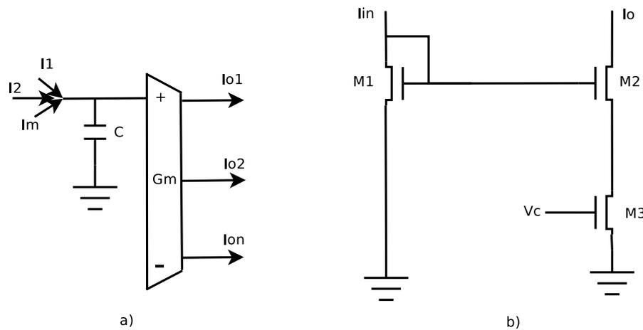
Figure 2.2: Circuits examples presented in [20].a)Current transconductance integrator.
