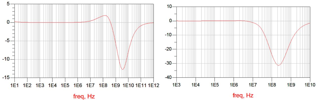
Figure 5.5: Phase Response for CM OpAmp 7.2GHz and 155MHz filters after IC analysis.Cut-off points at -10.1 and -29.5 degrees respectively.
