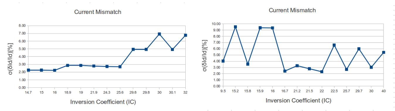
Figure 5.9: CM OpAmp filters' Current Mismatch for its current mirrors. The mismatch for the 155MHz and 7.2GHz filters are shown here respectively.
