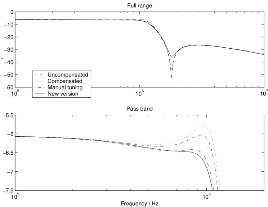
Figure 4.13: The 1.2um filter frequency response[14]
