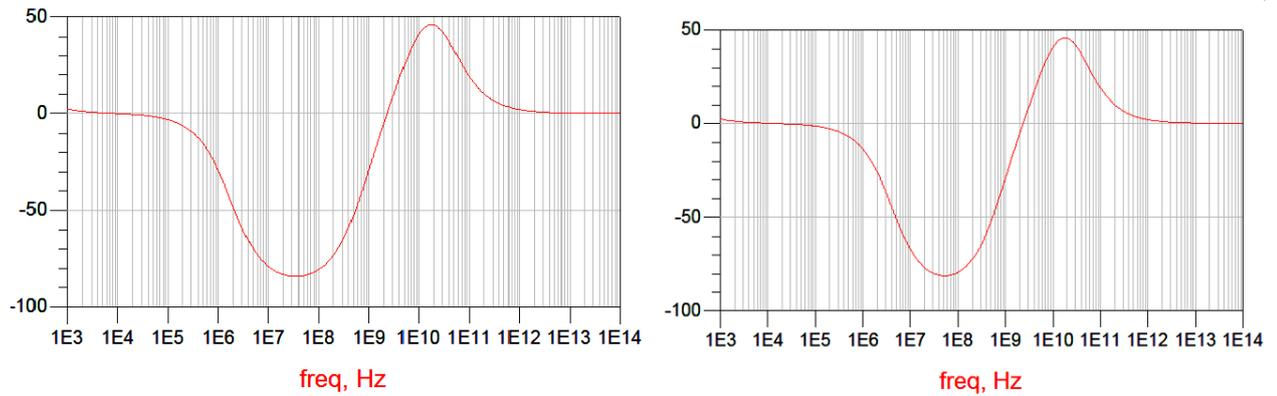
Figure 5.4: Phase Response for 1.7MHz and 4.2MHz Gm-C filters after IC analysis..Cut-off points at -44.6 and -45 degrees respectively.
