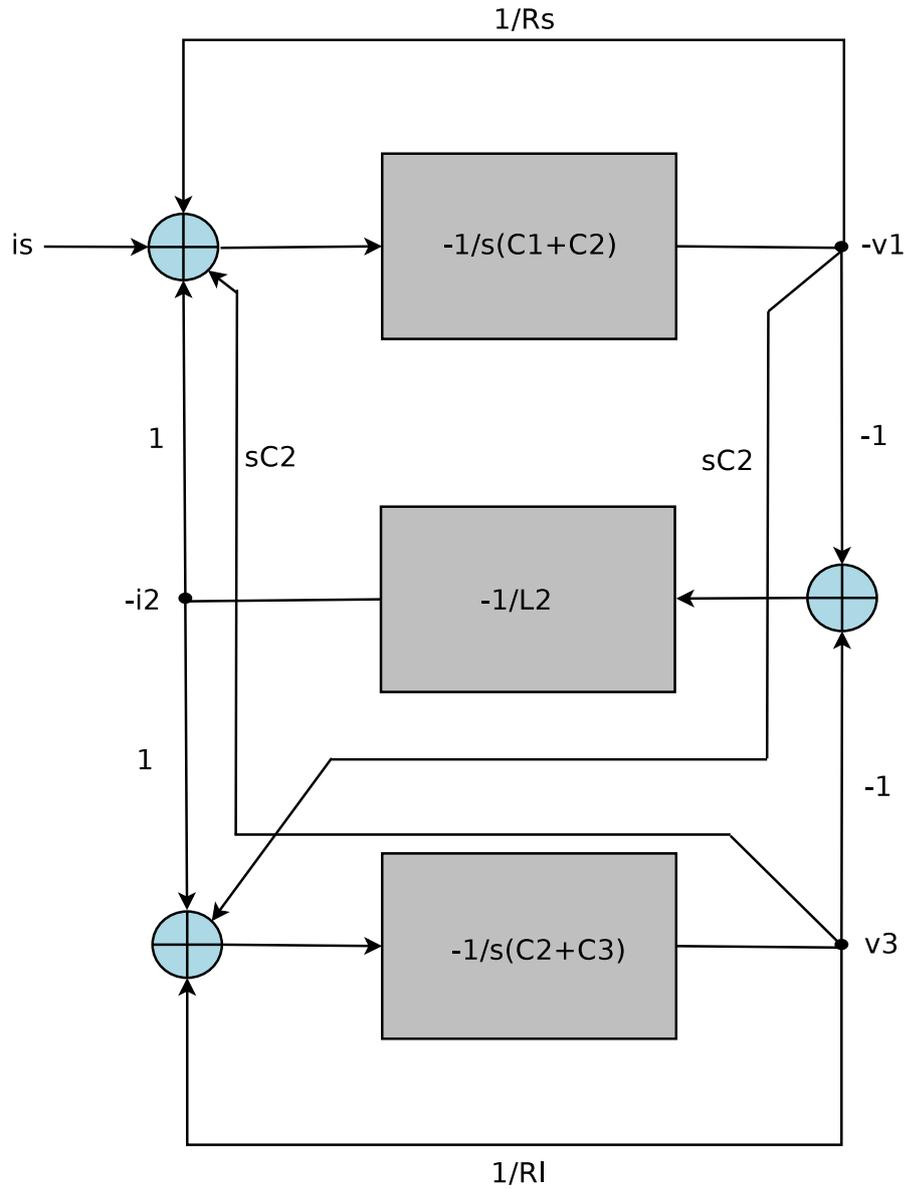
Figure 4.3: The filter Block Diagram as derived by KVL and KCL.
