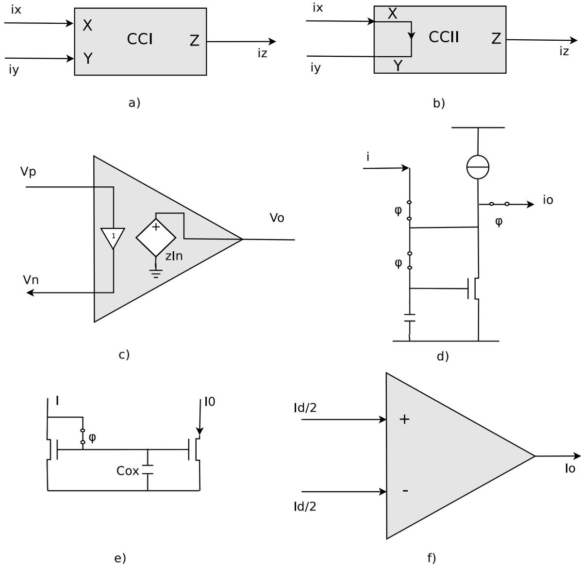
Figure 2.1: Current Mode Device Examples. a) Current Conveyor. b) 2nd generation Current Conveyor. c) Current Feedback Operational Amplifier. d) Switched Current memory cell. e) 2nd generation switch current, current store f) Current mode OpAmp.
