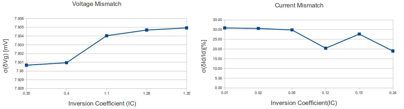
Figure 5.8: 1.7MHz Gm-C filter Current Mismatch for current mirrors and Voltage Mismatch for the differential pairs in the transconductor.
