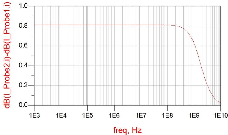
Figure 4.22: Current mode differentiator frequency response
