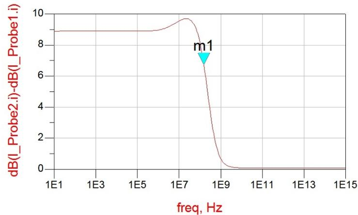
Figure 4.23: 155MHz CM filter frequency response. -3db point at 6.7db at 155.1 MHz frequency point.
