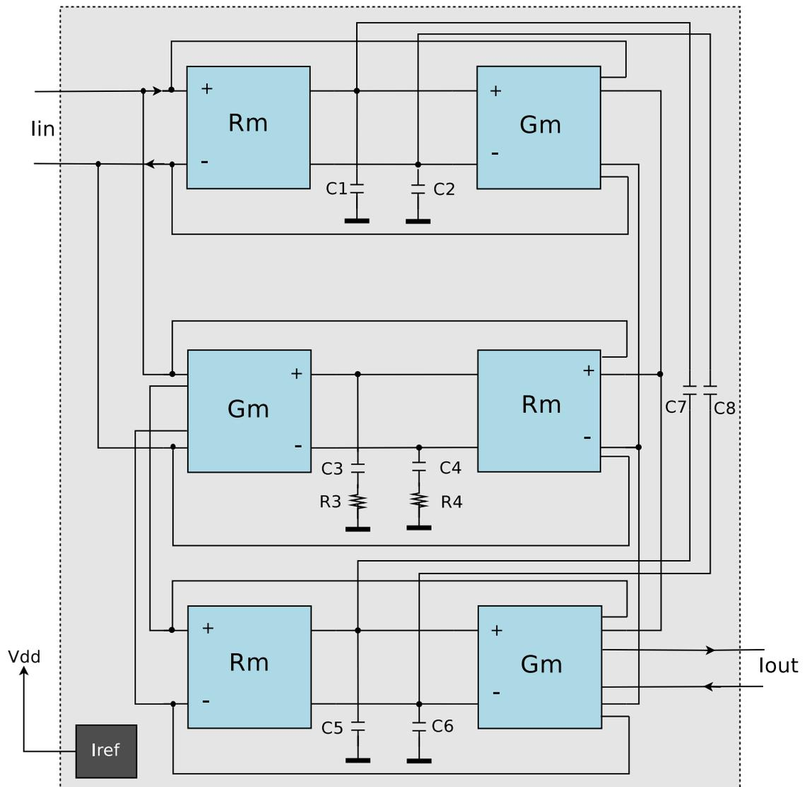
Figure 4.11: Gm current mode filter block diagram.
