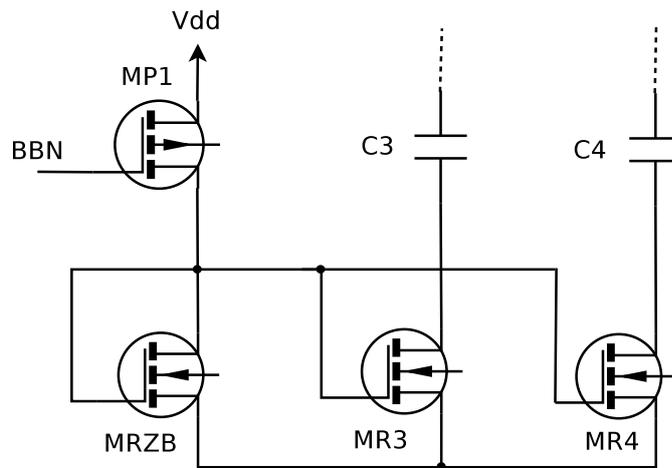
Figure 4.12: NMOS resistor circuit.
