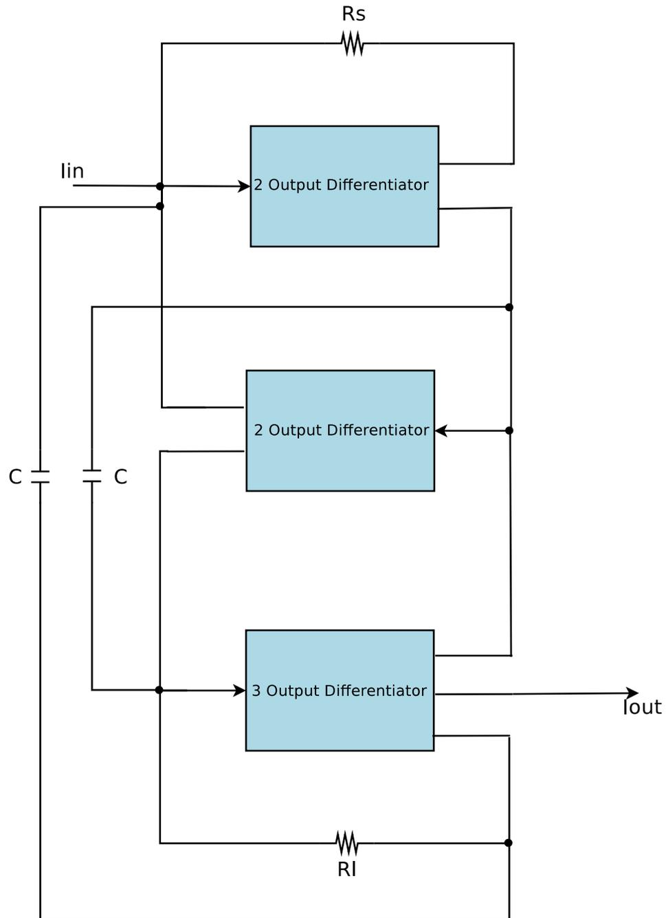
Figure 4.20: Filter block diagram for the current mode operational amplifier implementation
