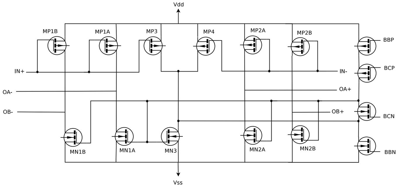
Figure 4.7: Linearized Transconductor implemented for the current mode Integrator design.
