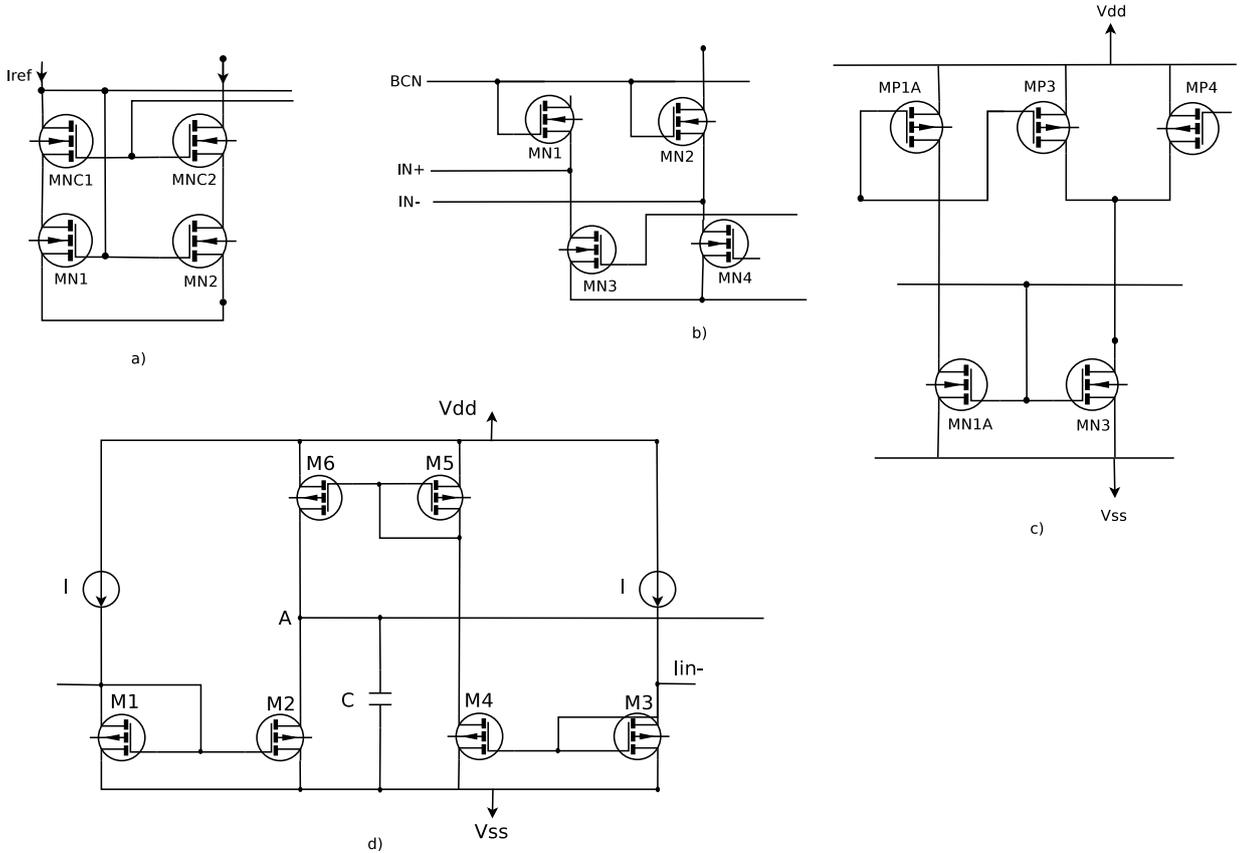
Figure 4.25: Circuit parts included to the IC analysis. a) Current reference b) Driver c) Transconductor d) CM OpAmp
