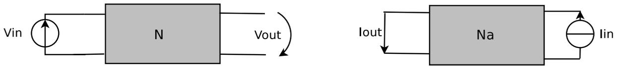
Figure 3.12: Network conversion according to the adjoint principle
