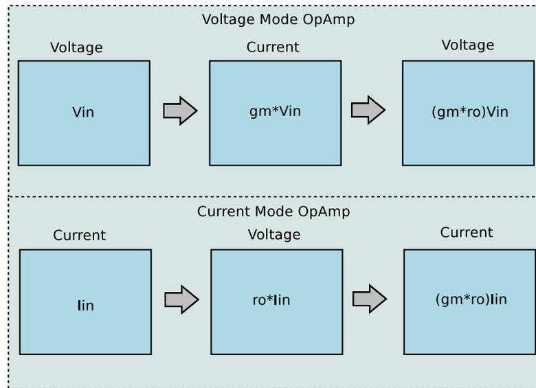
Figure 4.17: Signal Flow in voltage and current mode OpAmp
