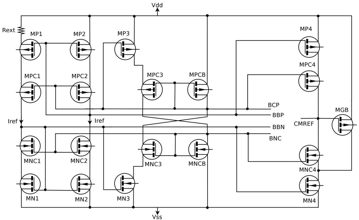
Figure 4.9: The current reference circuit.
