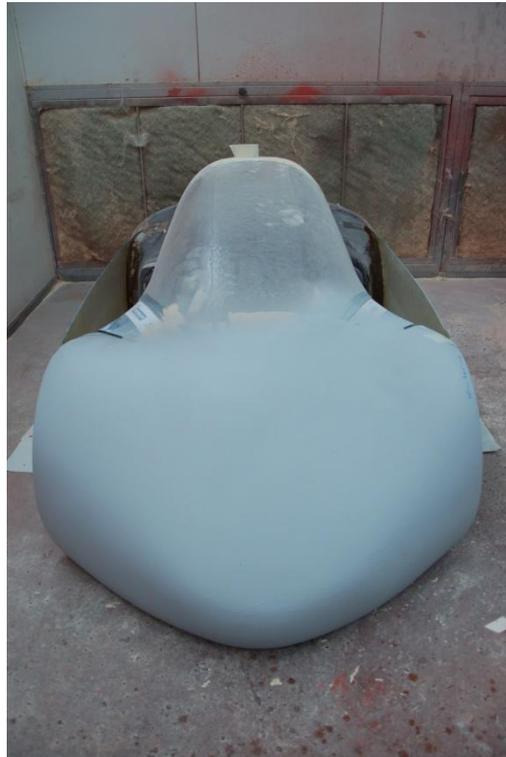
Figure 7.1: Using the old vehicle to construct the initial mockup
