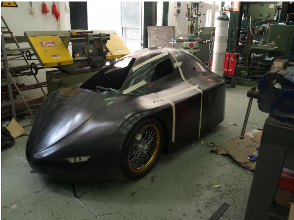
Figure 7.6: The final carbon-fiber surface of ER12 (4th model)
