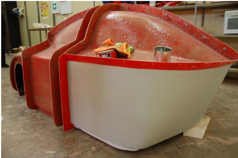
**Figure 7.4: The rear side of the female-mold**
