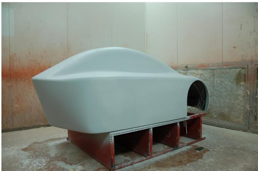
Figure 7.2: The Final male-mold
