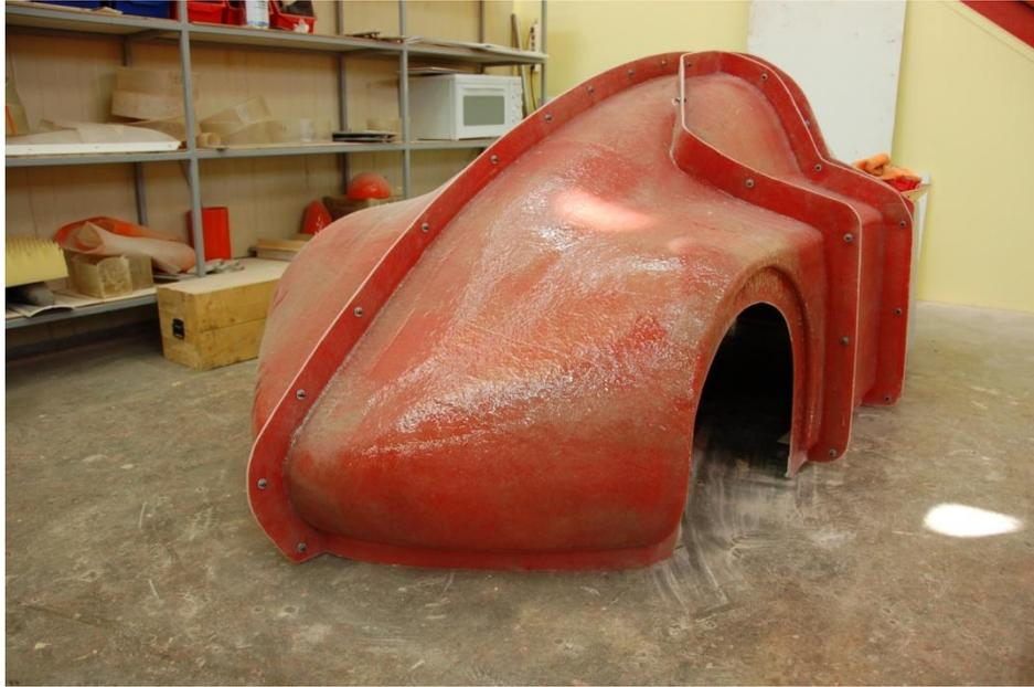
**Figure 7.3: The constructed female-mold**
