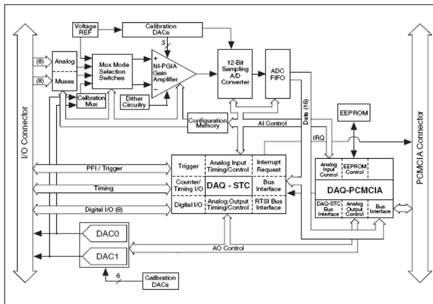
Figure 45 -Block diagram of 6024E
