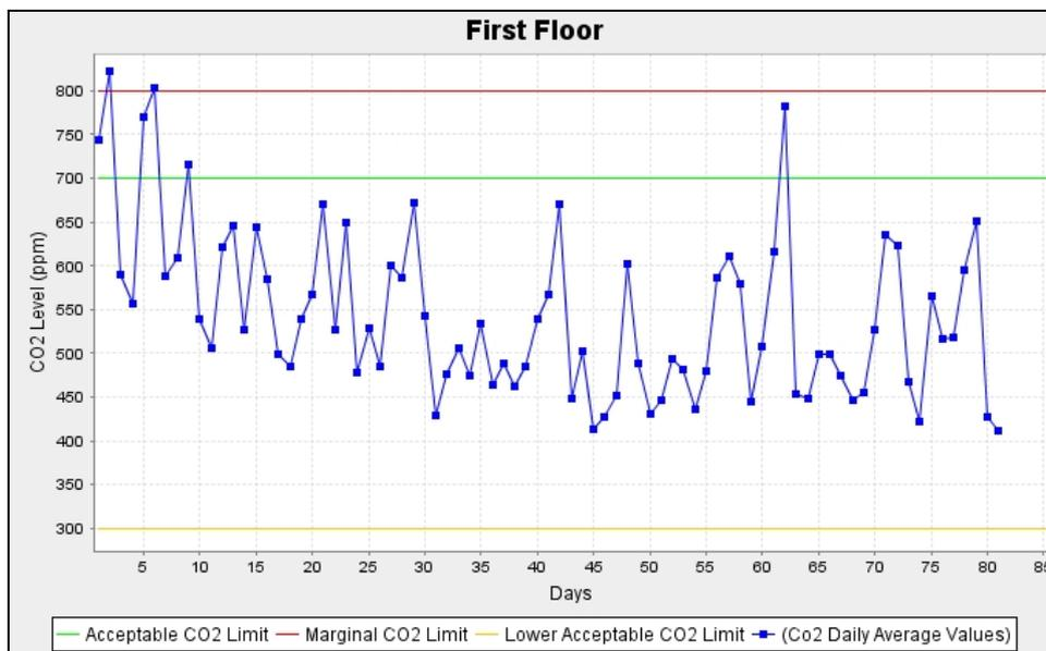
Figure 23 - Carbon Dioxide Classification chart for Zone B – First Floor
