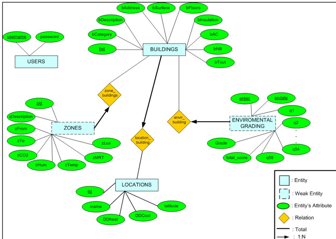
Figure 8 - Database Entity Relationship diagram
