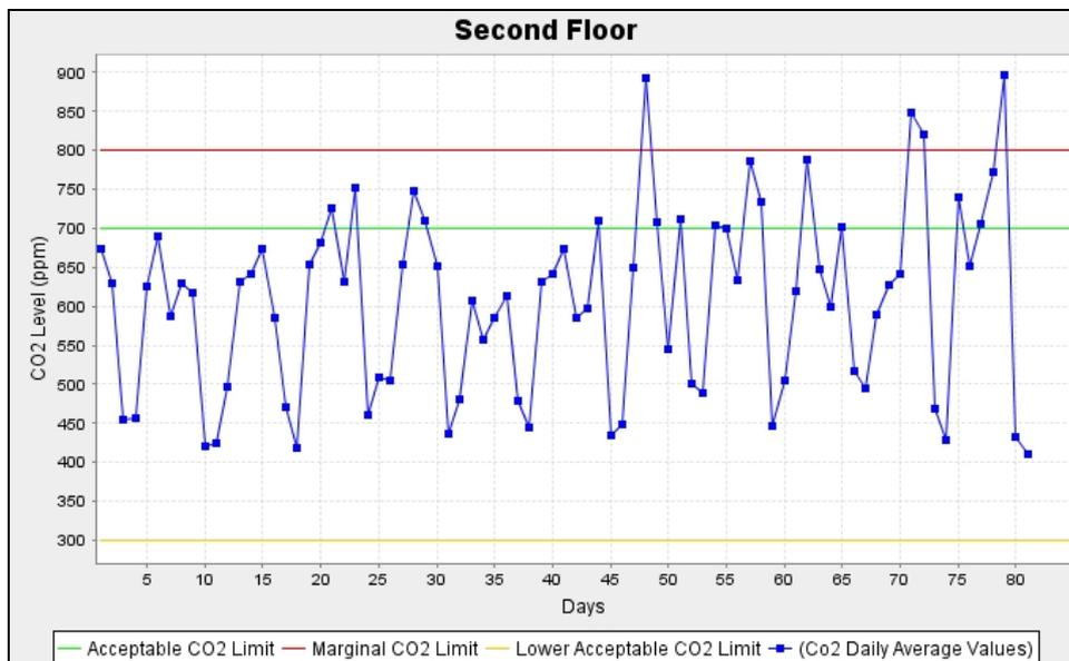
Figure 25 - Carbon Dioxide Classification chart for Zone C – Second Floor
