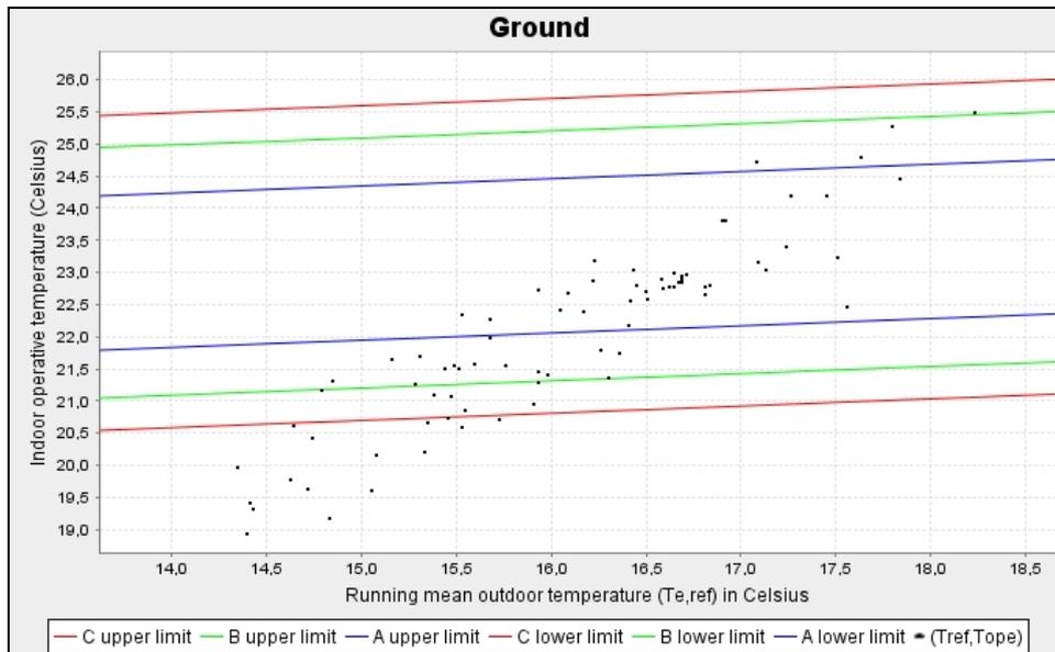
Figure 9 - Thermal Comfort Classification chart for Zone A – Ground Floor
