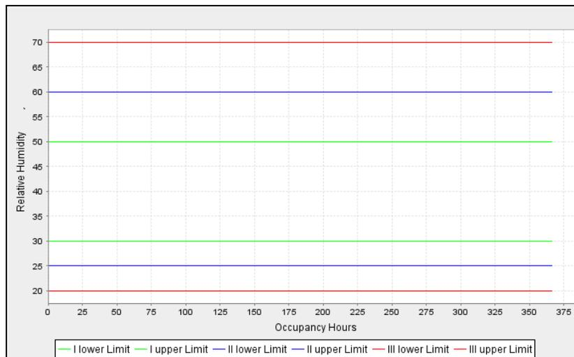
Figure 5 – Relative humidity classification limit lines
