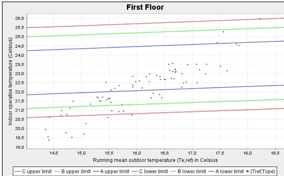
Figure 11 - Thermal Comfort Classification chart for Zone B – First Floor
