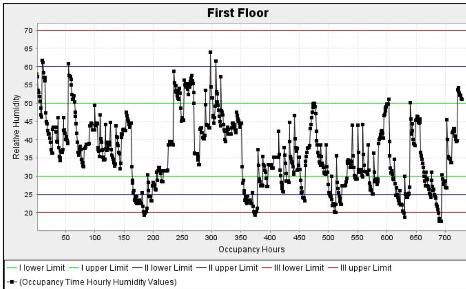
Figure 17 - Relative humidity Classification chart for Zone B – First Floor
