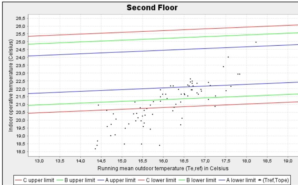
Figure 13 - Thermal Comfort Classification chart for Zone C – Second Floor
