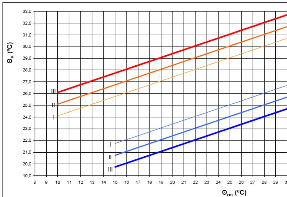
Figure 1 - Design values for the indoor operative temperature for buildings without mechanical cooling systems as a function of the exponentially-weighted running mean of the outdoor temperature.
