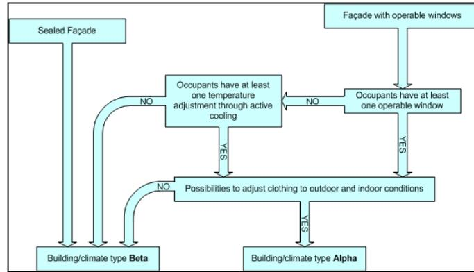
Figure 2 - Diagram determining the type of building/climate
