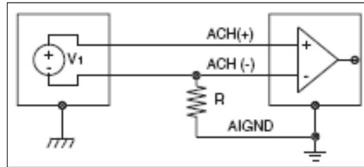
Figure 47 - Differential Connection between sensor and 6024E
