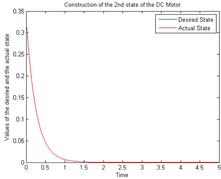
Figure 8.2: Evolution of the Angular Velocity of the DC Motor System
