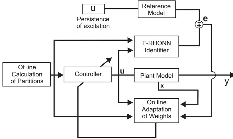
Figure 3.1: Overall scheme of the indirect adaptive neuro-fuzzy control system [54]
