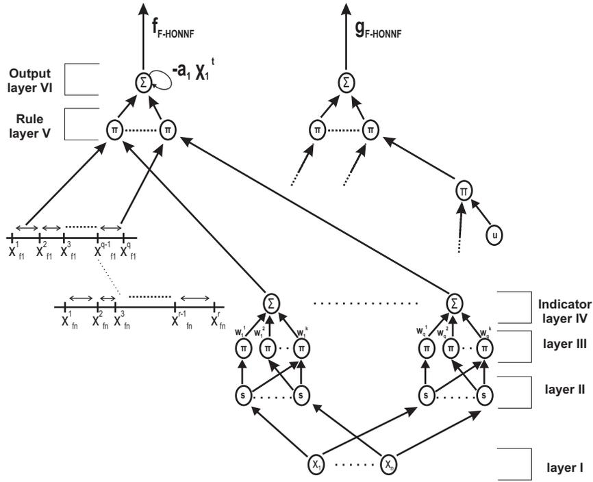
Figure 7.1: Overall scheme of indirect adaptive neuro-fuzzy approximator [54]
