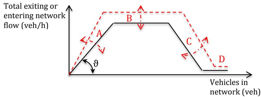
Figure 2-5: The fundamental diagram.
