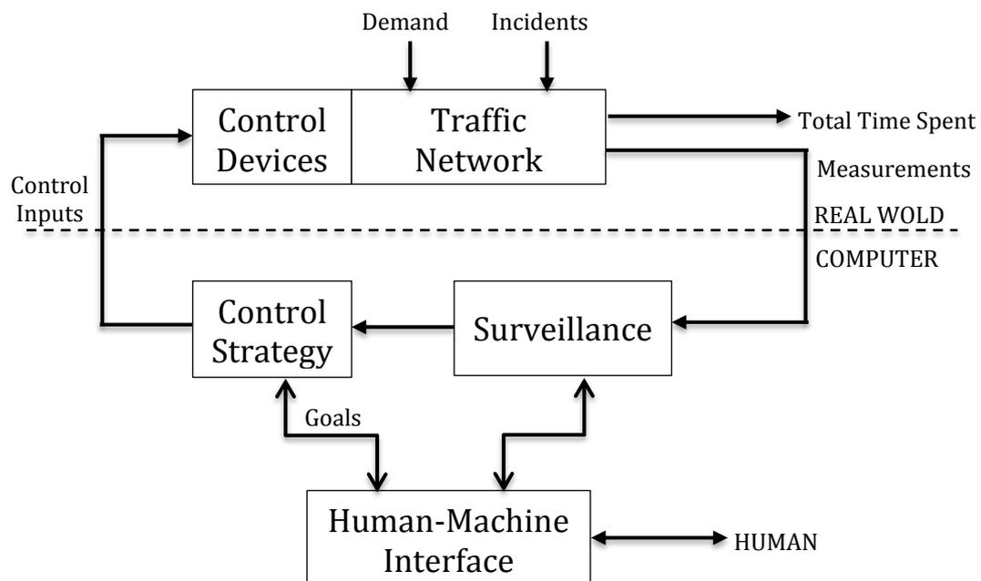
Figure 2-1: The control loop.
