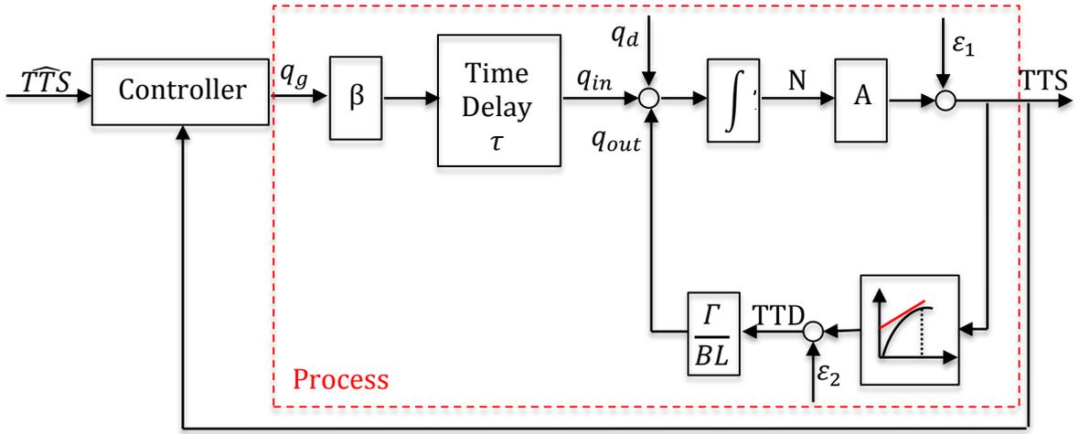
Figure 3-2: Feedback process for gating.
