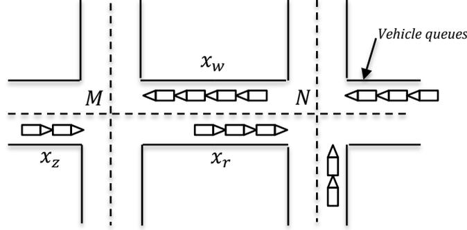
Figure 4-2: A two-way link connecting two junctions M and N
