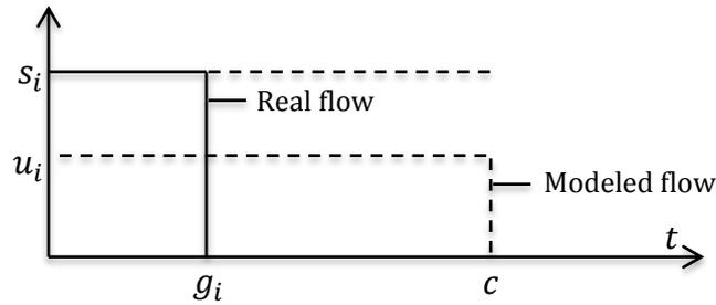
Figure 2-4: Simplified modeling of link outflow  $u_i$ .
