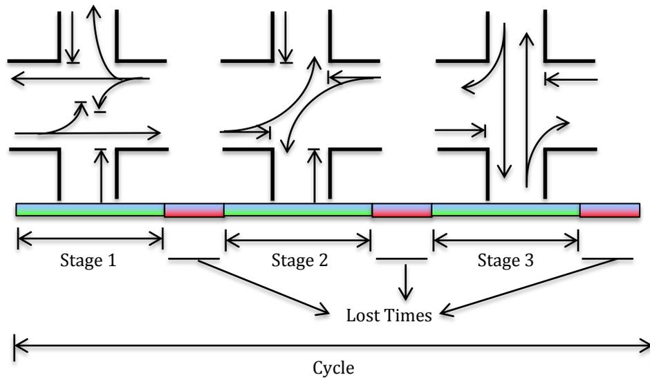
Figure 2-3: Example of signal cycle.
