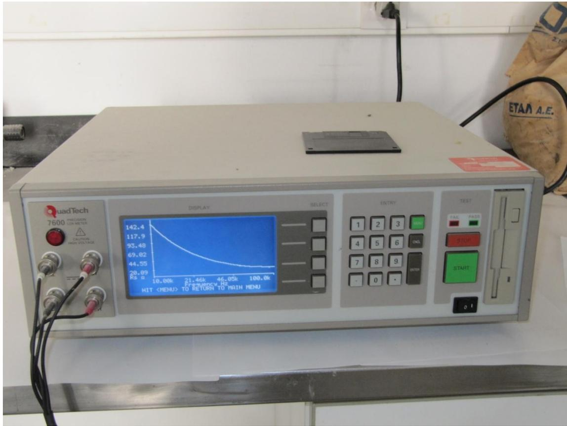
Picture 6.5 Quadtech 7600 Precision LCR meter
