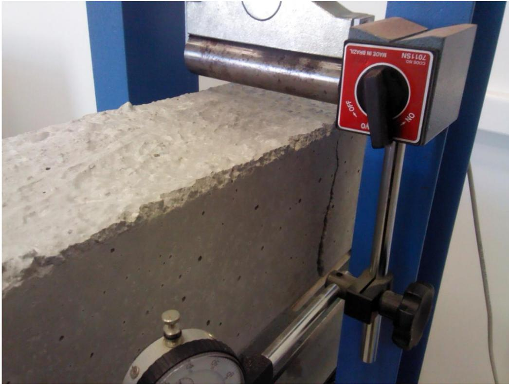
Picture 9.16 Crack occurred for load 6
