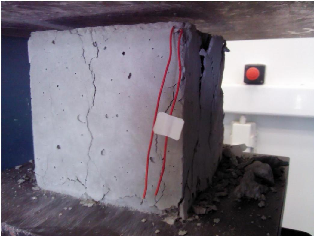
Picture 9.10 – Cycle load 16 (Failure)
