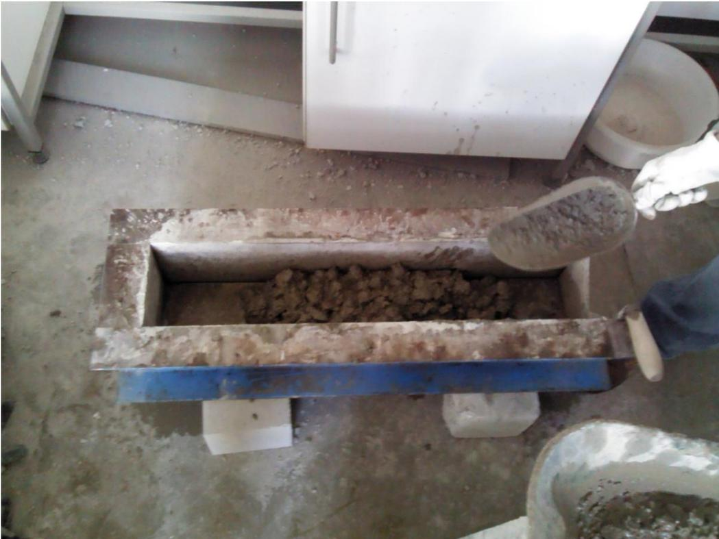
Picture 8.6 Creation of the beam specimen
