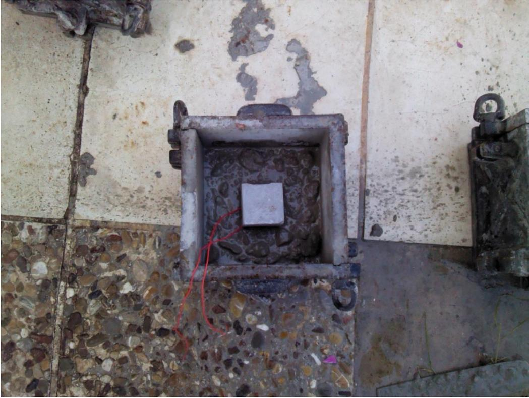
Picture 8.3 Smart aggregate inside the cubic specimen
