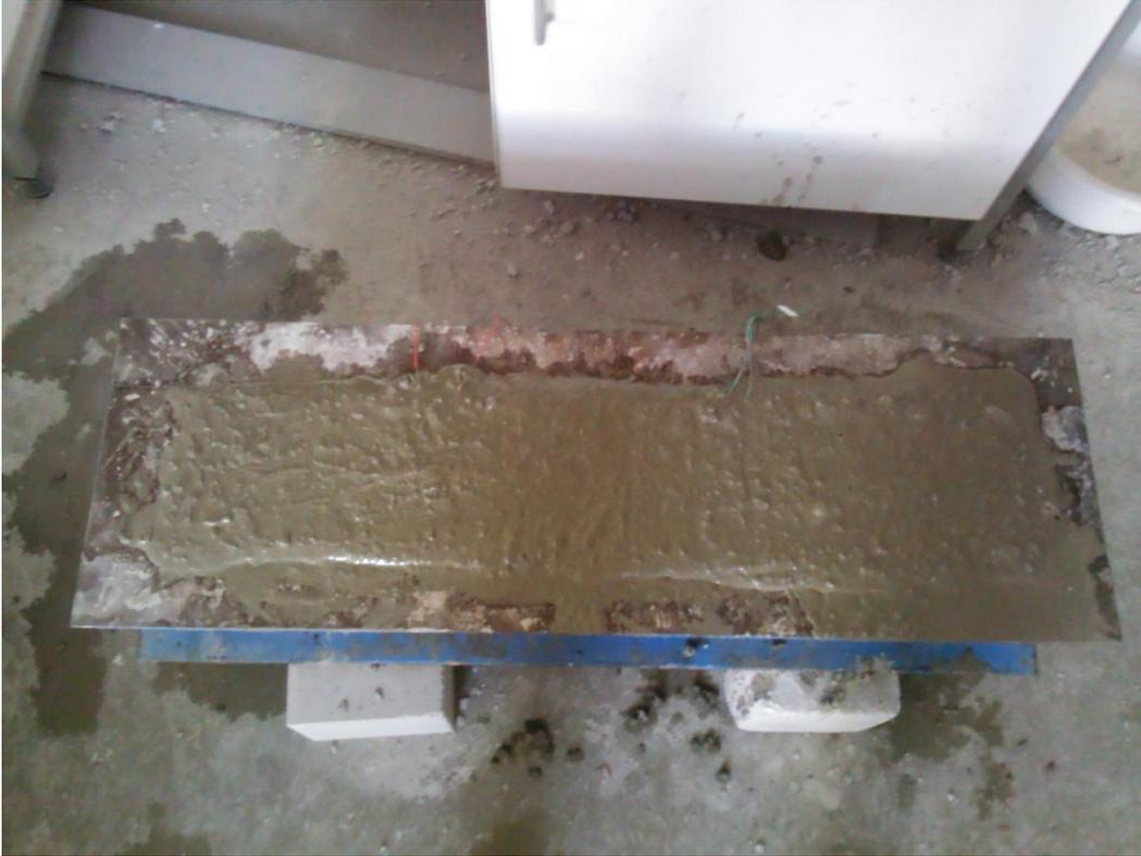
Picture 8.9 Final form of beam specimens
