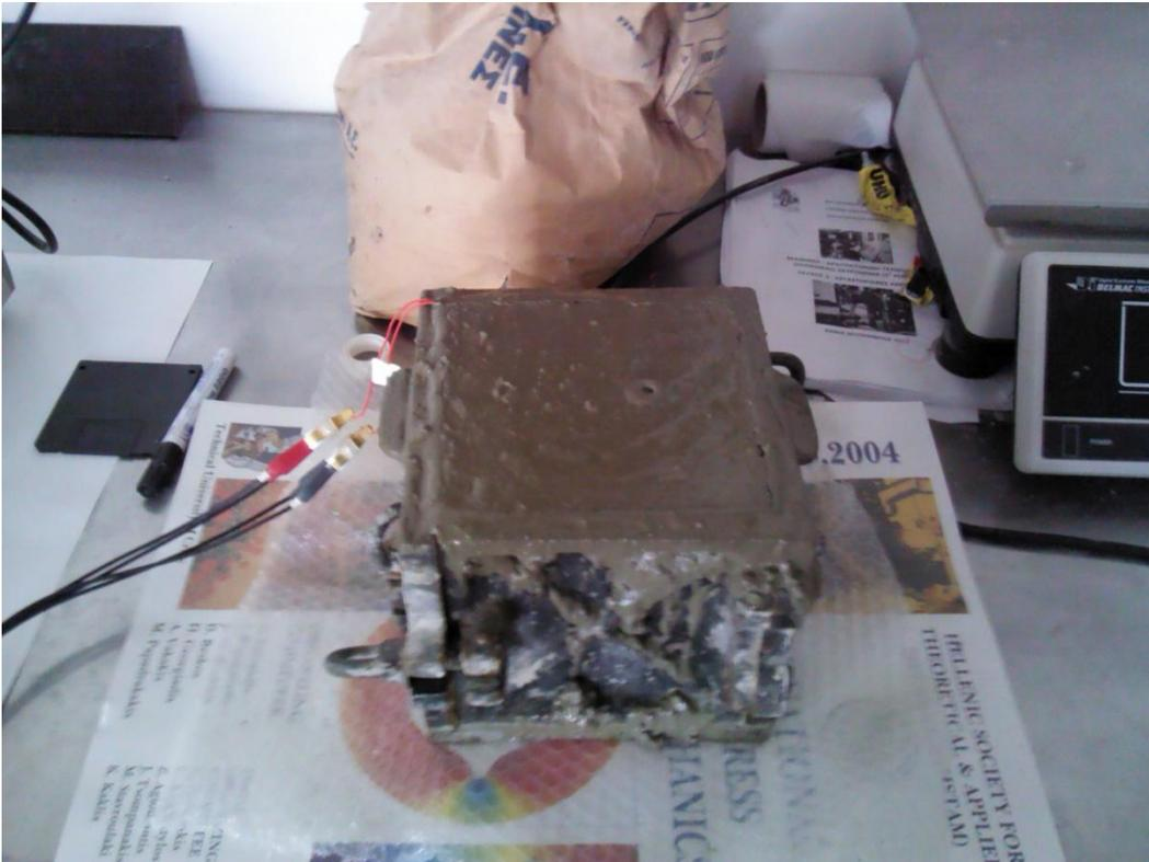
Picture 8.9 Final form of cubic specimens
