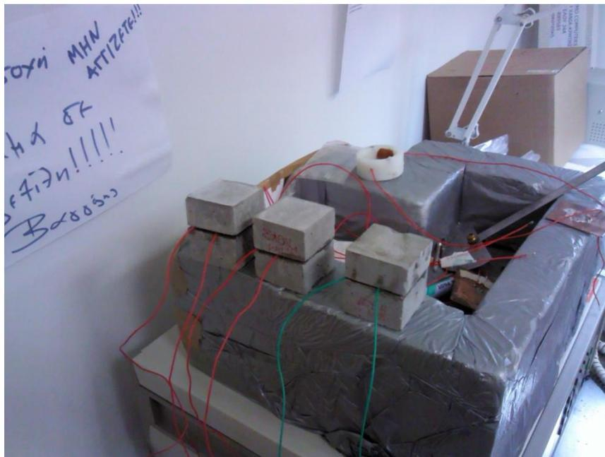
Picture 7.3 Final form of "smart" aggregates
