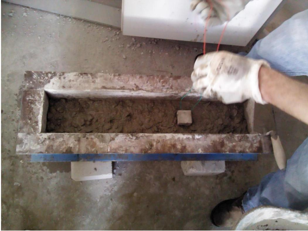
Picture 8.7 Creation of the beam specimen
