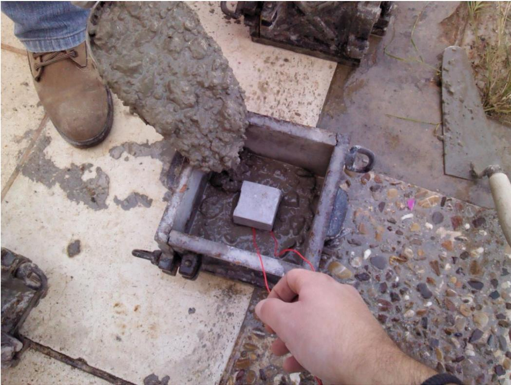
Picture 8.4 Smart aggregate inside the cubic specimen
