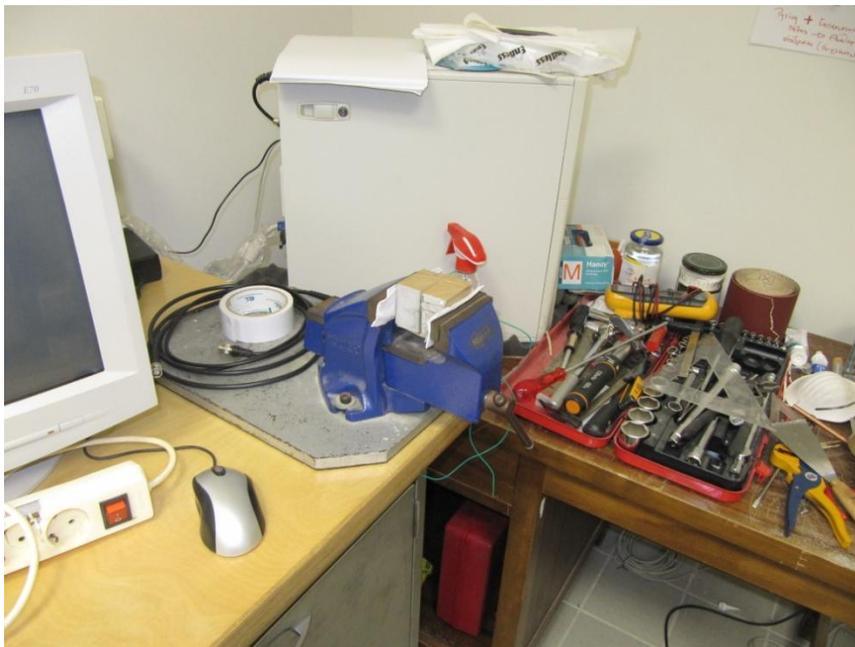
Picture 7.5 Manual compression of “smart” aggregates
