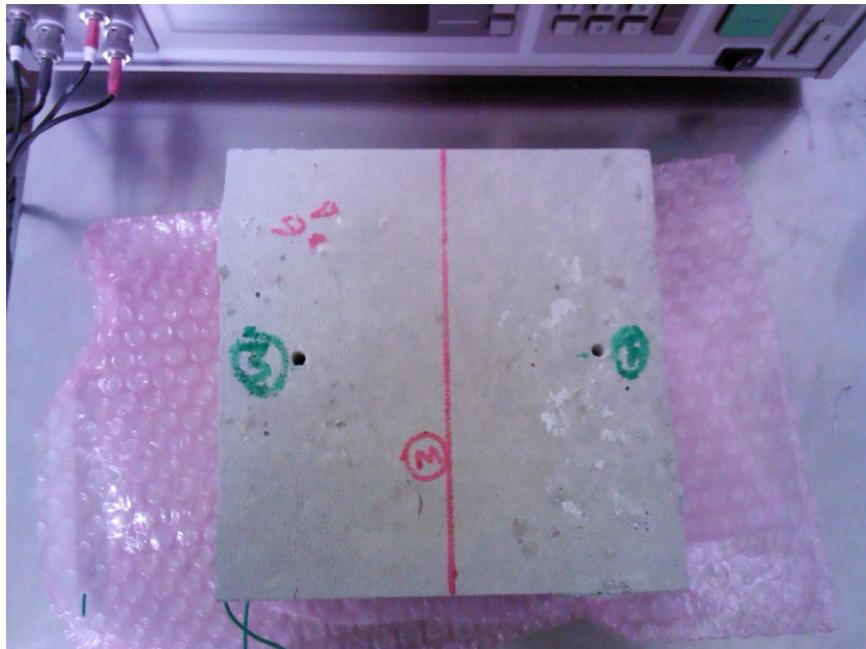
Picture 9.1 Damage holes 1,3
