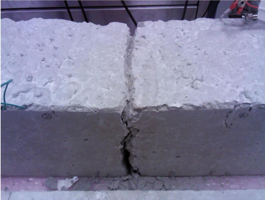
Picture 9.19 Damage 2-Detachment of the cement paste layer (failure)
