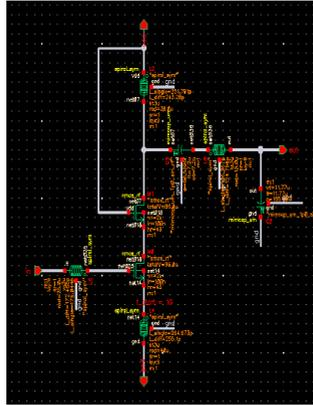
Figure 2.10: Schematic diagram of the LNA.
