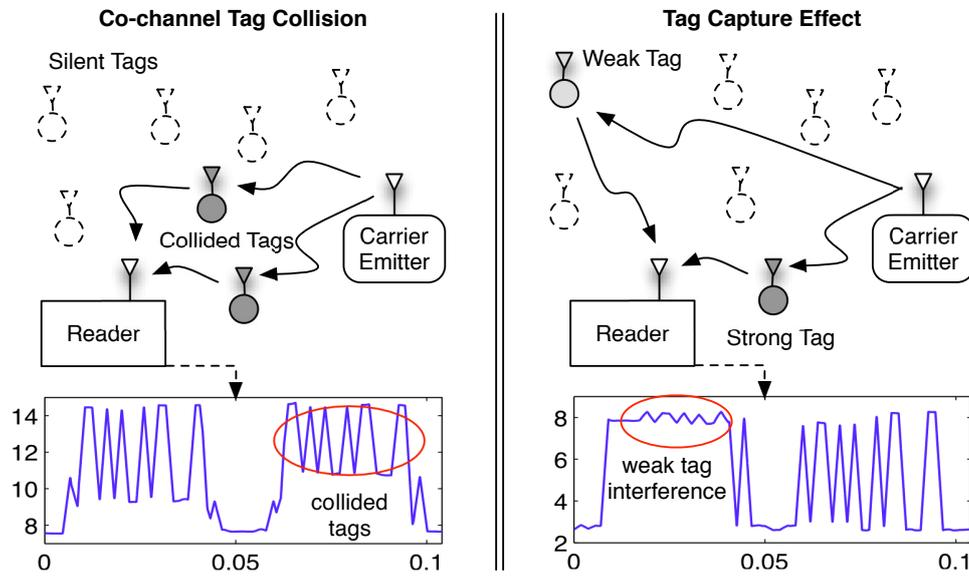
Figure 4.12: Capture effect experimentation. Left: Tags collide by transmitting at the same time. Right: Tags are re-programmed to examine capture effect (strong tag is decoded successfully, even at the presence of a weak interfering tag). The figure depicts real signals captured by the SDR receiver.
