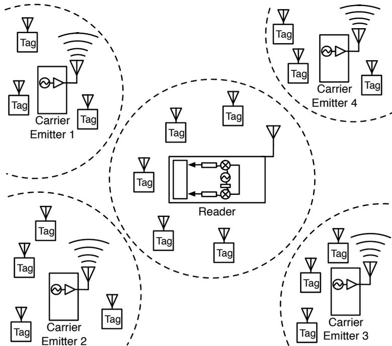
Figure 1.3: Proposed WSN architecture. Multiple, low-cost carrier emitters are placed in the field. Around them many ultra low-power tags are deployed.
