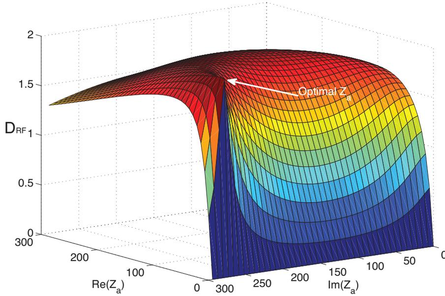
Figure 2.5: 3D plot of real and imaginary value of  $Z_a$  vs  $D_{RF}$  at 868 MHz. Observe that there exists an antenna with  $Z_a = 56.6 + 196.08i$  Ohm that sets  $D_{RF} = 1.916$ .
