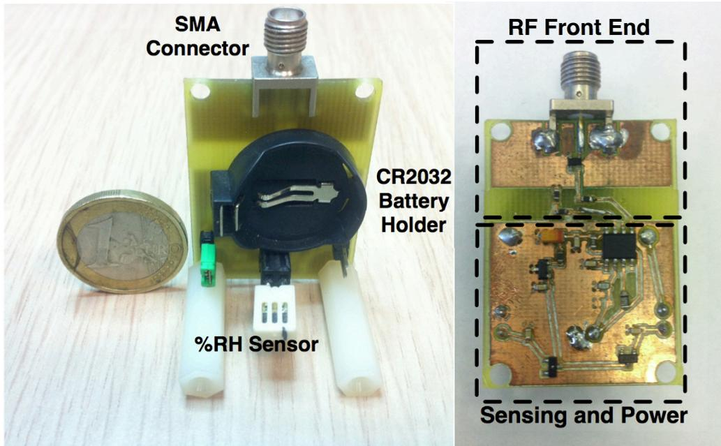
Figure 2.2: The developed prototype sensor tag. The sensing/power part are distinguishable from the RF front-end part.
