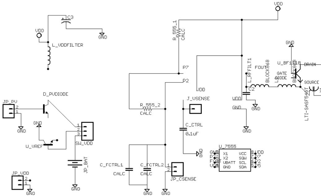
Figure 6.8: V3 schematic. Improved power supply with voltage reference, through-hole SMA (smaller cost), BF1118 utilization, no enhanced RF front-end
