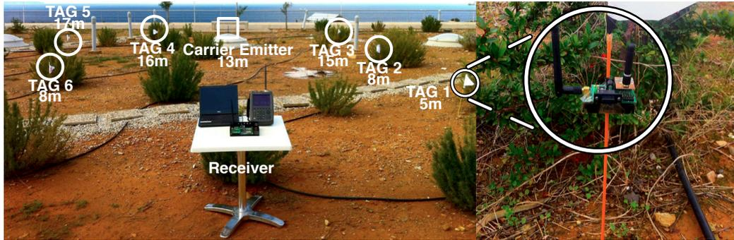
Figure 4.7: Remotely programmable testbed and hybrid node, outdoor deployment.
