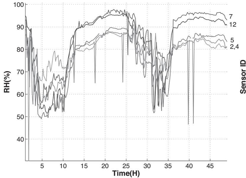
Figure 4.4: Data collected from multiple tags inside the tomato greenhouse for a total of 48 hours. Differences in %RH are due to the variability of microclimatic conditions across the greenhouse (e.g., tags closer to the window exhibit smaller %RH values).
