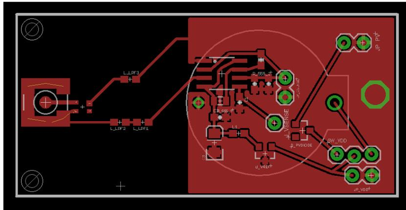
Figure 6.10: V4 layout. First effort for enhanced RF front-end with utilization of chokes. Schematic same as V3.
