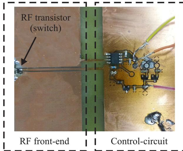
Figure 2.4: Tag with enhanced RF front-end.
