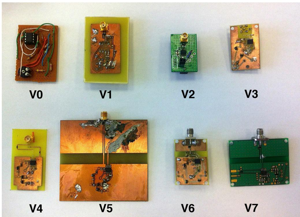
Figure 6.1: The major tag prototypes that were fabricated.
