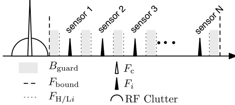
Figure 2.6: Scheme for networking multiple tags. Each tag operates in different frequency bands, while guard bands are set up in between to avoid collision.
