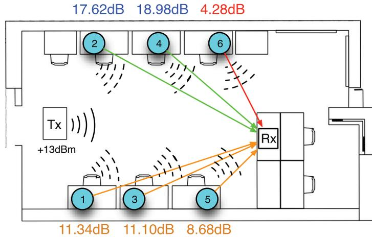
Figure 4.10: Measured SNR values per scatter radio tag in lab deployment.
