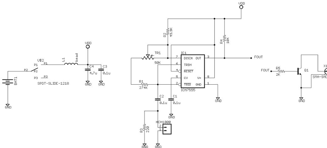
Figure 6.4: Schematic of the first working tag (V1). Utilization of 3V transistor (AT32033), no sophisticated power supply and RF front-end.
