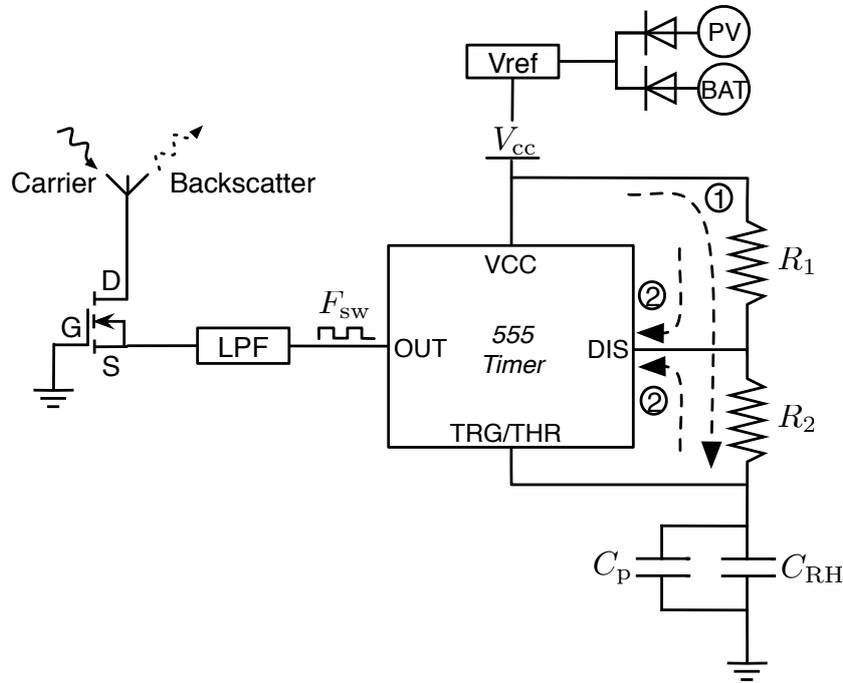
Figure 2.1: Sensor circuit diagram with scatter radio: capacitance varies the timer output frequency, producing a variable-frequency pulse that switches a single transistor; the latter is directly connected to the antenna [32,33].
