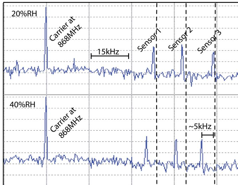
Figure 2.7: Scheme for networking multiple tags. Each tag operates in different frequency bands, while guard bands are set up in between to avoid collision.
