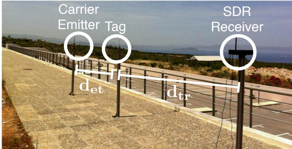
Figure 3.4: Bistatic setup in outdoor deployment for characterizing the communication range of a point to point link. Each device is set up in poles of 1.5 m height.
