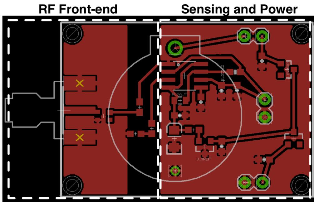
Figure 6.13: V6 layout. Improved for reduced stray capacitances. This is the tag layout that was used in the tomato greenhouse demo.
