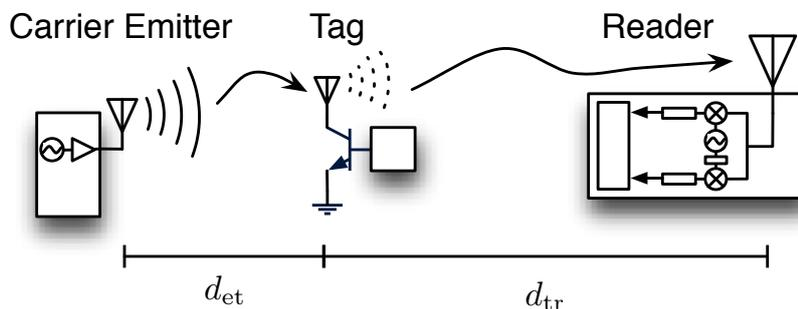
Figure 1.2: Bistatic scatter radio topology; carrier emitter placed in a different location from the reader.  $d_{et}$  and  $d_{tr}$  denote the emitter-to-tag and tag-to-reader distance, respectively.
