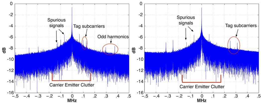
Figure 4.11: Left: tag operating inside RF clutter (BER 35%). Right tag operating away from RF clutter (BER 3.5%)
