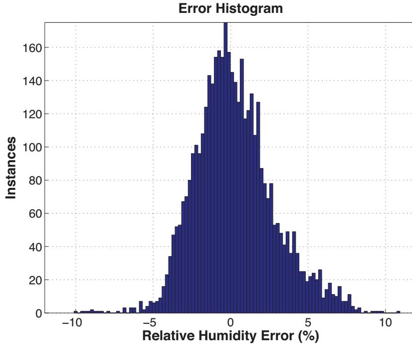
Figure 2.10: Measured %RH error histogram.
