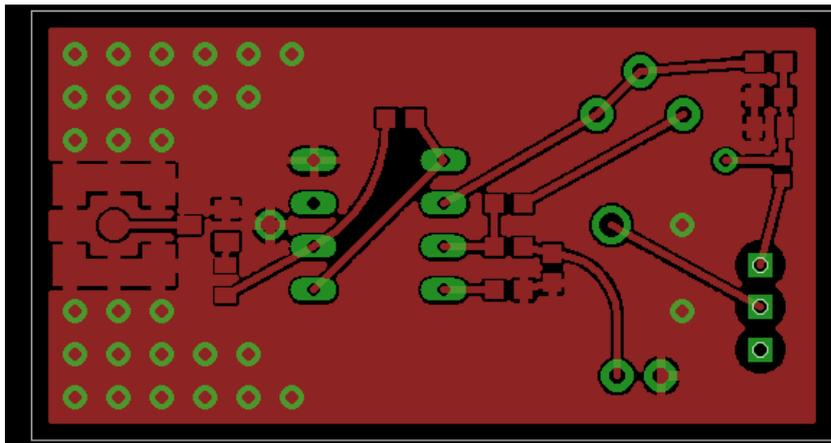
Figure 6.5: Layout of the first scatter radio tag prototype (V1).
