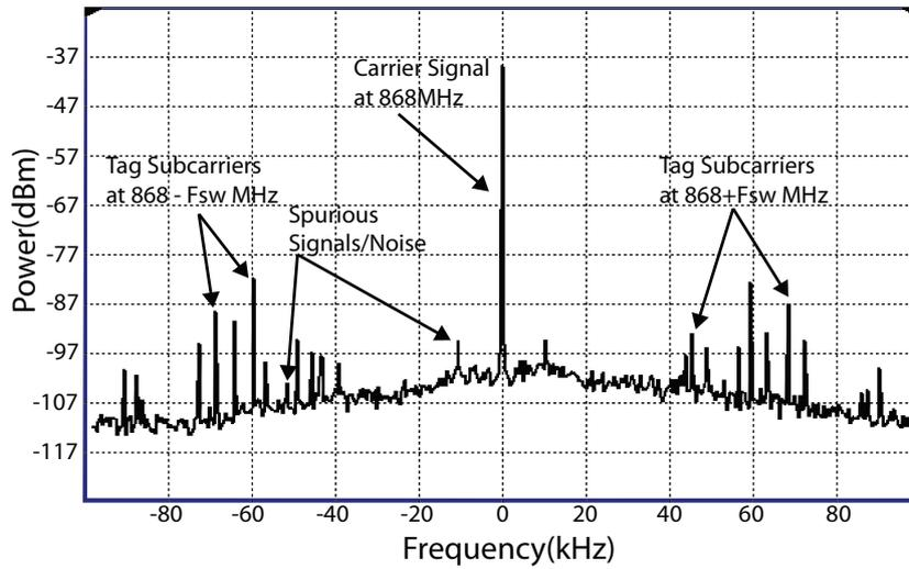
Figure 4.3: Periodogram from multiple sensors in the greenhouse. Each tag operates in a distinct frequency band.
