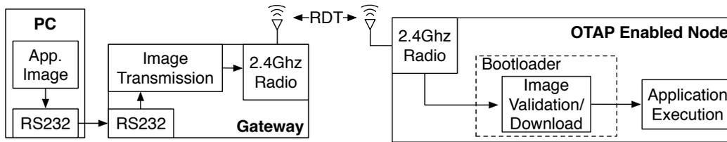
Figure 4.8: Over the air programming block diagram.
