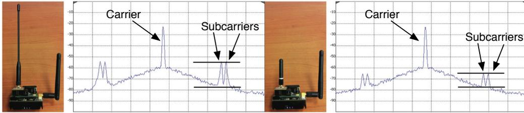
Figure 4.9: Received power spectrum of a half-wavelength and a quarter-wavelength antenna with fixed tag-reader distance. The switching (i.e sub-carrier) frequencies are clearly visible. The quarter-wavelength antenna scattered signal has fairly smaller amplitude than the one scattered from the half-wavelength antenna.
