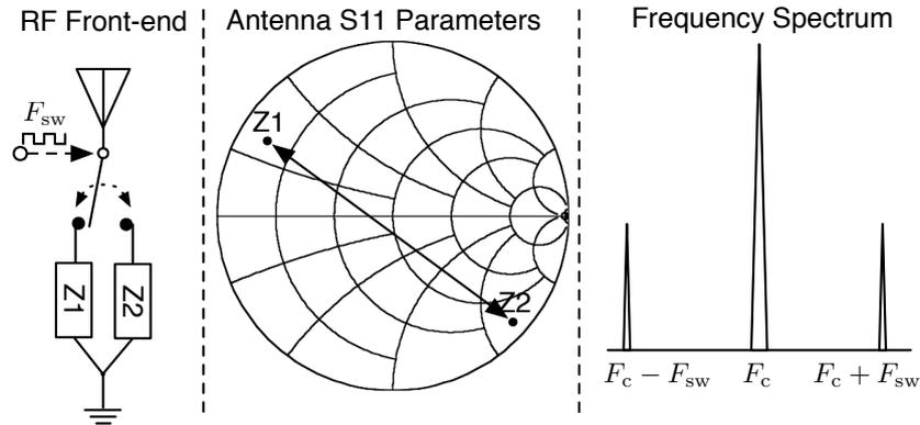
Figure 1.1: Scatter radio communication principles: RF switch alternates the loads of the tag antenna with frequency  $F_{sw}$ . When a carrier is imminent with frequency  $F_c$ , two subcarriers appear, with frequencies  $F_c \pm F_{sw}$ .
