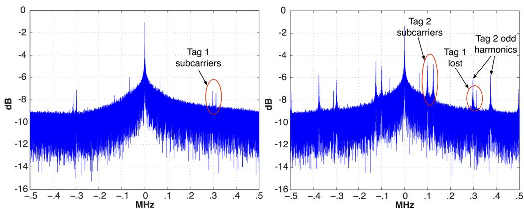
Figure 4.13: Left: Tag 1 operating without interferer with BER 3.5%. Right: Tag 1 operating with BER 35% due to interfering Tag 2 odd harmonics.
