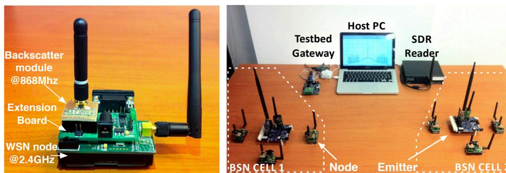
Figure 4.5: Left: Hybrid testbed node. Right: Experimentation testbed.
