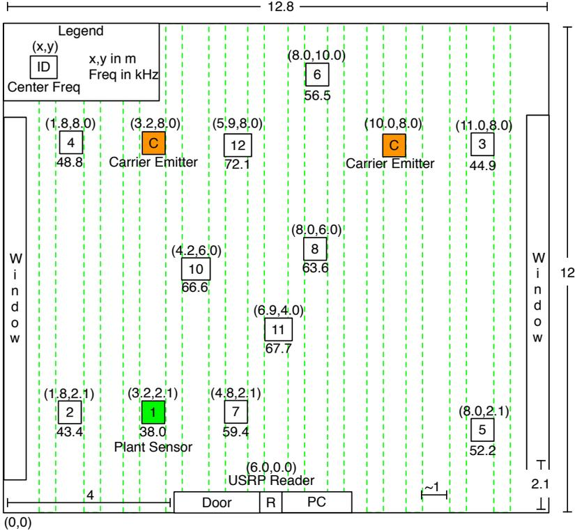
Figure 4.1: Experimental network topology. 10 %RH sensors, 1 plant voltage sensor and 2 carrier emitters with transmit power at 20 mW were deployed.
