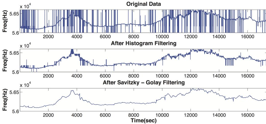
Figure 3.3: Filtering process of received measurements. Histogram filtering followed by Savitzky-Golay filtering is applied.
