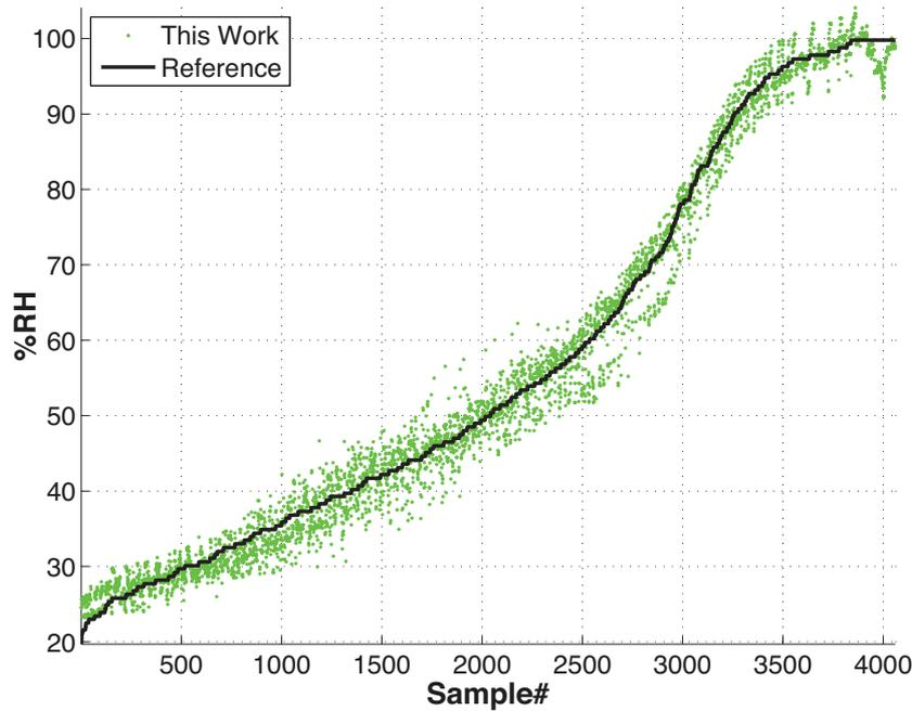
Figure 2.9: Reference vs received %RH measurements.
