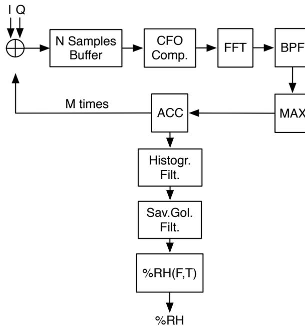
Figure 3.1: Sensor's subcarrier frequency value is estimated using periodogram detection. After a set of data is collected, the aforementioned filtering is applied.
