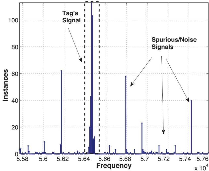
Figure 3.2: Histogram filtering: A set of measurements is collected and their histogram is calculated. Only measurements within a certain range and with the highest occurrence are kept.
