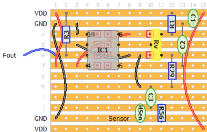
Figure 6.3: V0: Breadboard design of the prototype capacitance-to-frequency converter.
