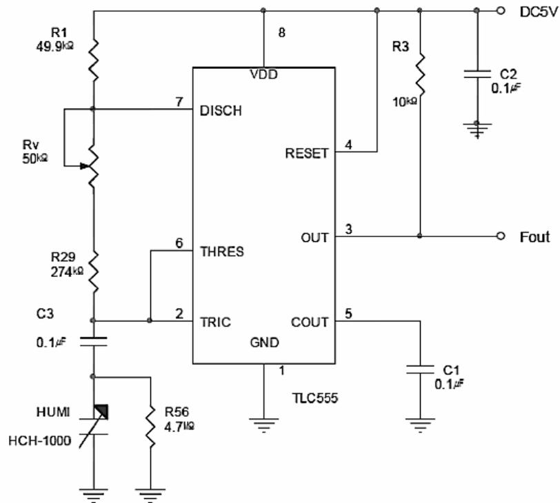
Figure 6.2: V0: Capacitance-to-frequency converter prototype.
