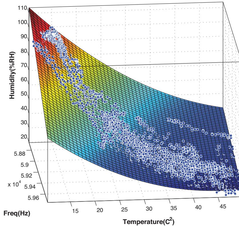
Figure 2.8: Temperature is included as a calibration parameter and thus the characteristic function is the surface  $RH(F,Temp)$ .
