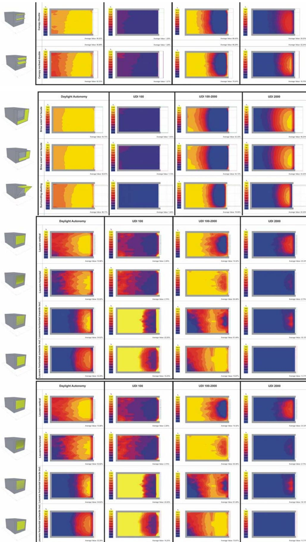
Figure 3: Comparison of UDI values in relation to DA values for all SDs examined for the case of Chania
