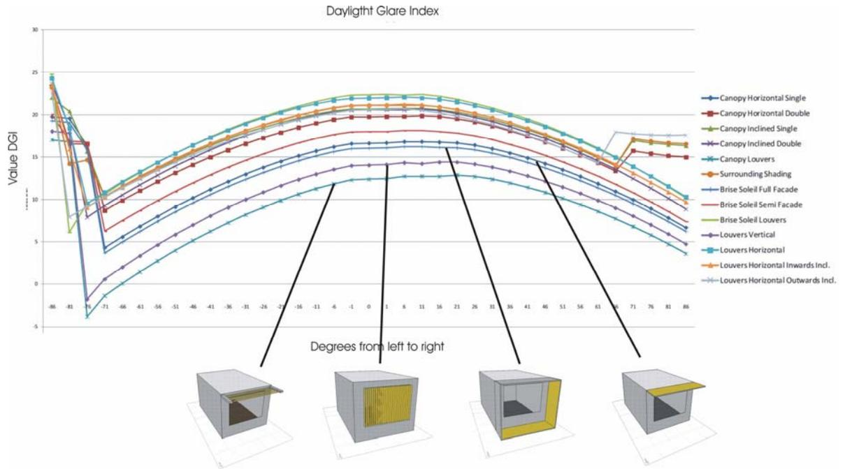
Figure 4: DGI values for the 21 December at 12:00 o'clock for all examined systems in relation to the angle of view for the camera away from window
